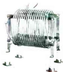
**ISOLATION INDUCTOR** . . . carries sampling line across base insulator without detuning tower. Wound of 3/8 inch coaxial cable. Diameter 12 inches. Length 15 inches. 70 microhenries.
