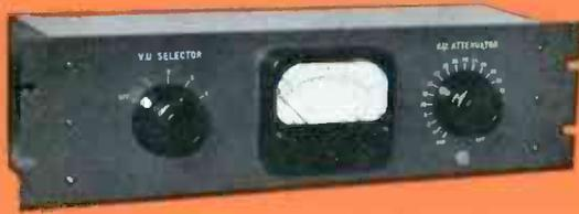
**62E-2 VU PANEL** . . . accurately monitors audio levels in broadcasting, recording studios, and sound systems. A Weston type 30 meter is provided, with illuminated face and easily read figures. Overswing is small, and pointer action is deliberate and positive. The 62E vu panels are designed to operate from a 600 ohm line. However, other impedances may be used in conjunction with a calibration chart.
