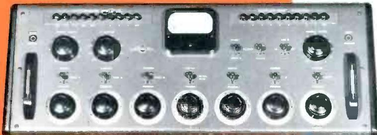
**212B AUDIO CONSOLE** . . . has the same features as the 212A-1 but is smaller, has fewer amplifiers and functional facilities.
