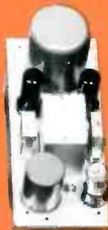
**6W-2 MONITOR AMPLIFIER** . . . is a 2 watt amplifier which may be used to drive monitor speakers, or for any other applications requiring up to 2 watts. An external power supply is needed.
