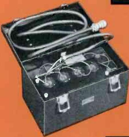
**412C BATTERY BOX** . . . is recommended for use with the 212Y and 212U Remote Amplifiers. The 412C-2 battery box is sturdily constructed, and holds the batteries securely. Space in the top of the case receives the 6 ft. rubber jacketed cable for transportation. Three thumb screws hold the clamp which secures all of the batteries in place.
