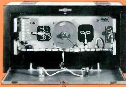
**414F-3 RELAY POWER SUPPLY** . . . well filtered, well regulated d-c power source for operating relays and pilot lights. An on-off switch and a pilot light are mounted on the front of the cabinet. A fuse receptacle is available through the access door.
