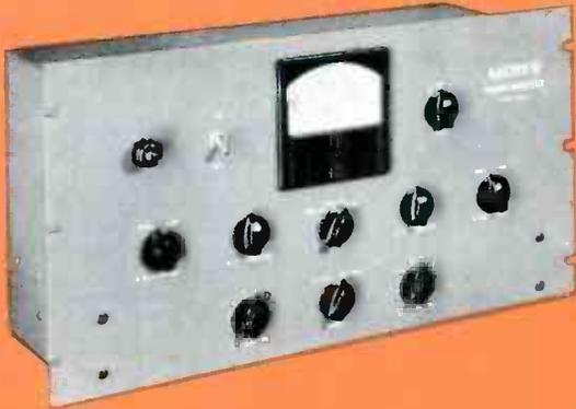
**ANDREW 40-C PHASE MONITOR** . . . facilitates adjustment and maintenance of broadcast directional antenna arrays. Phase Angles are indicated directly in degrees on a single meter, permitting immediate observation of the effects of small antenna system adjustments. Relative amplitude of antenna currents can be quickly determined with the ratio appearing on a special ratio scale.
