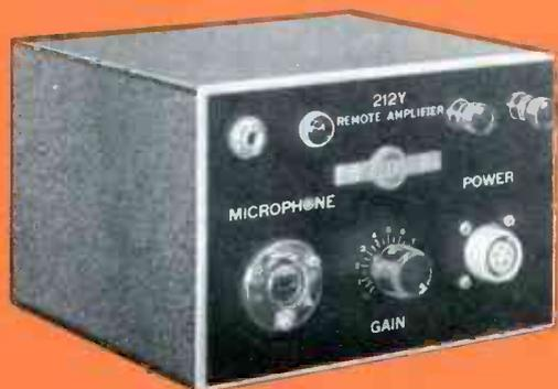
**212Y SINGLE CHANNEL REMOTE AMPLIFIER** . . . combines small size and light weight with high fidelity. One high fidelity channel is incorporated, which operates from a low level velocity, dynamic or other self-generating microphone. A universal input transformer matches all low impedance commercial type microphones.
