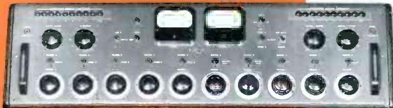
**212A-1 AUDIO CONSOLE** . . . provides facilities for auditioning or rehearsing, cueing and broadcasting simultaneously from any combination of two studios, an announce booth, a control room microphone, two turntables, and any two of nine remote lines. Two program amplifiers are included to feed two independent programs, or by operating the line reversal switch, providing an emergency amplifier for normal use.
