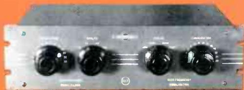
**116F-1 PROGRAM EQUALIZER** . . . provides complete facilities for controlling the frequency response of program and communication circuits. Since this unit has an insertion loss of 30 db, the Collins 6R Isolation Amplifier in association returns the level to normal, plus gain if desired.
