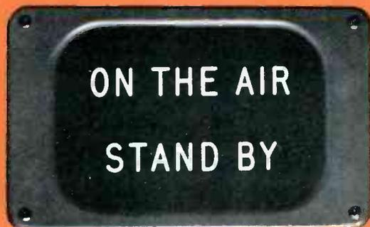
**209A WARNING LIGHT ASSEMBLIES** . . . are constructed of aluminum sheet metal with a divided light compartment. Each of the two light compartments contains two 7½ watt 110-volt a-c bulbs and sockets to provide illumination of the lettering.
