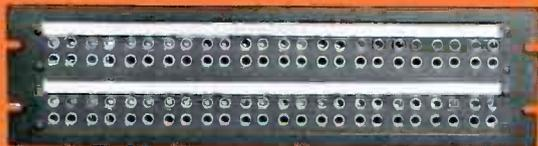
**TYPE 265D JACK PANELS** . . . provide connections for test purposes or for terminating program lines and order wires. Lines, amplifiers, microphones, equalizers, and other audio equipment can be speedily interchanged for maintenance or emergency operation. These jack panels mount in standard 19-inch racks. Regularly supplied with Collins 360 1010 00 jack.
