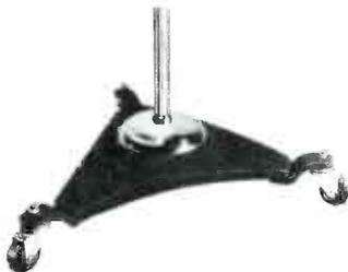
**DS-10 DESK STAND** . . . receives any microphone having ⅝" x 27 thread. Adequate space underside for installation of on-off or push-to-talk switch. Rubber bumpers protect desk surface. Constructed entirely of precision die castings. Finish is gunmetal opalescent enamel with chrome trim. Weight is 1½ pounds.
