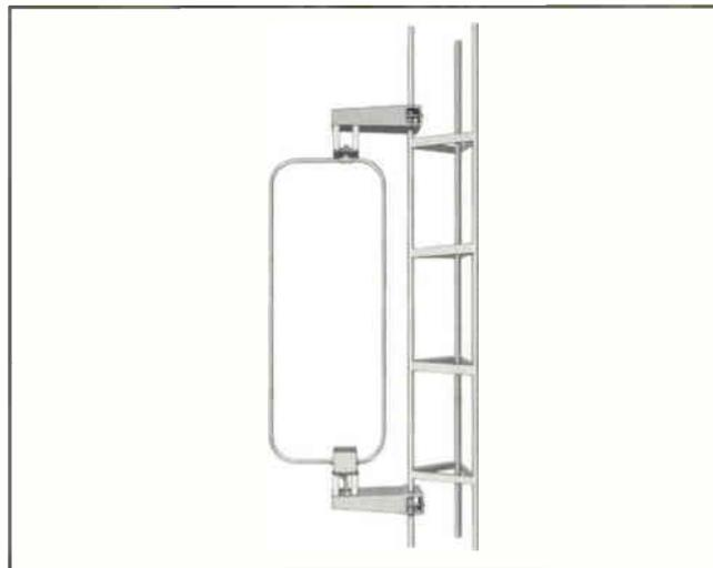
Designed to sample the relative phase relationship of radio frequency energy from 550-1600 kc antenna towers in directional antenna arrays, the Collins 564A-1 is made of two loops of #10 copper wire which may be connected either in series or in parallel. The wires are contained within a loop of 7/8" painted, copper tubing which serves as an electrostatic shield.
