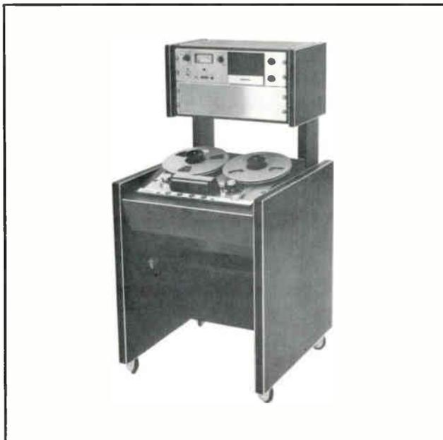
The ampex AG-350 series transport retains the time proven 350 series transport features. Outstanding features include automatic equalization, rigid top plate, direct drive capstan, accurate traction pressure through positive solenoid control of capstan idler which disengages automatically when power is shut off, take up arm to eliminate tape bounce, push button control panel, 10 $\frac{1}{2}$  inch reels, tape speed switch automatically switches equalization,
