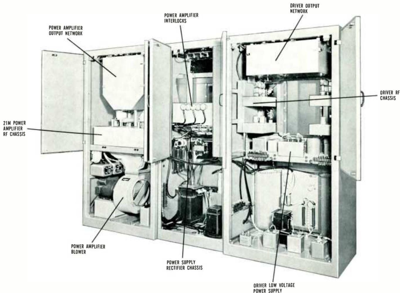
unit has separate power supplies for high voltage, low voltage and bias.
