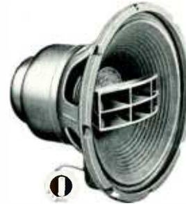
A coaxial, 12" speaker, the H-222 has electrically and acoustically independent "woofer" and "tweeter," and employs the through-bore compression driver tweeter. *Frequency Range:* 30-15,000 cps. *Impedance:* 16 ohms. *Power Rating:* 25 watts. *Baffle Opening:* 10 1/2". *Weight:* 12 lbs. Jensen transformer (ZY-2003) for H-222 speaker matches to 600 ohms.
