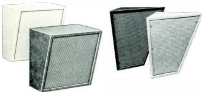
Entire front is inset with plastic grille and cloth covered panel. Constructed of plywood and hardboard for good resonant tone. Extra reinforcing blocks and four bolts installed for mounting speakers. Covering is plastic coated leatherette. Available in blonde or walnut. Slanting corner baffle for 8" speaker (SCB-8A) or 12" speaker (SCB-12A). *Weight:* 6 lbs. or 8 lbs. Wall baffle for 8" speaker (WB-8C) or 12" speaker (WB-12C). *Weight:* 2½ lbs. or 4¼ lbs.
