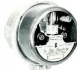
Designed to be mounted on either curved or flat surfaces, the 63305-C will automatically control broadcast tower, billboard or street lighting system directly or with auxiliary controllers. Operated by stable phototube with high sensitivity to north sky illumination, which is predictable and smooth in decline to darkness.
