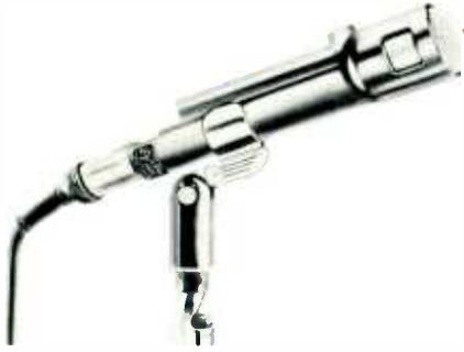
This microphone provides high discrimination against sounds from back hemisphere. Permits close talking with no bass accentuation and increases working distance over pressure microphones by factor of 1.7:1 due to polar pattern. Clamp-on stand mount with  $\frac{5}{8}$ "-27 thread,  $\frac{1}{2}$ " pipe thread adapter and 20' cable included.
