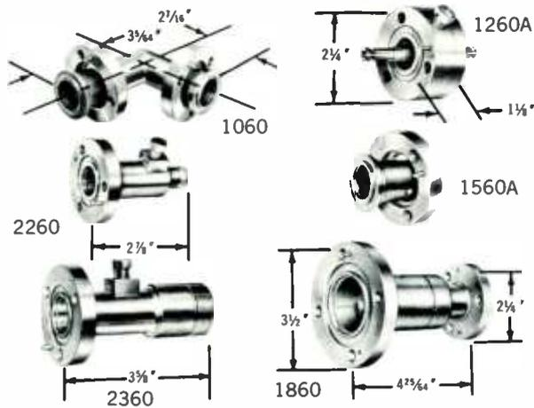
**REDUCER** — Connects Type 560 to Type 561 line. VSWR is less than 1.03 up to 1900 mc. Includes connectors and hardware for both ends (Type 1860).
