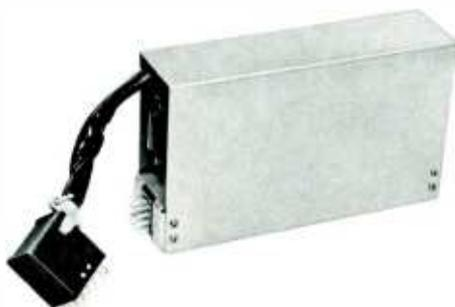
Used in Collins 212E-1 Console, this unit has four relays to control studio speakers and warning lights. Each relay is provided with a series shunt circuit to minimize switching transients and arcing. Noise is held to a minimum by mounting the relays on rubber. The 409X-2 Power Supply provides 12 v dc at 1 amp and studio wiring provides power for the warning lights.
