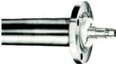
Constructed of high conductivity copper tube, the Prodelin 100-825 1 5/8" transmission line is manufactured in 20' lengths, flanged at both ends. Includes anchor insulator-connector assembly, "O" ring and hardware.
