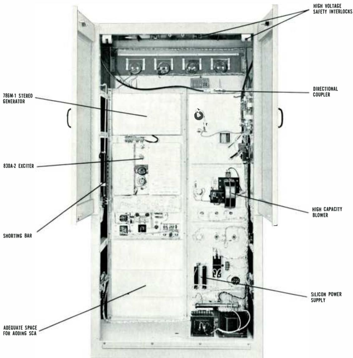
taking the transmitter off the air. Simplified controls make remote operation possible by addition of remote control units.
