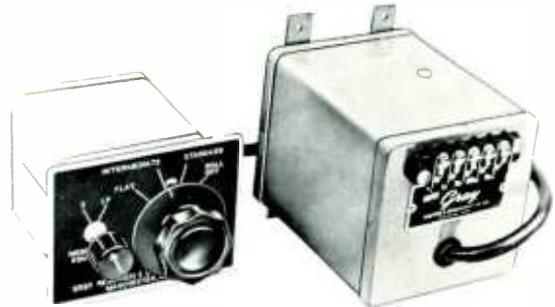
Normally used with standard microphone preamplifiers, making it unnecessary to purchase special audio input equipment when using magnetic cartridges. A convenient control permits instantaneous input switching from conventional records to microgroove. *Output Impedance:* 250 ohms balanced (150 or 50 ohms available). *Insertion Loss:* 20 db. *Output Level:* -67 VU at 4.7 cm/second. *Cable Length:* 18".
