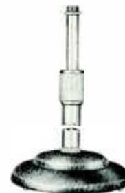
A general purpose, chrome plated adjustable desk stand with base of cast iron and finished in gun metal shrivel finish. Stable base is equipped with pads to prevent damage to desk. Equipped with standard "velvet action" clutch adjustment. Thread size at microphone end is  $\frac{5}{8}$ "-27. Adjustable from 8" to 12". *Weight:* 3 lbs.
