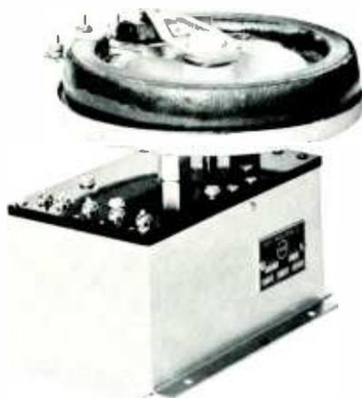
**MOTORIZED PLATE RHEOSTAT** — For 250-1,000-watt transmitters. Standard 750 ohms, 500 watts, 3,000 v insulation (Type 108-21B).
