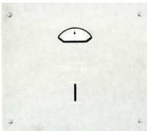
Gives direct indications of magnitude and direction of frequency deviation of AM transmitter. Positive indication is provided for failure of either transmitter carrier or monitor crystal oscillator. *Frequency Range:* 0.5-1.6 mc (specify crystal frequency). *Deviation Range:*  $\pm 30$  cps. *Primary Power:* 105-125 or 210-250 v, 50/60 cps, 125 watts. *Size:* 19" W, 15 $\frac{3}{4}$ " H, 13" D. *Weight:* 51 lbs.
