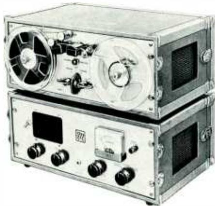
The PT6-6A Recorder and PT6-6J Amplifier are designed for either rack mounting or portable use. Powered by two-speed hysteresis synchronous motor for 7½ and 15 ips, selectable by switch. Low impedance and high impedance inputs are provided as well as 4, 8, 16 and 500 ohm outputs. The unit includes full-track erase and record/playback heads (half-track heads may be specified at no additional cost).
