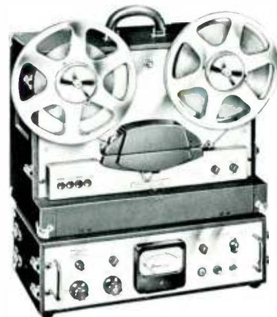
A portable recorder-amplifier combination, the M-90AC has a two-speed (7 $\frac{1}{2}$  and 15 ips) direct tape drive with outboard capstan bearing assuring low flutter. Integrated design, torque motor supply and take-up tension achieve timing accuracy of better than 3 seconds in 30 minutes. Available without carrying case (M-90ACX) for rack mounting and in monoaural or stereo models. Also available on special order are remote control (M-90R) and console cabinet.
