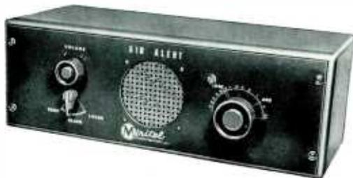
Designed to control visible and/or audible alarm circuits on CONELRAD signal from local or sky wave stations. Frequency tunable from 550 to 1600 kc. Built-in speaker operates upon alarm. Relay circuit is voltage regulated. External bell or light control terminals and antenna terminals on rear terminal board. Available for rack or table mounting.
