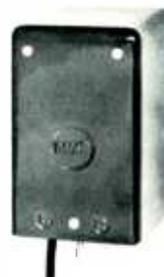
**ROTARY ACTUATOR** — Uses 2 rpm reversible motor replacing control knob. Contains momentary switch and needs no relays. Torque adjustable up to 27 pound inches. Standard shaft ½". Requires 115 v, 60 cps (Type 108-10A).
