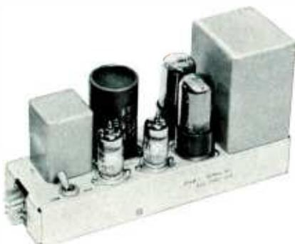
Used as the program line amplifier and monitor amplifier in Collins Consoles, the 356B-1 is a three stage amplifier with push-pull output and has a switch for high or low gain.
