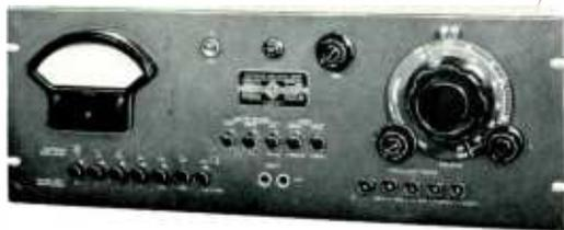
Measures distortion, noise and hum level in audio frequency circuits. In conjunction with the 1931-B Modulation Monitor, the 1932-A can be used to measure these quantities directly in the output of the transmitters.
