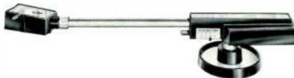
Accepts stereo and monophonic cartridges. Arm features precision ball bearings at all pivot points, plug-in head with positive alignment lock and variable adjustment. Supplied with arm rest, mounting template, mounting hardware and 4-foot cable assembly. *Size and Weight:* 12" arm (M232),  $12\frac{1}{8}$ " L, 1 lb.; 16" arm (M236),  $14\frac{1}{2}$ " L,  $1\frac{1}{8}$  lbs.
