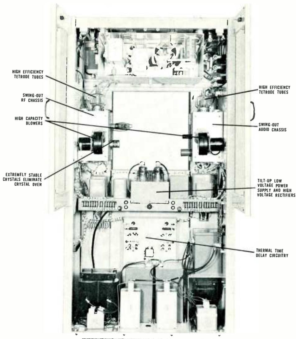
the air after a power line failure. After an instantaneous power interruption the carrier can be returned to the air immediately, cutting off-the-air time to a minimum. Overload relays are adjustable and are provided for the RF driver, audio driver, power amplifier and modulator stages. These relays are connected so that an overload removes plate power and the equipment must be re-energized manually.
