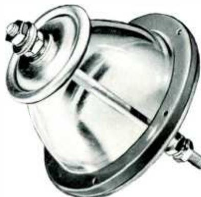
Designed to carry RF transmission line through a wall. Complete assembly includes heavy electrical glass feed-thru bowls, cork gasket and steel mounting flange with six 3/16" mounting holes. Bowl is 6-5/16" maximum diameter and 4 3/8" high. Mounting flange has 7 3/8" diameter. Fittings include spun aluminum corona shield, 1/2"-13 threaded stud (except 135-15-4 which has 5/8"-18 threaded stud, hollow), washers and nuts.
