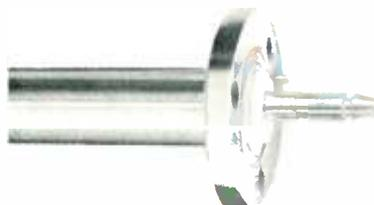
Constructed of high conductivity copper tube, the Prodelin 100-815 7/8" transmission line is manufactured in 20' lengths, flanged at both ends. Includes anchor insulator-connector assembly, "O" ring and hardware.
