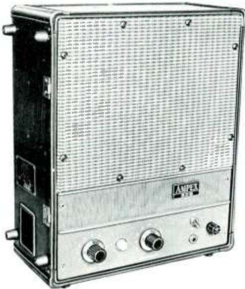
An ideal companion unit designed to match the Ampex 601 Series Recorder, the 620 has an 8-inch speaker that utilizes a high degree of bass and treble boost without undue harmonic or intermodulation distortion. The 10-watt power amplifier is of push-pull design. It is conventional high fidelity type but is unusual for its fast transient overload recovery.
