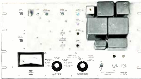
An optional feature of the Collins 830A-2 10-watt FM exciter, the Collins Stereo Multiplex Generator provides an audio modulation signal that meets all the requirements of the FCC-approved system.
