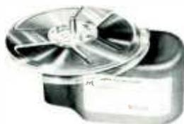
A bulk tape demagnetizer that develops a high intensity magnetic field to erase signals and noise without rewinding. Spindle mounting of reel permits rapid and thorough coverage. *Reel Size Range:* 5", 7", 10½" (spindle removable for use with other size reels). *Adapter Hub:* Available for use with 10½" reels. *Rating:* 117 v ac, 5 amps. *Size:* 5" W, 3" H, 8" D.
