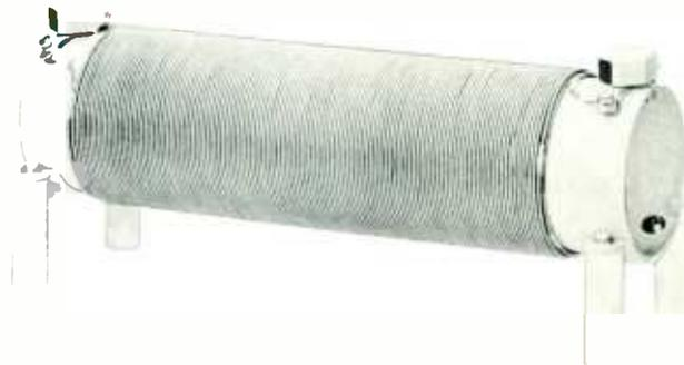
These solenoid wound 2- and 3-wire chokes provide high impedance throughout the broadcast band for isolation of the ac power lines from the antenna. Coils are wound of #10 wire and are rated at 2,000 watts, 120 v ac, single phase. Provided with mounting brackets and standoff insulators for mounting in 42E-7/8 antenna coupling units. Weatherproof cabinets are available for outdoor mounting.
