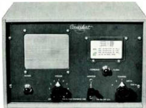
Designed expressly for CONELRAD Radio Alert. Built for 24-hour service, it gives automatic alarm with visual and aural warning. At time of radio alert, the speaker is automatically connected, you hear CONELRAD message and red pilot lamp on panel is lighted. Provision is also made for external alarm. Available in either cabinet or rack mounting models.
