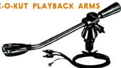
Tubular arm body with die cast aluminum cartridge shell and counterweight. Four-conductor lead accommodates all 3- and 4-wire stereo cartridges. Does not include but uses all standard cartridges. Available for either 16" (S-260) or 12" (S-320) recordings.
