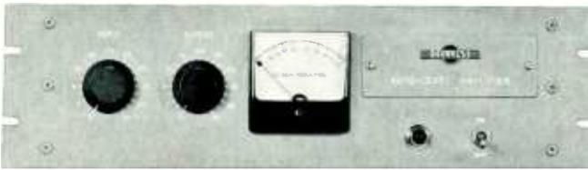
The average program level of the radio broadcast station can be automatically and effectively raised with the Collins 26J-1 Auto-Level Limiting Amplifier. The resulting effect of the 26J-1 is similar to turning up the volume of the radio receiver so that the low level transmission is as well received as the high level transmission.
