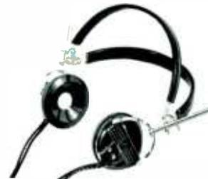
The Brush BA-206 headphones have an exceptionally flat response out to 10,000 cps and create outstanding fidelity of reception. Their high impedance and negligible power requirements allow monitoring without any effects on associated equipment. The special "Metalseal" crystal elements provide maximum protection against excessive humidity.
