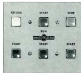
Three Collins automatic programming playback units, in addition to a record/playback system, may be operated with this control panel from a remote point in the broadcast studio. Buttons illuminate when in operation. *Size:* 5 $\frac{1}{8}$ " W, 2 $\frac{3}{4}$ " H, 4 $\frac{1}{2}$ " D.
