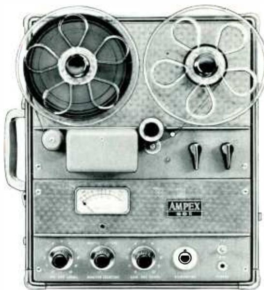
A lightweight and convenient portable recorder that is ideal in a variety of broadcast situations, the Ampex 601 has synchronous motor drive with a timing accuracy within 3.6 seconds during 30 minutes playback. Record and playback amplifiers are separate units.
