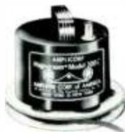
A compact and convenient bulk tape eraser that removes recorded signals from tape up to 35 mm in size and lowers background noise level up to 6 db below that of unused tape. A pushbutton safety switch prevents current from being applied when not in use. *Operating Voltage:* 100-130 v, 50-60 cps. *Size:* 2" H, 4" diameter. *Weight:* 2½ lbs.
