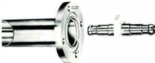
A very low VSWR line that is field proven for transmitter room interconnections, the Andrew 561 1 5/8" Teflon insulated line has compensated inner conductors. Anchor insulator connectors at each flange support the inner conductor on vertical runs and provide for differential expansion. Conductors and con-
