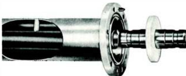
A Teflon insulated line, the Andrew 562A 3 1/8" is a versatile low VSWR line fully compatible with EIA standards. Inner conductor connectors use an Andrew designed piston ring spring to insure uniform and positive contact. The line is supplied in 20' sections. Special lengths are available by specifying Type 2762A and length in inches. Each section includes inner connector, "O" ring gasket, nuts, bolts and lockwashers. Where weight is important, aluminum construction is available.
