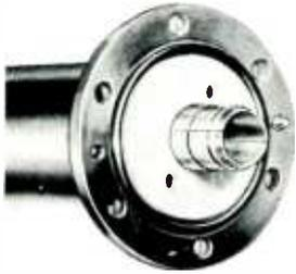
Constructed of high conductivity copper tube, the Prodelin 100-835 3 1/8" transmission line is manufactured in 20' lengths, flanged at both ends. Includes anchor insulator connector assembly, "O" ring and hardware.
