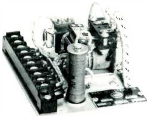
**DUAL MOMENTARY RELAY** — Adapts system to control start-stop pushbutton station or other operation requiring two SPDT relays rated 10 amperes ac (Type 108-18).
