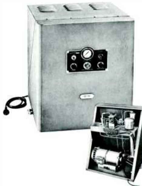
A piston type compressor unit that provides dry air for pressurization of air dielectric coaxial transmission line, the 1910A uses carbon rings to assure oil-free dry air and years of maintenance-free service. The compressor unit is driven by a heavy duty 1/4 hp motor.
