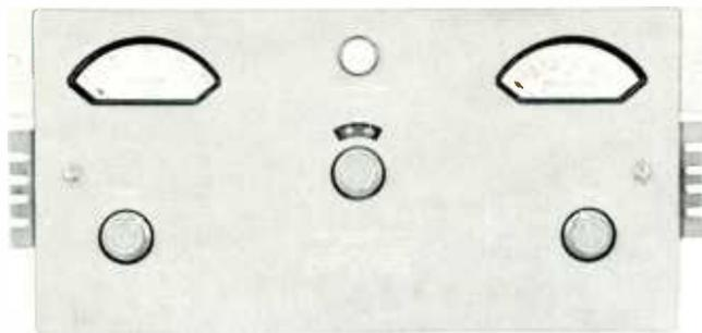
Measures percentage modulation on positive or negative peaks, indicates overmodulation, monitors program level and measures transmitter audio frequency response and carrier shift when modulation is applied. Operates in either 0.5-8 mc range or 3-60 mc range, depending on input coil used. *Primary Power:* 105-125 v, 50/60 cps, 50 watts. *Size:* 19" W, 8 $\frac{3}{4}$ " H, 10" D. *Weight:* 32 lbs.
