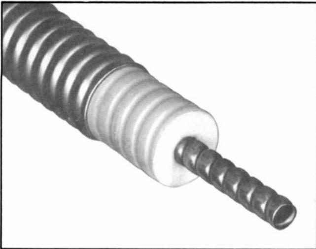
Type FH8 is the largest size foam dielectric Heli-ax available. The use of corrugated copper inner and outer conductors guarantees a flexible cable with extremely low attenuation for long runs or high efficiency systems.
