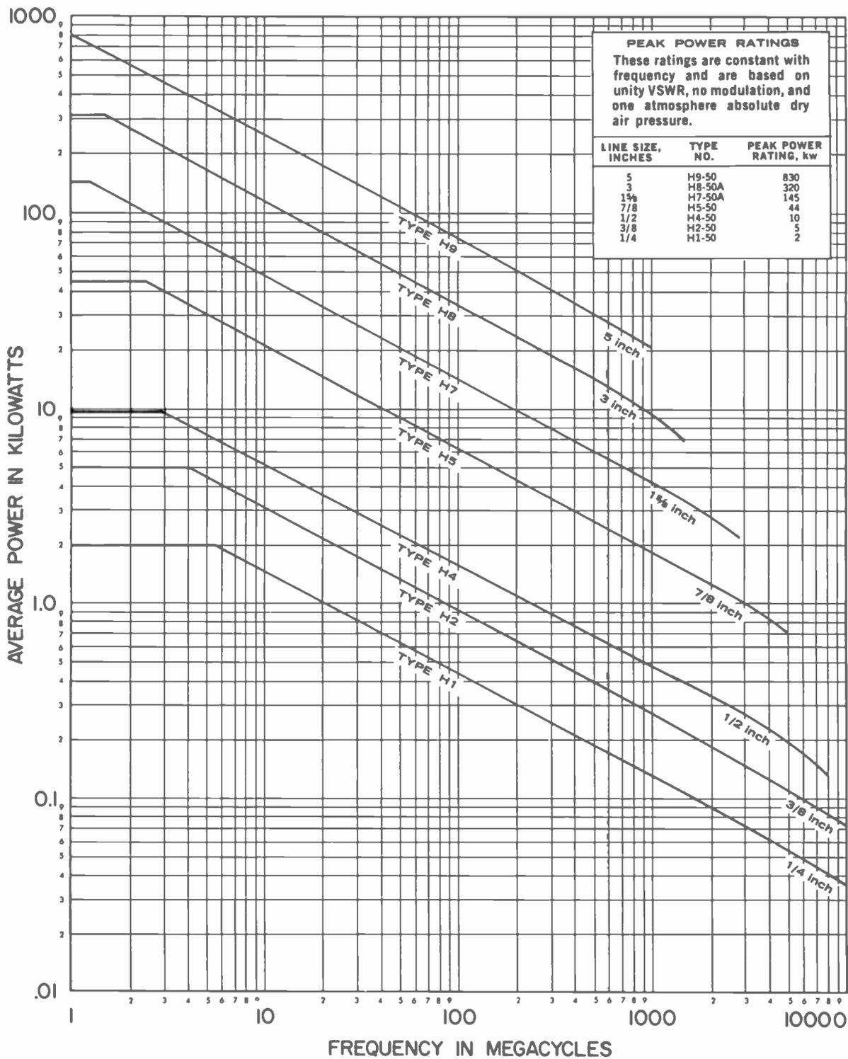
The average power ratings shown above are for 50 ohm copper Heliax and are based on unity VSWR and a maximum inner conductor temperature of 212°F at an ambient temperature of 104°F. For 75 ohm copper cables the values shown should be reduced 30%. For 50 ohm aluminum (outer conductor) cables the values should be reduced 10%. For Teflon insulated cables, average power ratings should be increased by 35%.
