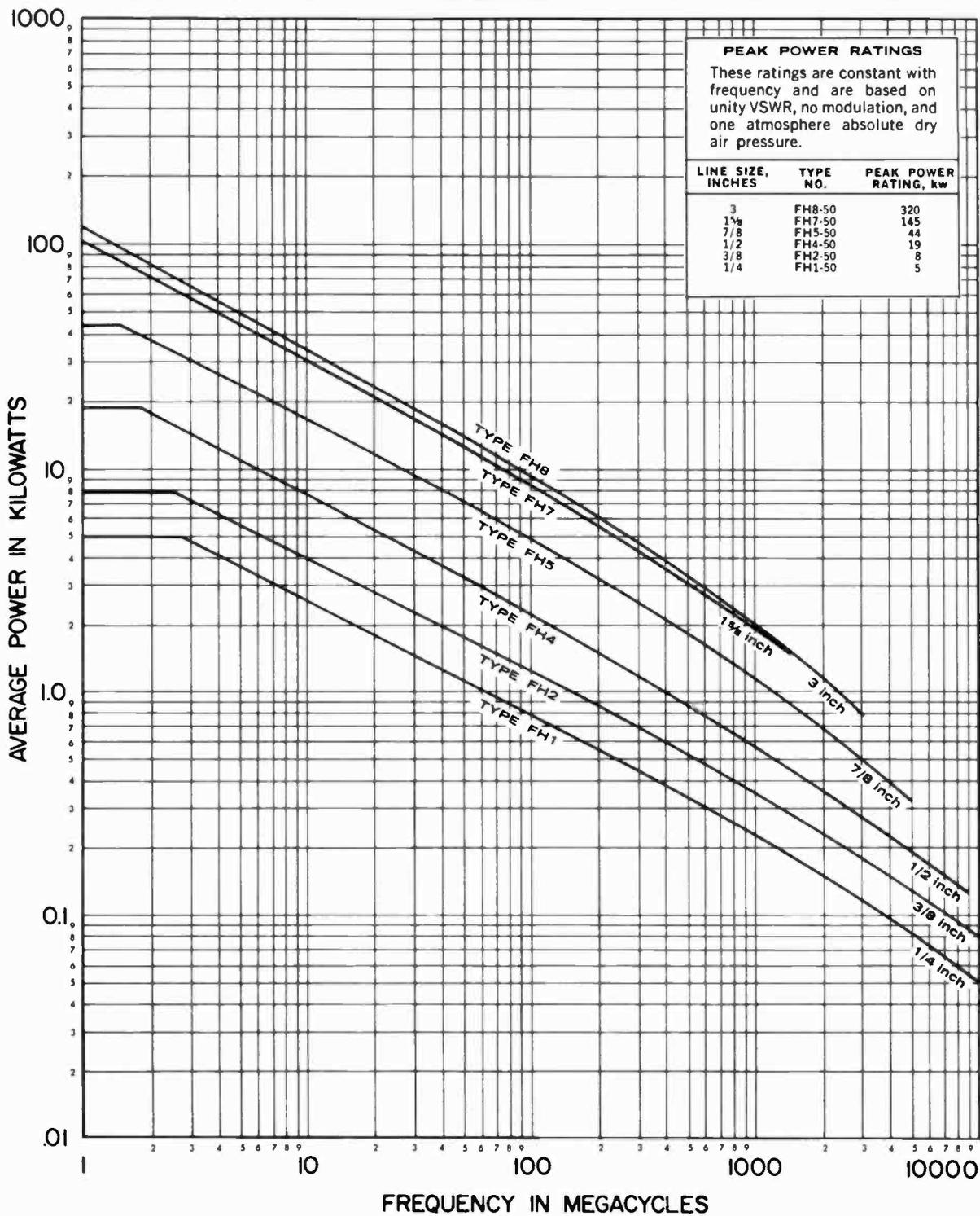
The average power ratings shown above are for 50 ohm copper Heliax and are based on unity VSWR and a maximum inner conductor temperature of 175°F at an ambient temperature of 104°F. For 75 ohm copper cables the values shown should be reduced 30%. For 50 ohm aluminum (outer conductor) cables the values should be reduced 10%.
