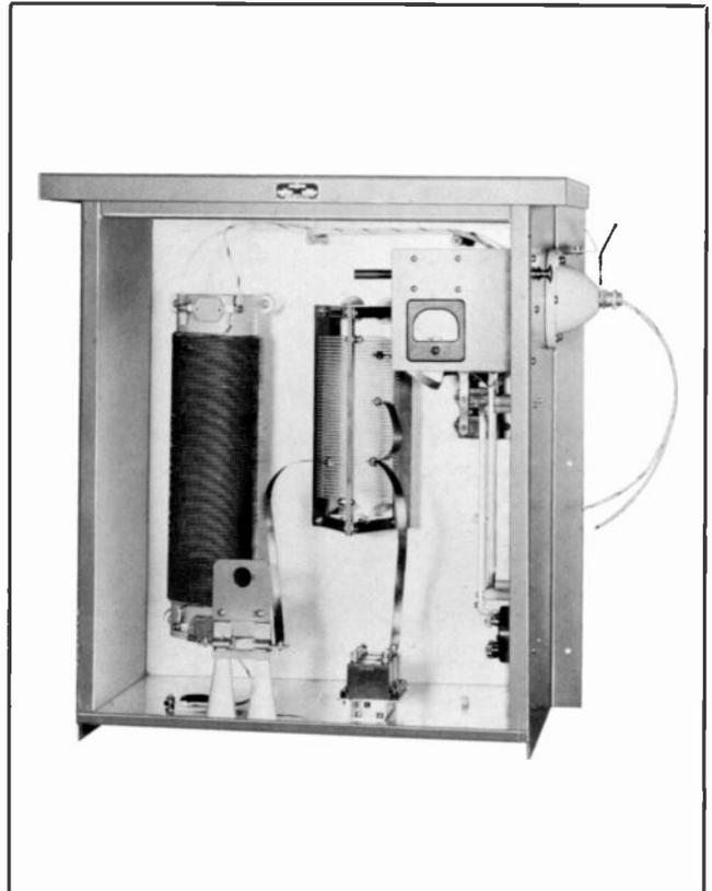
These specially constructed units match a series-fed vertical radiator to an unbalanced transmission line. Intended for continuous, unattended duty in conjunction with transmitters having emission type A0, A1, A2 or A3, the 42E-7 operates with transmitters of carrier power output of 250-1,000 watts. The 42E-8A operates with transmitters of 5,000 watts and the 42E-8B operates with transmitters of 10,000 watts.
