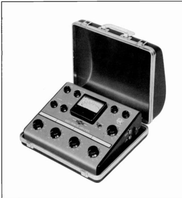
Weighing a total of 22 pounds including batteries and carrying case, the 212Z-1 offers full functions for remote broadcasts. This transistorized remote amplifier mixes inputs from up to four microphones, with program line and communication line outputs as well as an auxiliary output for PA feed.
