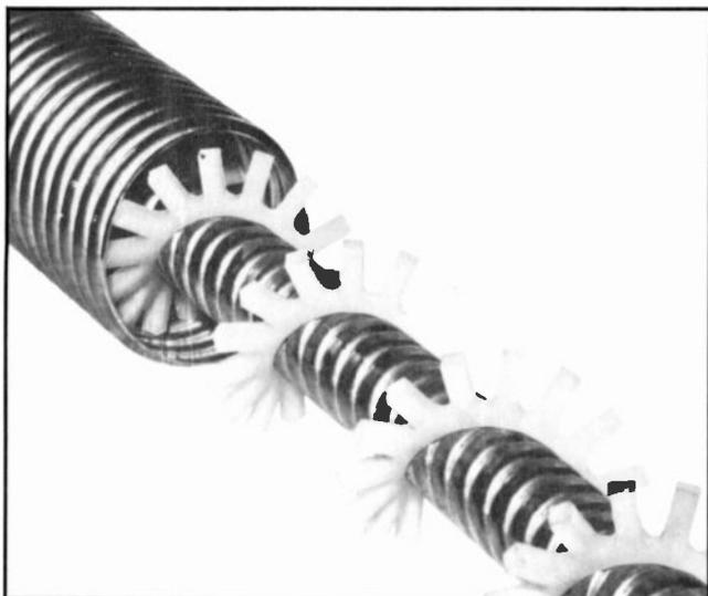
Type H9 HeliAx is designed for very high power, low attenuation service and is the largest available flexible coaxial cable. From VLF, LF and HF up through UHF-TV it is being used to replace many 6 $\frac{1}{8}$ " rigid transmission line installations.
