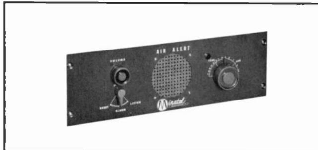
Designed to control visible and/or audible alarm circuits on EBS signal from local or sky wave stations. Frequently tunable from 550 to 1600 kc. Built-in speaker operates upon alarm. Relay circuit is voltage regulated. External bell or light control terminals and antenna terminals on rear terminal board. Available for rack mounting only.
