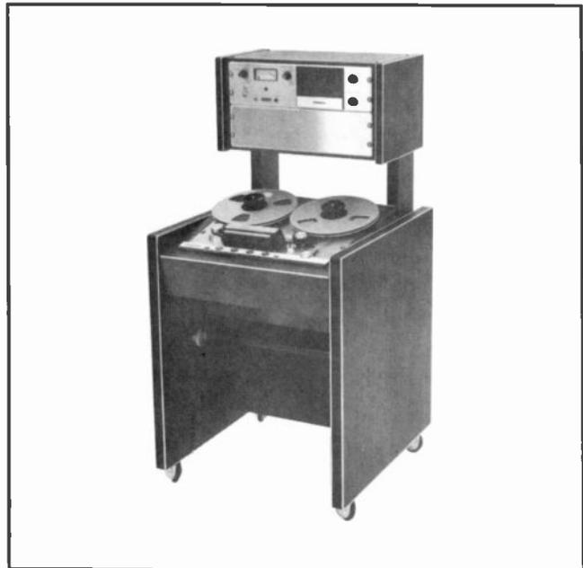
The ampex AG-350 series transport retains the time proven 350 series transport features. Outstanding features include automatic equalization, rigid top plate, direct drive capstan, accurate traction pressure through positive solenoid control of capstan idler which disengages automatically when power is shut off, take up arm to eliminate tape bounce, push button control panel, 10 1/2 inch reels, tape speed switch automatically switches equalization,
