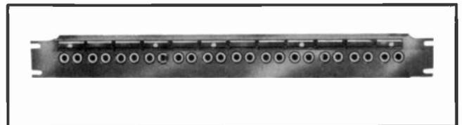
These panels are available in 12 pair, single row and 24 pair, double row models to fit any standard 19" rack and include such features as: solid 5/8" thick Bakelite panel with steel reinforcing; heavy gauge, special spring temper nickel/silver alloy leaves; ground lugs aligned to allow single ground bus to be run full length of strip; large palladium silver contacts; connection lugs fanned out for ease of soldering.
