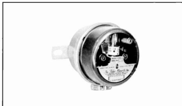
Designed to mount in a standard commercial meter socket. The 63305DB will automatically control broadcast tower lights directly or with auxiliary contactors. Adjustable potentiometer allows adjustment for operation from 0 to 50 f.c.
