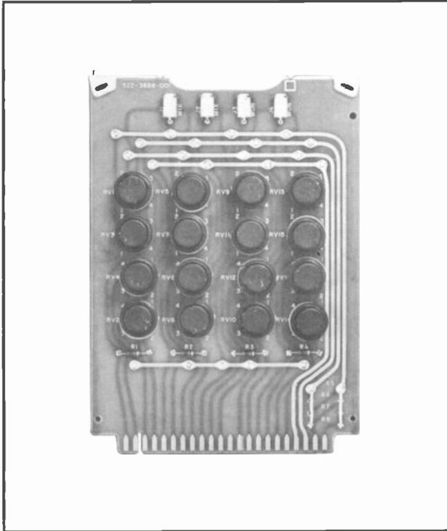
The 384D-1 is used in the 212S-1 and 212M-1 consoles to switch remote lines coming into the consoles.
