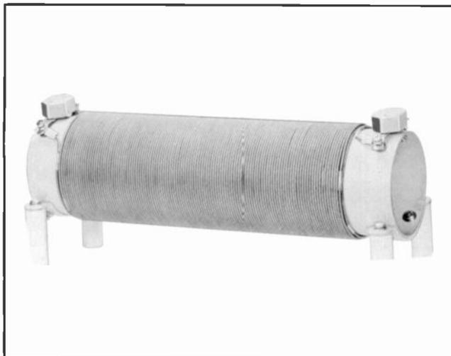
These solenoid wound 2- and 3-wire chokes provide high impedance throughout the broadcast band for isolation of the ac power lines from the antenna. Coils are wound of #10 wire and are rated at 2,000 watts, 120
