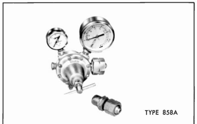
Type 858A Nitrogen Tank Fittings includes a pressure regulator, high and low pressure gauges and 10 feet of 3/8" O.D. polyethylene tubing with fittings to fit 1/8" pipe threads and adaptors to nitrogen tanks.
