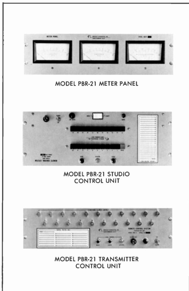
The PBR-21 represents a new concept in the design of broadcast and television transmitter remote control systems. The path between studio and transmitter is no longer restricted to DC line requirements. A single low cost, voice quality line or STL circuit is all that is necessary. Line attenuation up to 20 db will not adversely affect system operation.
