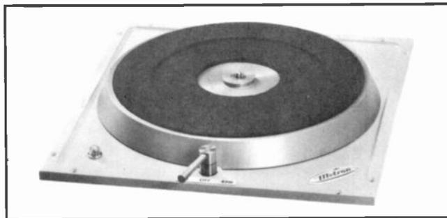
The TT-900 is a turntable designed specially for stereo operation and meets NAB specifications for stereo operation. The chassis is of heavy cast aluminum. A simple speed shift lever is located in the center of the chassis for choice of 2 speeds, 33⅓ and 45 rpm. In the off position the drive puck is removed from the rim to prevent flattening. An indentation in the platter eliminates the need for a spindle adapter for 7" 45 rpm records.
