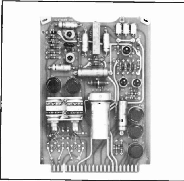
The 356T-1 is used with the 212S-1 and 212M-1 consoles in input channels where microphones are to be utilized.
