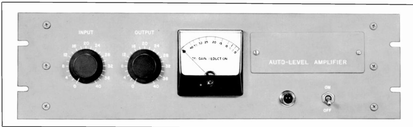
The average program level of the radio broadcast station can be automatically and effectively raised with the 26J-1 Auto-Level Limiting Amplifier. The resulting effect of the 26J-1 is similar to turning up the volume of the radio receiver so that the low level transmission is as well received as the high level transmission.
