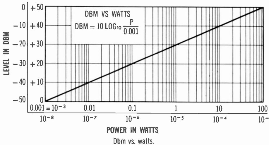
Dbm vs. watts.
