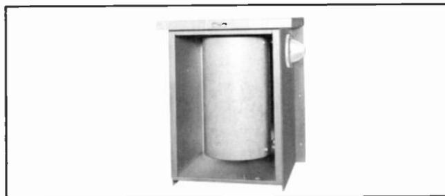
Coil provides isolation for the sampling line in directional arrays, presenting a high impedance for the line across the base insulator. Unit consists of a phenolic coil form which will accommodate 37 turns (approx. 100 ft.) of RG8/U or similar solid dielectric sampling line. May be mounted on wall of tuning shack or in housing similar to that pictured.
