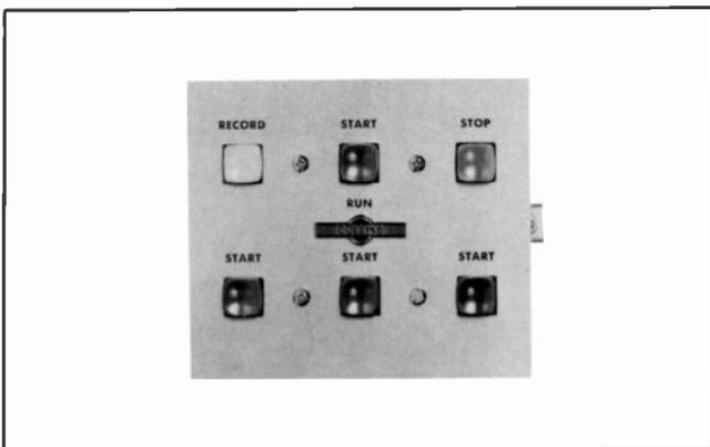
Three Collins automatic programming playback units, in addition to a record/playback system, may be operated with this control panel from a remote point in the broadcast studio. Buttons illuminate when in operation.
