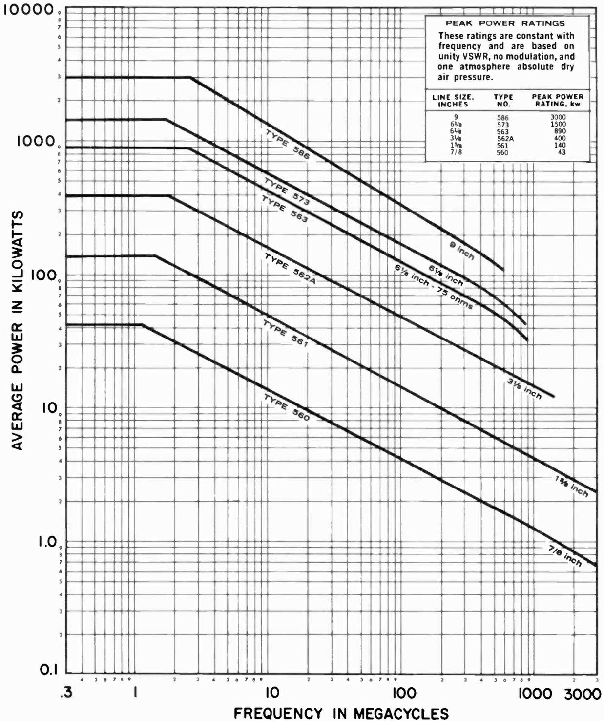
The average power ratings shown above are based on unity VSWR and a maximum inner conductor temperature of 216°F at an ambient temperature of 104°F.
