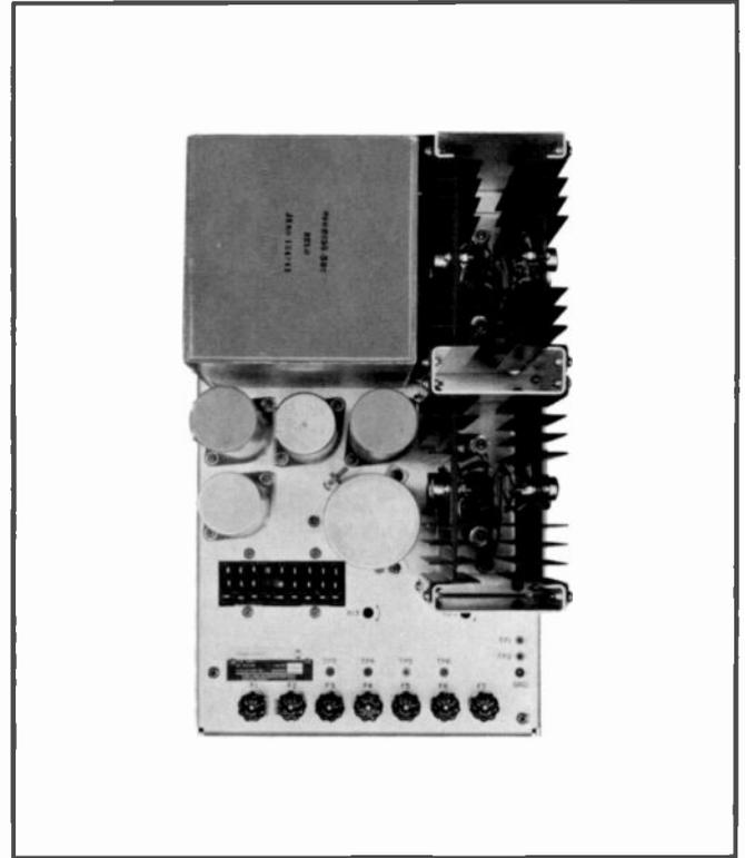
The 409Z-1 supplies the necessary voltage for the modules of the 212S-1 and 212M-1 consoles.
