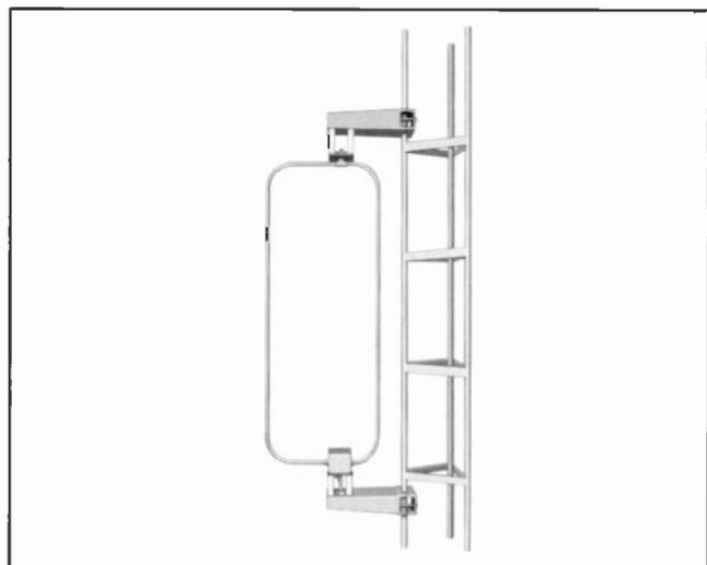
Designed to sample the relative phase relationship of radio frequency energy from 550-1600 kc antenna towers in directional antenna arrays, the Collins 564A-1 is made of two loops of #10 copper wire which may be connected either in series or in parallel. The wires are contained within a loop of 7/8" painted, copper tubing which serves as an electrostatic shield.
