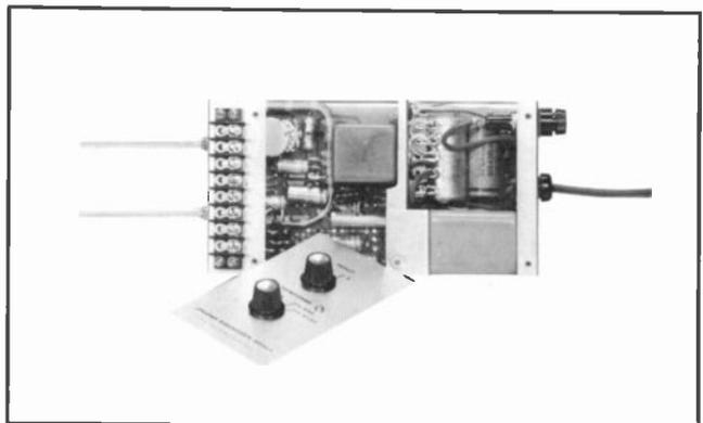
An economical unit to equalize and amplify the output signal of a magnetic phono cartridge, this small transistorized unit is used to replace passive equalizers and console or turntable preamplifiers. The housing of the unit is constructed of steel for magnetic shielding.
