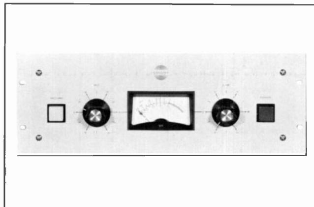
The 216C-2 Recording Amplifier is used with the 642A-2 Recorder/Playback Unit to provide facilities for recording pre-erased tape cartridges. This unit contains preamplifiers for 600-ohm line and 250-ohm microphone inputs, input level controls, and an output amplifier. The two inputs may be mixed if desired.
