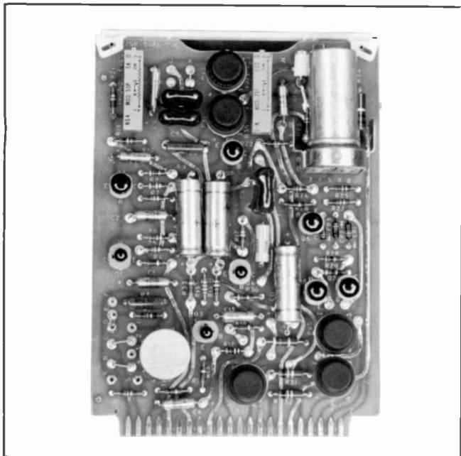
The 356R-1 amplifies and equalizes audio from a magnetic pickup or amplifies audio from a microphone. Two remotely switched inputs, three remotely switched outputs, and one direct output are provided.
