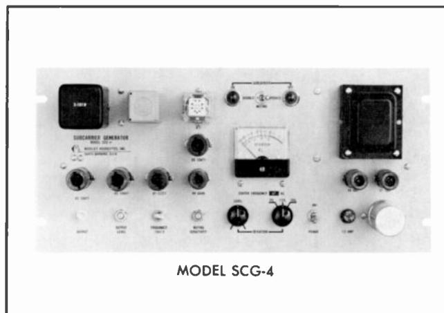
Designed to comply with F.C.C. Rules and Regulations for SCA operations, the Model SCG-4 Subcarrier Generator offers the FM broadcaster a reliable subcarrier generator for the transmission of a high fidelity SCA multiplex signal. This unit is compatible with FM stereophonic broadcasting. Precision components are utilized in the oscillator timing circuits to enhance the center frequency stability and to minimize effects of tube aging or replacement on the operating frequency.
