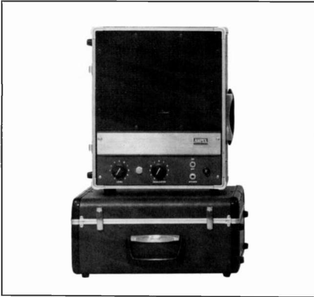
The 622 unit gives you "on-the-spot" studio-quality playback for demonstration or monitoring. Its 10 watt amplifier provides ample volume for a medium size auditorium.
