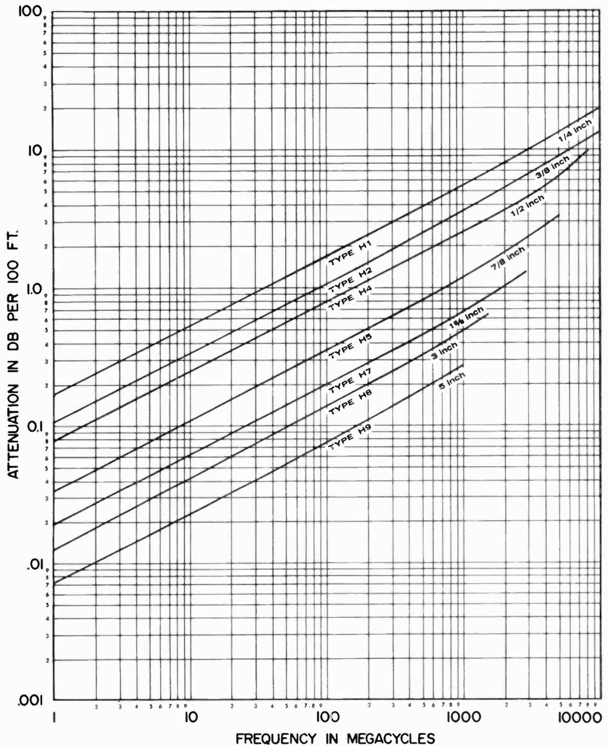
The attenuation curves above are for 50 ohm copper Heliax at unity VSWR. For 75 ohm copper cables the values shown should be reduced 5%. For 50 ohm aluminum (outer conductor) cables the values should be increased 12%.
