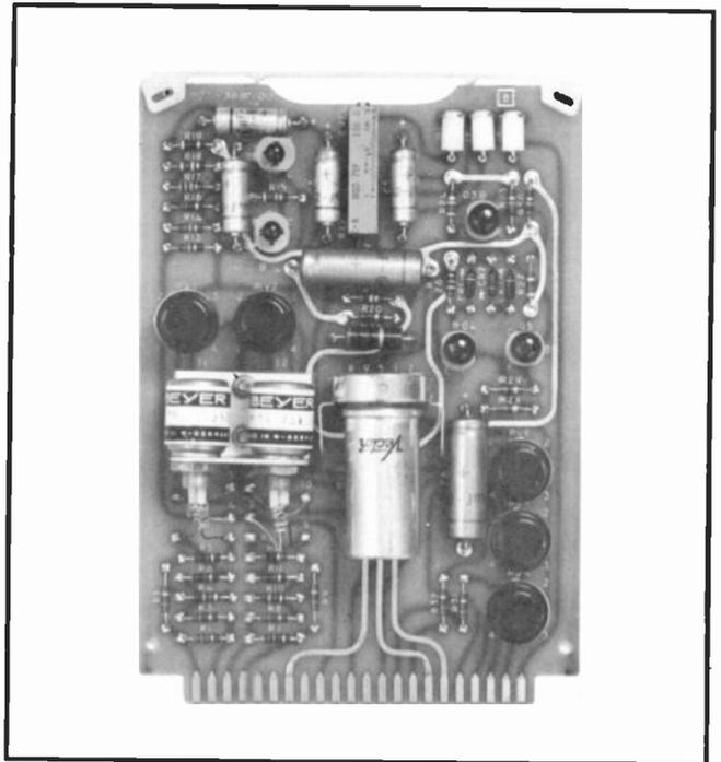
The 356V-1 is required for input channels for the 212S-1 and 212M-1 consoles where outputs of the turntable preamplifier, tape recorders, and other equipments with audio outputs between -10 DBM and +10 DBM are fed into the console.
