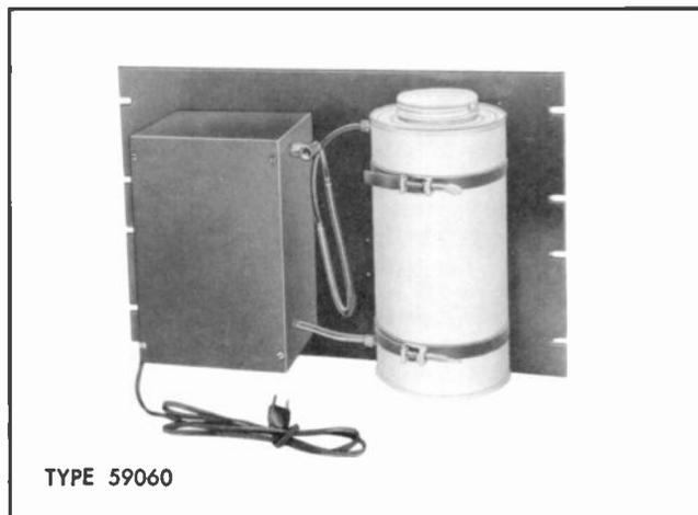
Type 59060, Low Pressure Dehydrator is ideal for pressurizing microwave waveguide systems or small air dielectric cables. This dehydrator maintains a constant pressure of dry air inside the waveguide or coaxial cable.
