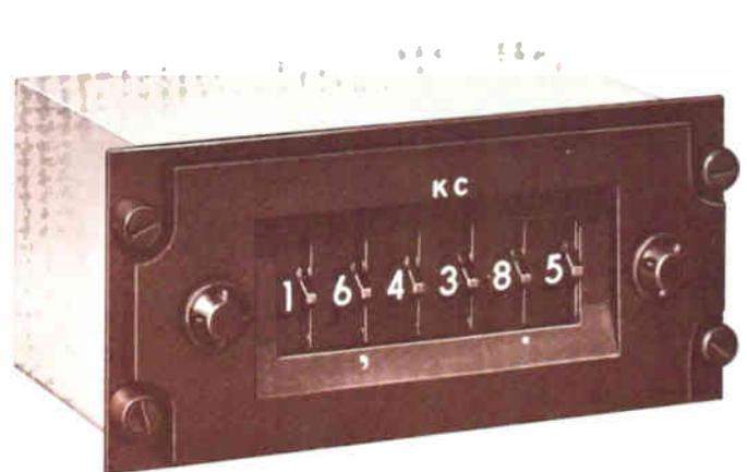
The 714Y-2 is a compact control unit for use with the Collins Universal Radio Group exciters, receivers or exciter-receivers. It allows remote selection of any of 280,000 channels with 0.1 kc spacing over the 2.0-29.999 mc frequency range. Thumb-index type knobs provide direct digital readout of the operating frequency. All frequency selection terminations are diode isolated for 200 ma current to allow paralleling of control units.
