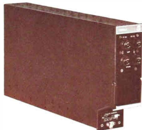
The 700B-2 consists of four plug-in modules on an aluminum chassis housed in a short  $\frac{1}{4}$  ATR case. All electrical connections are made through a single connector located at the rear. Test points on each module aid in performing maintenance checks. Reliability is greatly enhanced by the use of solid state components.
