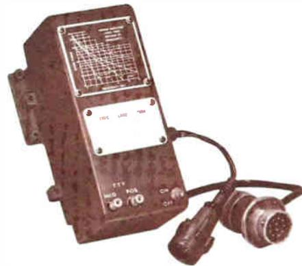
The 700C-1 is easily installed on the front panel and requires no wiring changes, adjustments or tuning. A switch and potentiometer are used to select the loop current option and adjust the current to the proper value. The teletypewriter can be located up to one mile from the AN/PRC-47. Terminals are included for connection of a remote push-to-talk switch.
