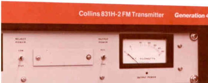
The new 40 KW 831H-2 transmitter is the top of the line in Collins **Generation 4** FM transmitters. The 831H-2 is recommended for Class B or Class C stations requiring solid close-in coverage combined with excellent fringe area reception. The 831H-2 allows a lower gain antenna to be utilized while still maintaining 50-100 KW ERP with circular polarization.
