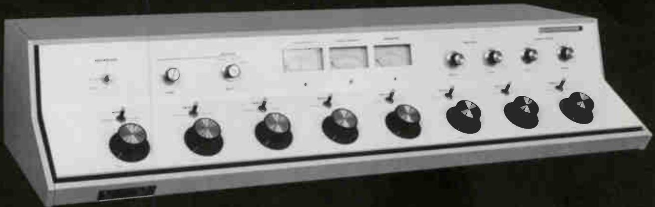
remote lines. The phono preamps are equalized for RIAA reproducing characteristic and strappable for 3-dB boost or cut. The mike preamps have a flat response and use transformer input. Impedances are easily selected by strapping. Both low level and high level inputs are available. The 212L-1 also has a mono output that will drive an AM transmitter while the stereo outputs are
