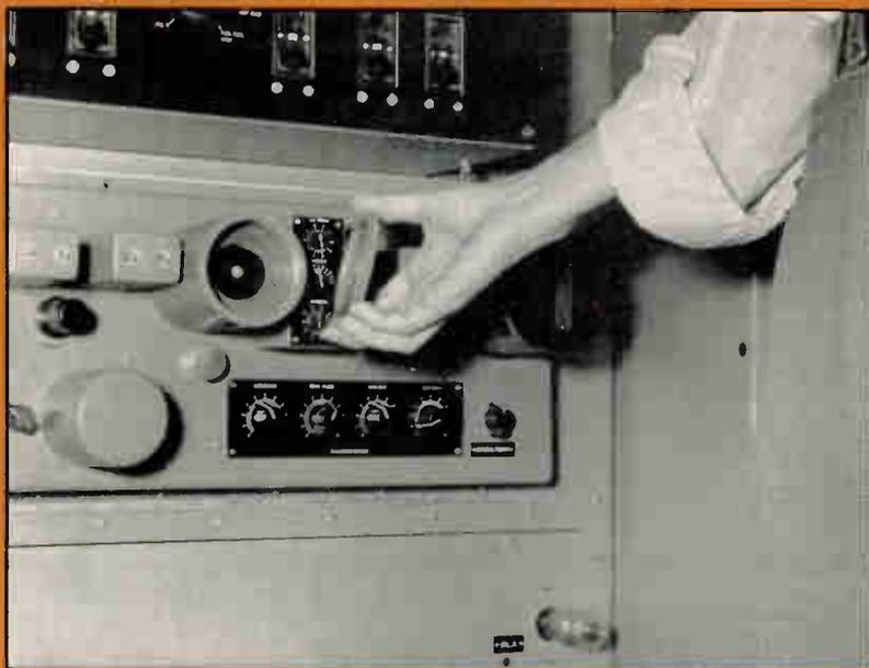
To remove the Phasitron, the operator exerts a small pulling force on the ejector knob which is immediately below the Phasitron shield.
