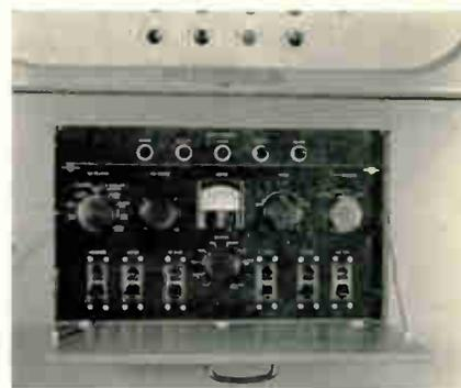
A small panel in the front door swings downward to reveal the transmitter controls. When it is lowered, the panel can be used as a desk while meter readings are being recorded. All switching and tuning controls are protected against accidental misadjustment when the panel is closed.
