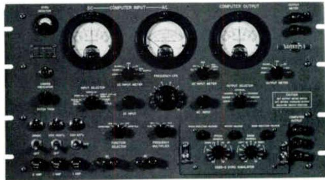
**478C-2 FD-104 IFS TEST SET** — Provides accurate simulated aircraft heading signals, lateral and vertical displacement signals, attitude signals, and rate of change of these signals as necessary for bench testing and calibrating the Collins 562A Steering Computers and components of the FD-104 IFS. Provides .001 to 10 cps signals for testing meter responses and servo mechanisms. No vacuum tubes are used. *Power Requirements:* 230 watts max. *Size:* 10½" H, 19" W, 12" D.
