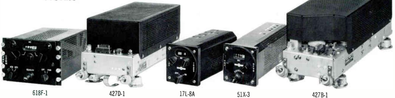
**618F-1 VHF COMMUNICATION SYSTEM** — The 618F-1 is a panel mounted, crystal-controlled transceiver providing 360 channel communication service with 50 kc spacing between channels in the 118.0-135.95 mc frequency range. It provides for single-channel-simplex (SCS) and double-channel-simplex (DCS) with direct frequency presentation. Only 9 $\frac{3}{4}$ " is required behind the panel, including space for rear connectors. Minimum transmitter output is six watts.
