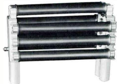
**172G-1, -2 DUMMY LOADS** — This air-cooled unit provides a load to dissipate transmitter output for off-the-air testing. Consisting of 8 ferrule type, non-inductive resistors, with insulated end brackets and clips, it may be mounted on the transmitter or adjacent wall. The 172G-1 has an impedance of 52 ohms; the 172G-2, 73 ohms. *Power Rating:* Up to 1 kw. *Size:* Approx. 6" W, 12 1/2" D, 9" H. *Weight:* 5 lbs.
