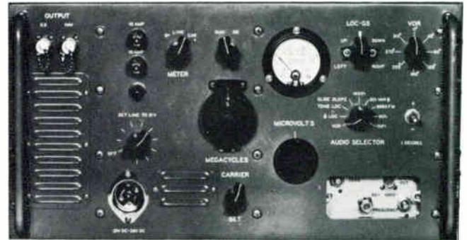
**479T-2 ALL CHANNEL VOR-ILS SIGNAL GENERATOR** — A portable test set for ramp testing of navigation and ILS receivers. May be used inside or outside the plane for an over-all check on the installation from receiving antenna to indicating instruments. Complete coverage of all channels from 108.0 through 135.9 and 329.3 through 335.0 mc. RF level can be varied from 4 to 200,000 microvolts. Signals include: VOR, LOC, glideslope, 1000 cps audio tone. Size: 19" W, 18" H, 10½" D.
