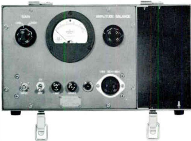
**478A-1 ZIFOR (Zero Indicator for Omni-range)** — Used for precisely ascertaining the proper zero, or North, setting on audio signal generators used in VOR testing and to set the zero on the Collins 479S series of test equipment and their equivalents. May also be used to check for phase shift through the RF signal generator. Used with the 479S-3. *Size: 13 $\frac{1}{2}$ " H, 13 $\frac{1}{2}$ " W, 7 $\frac{1}{2}$ " D.*
