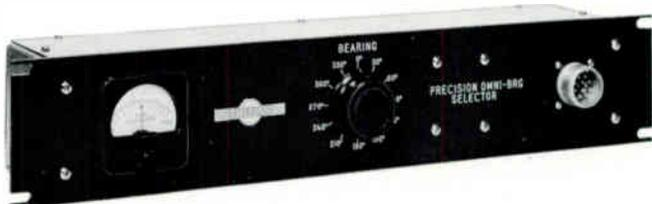
**479V-2 PRECISION OMNI-BEARING SELECTOR** — Used for a test panel for checking the 344A-1, 51R-3 and earlier navigation receivers. 30° steps selected by a tap switch with a maximum runout error of ±.05°. Tests the receiver without introducing omni-bearing selector errors. *Weight:* 5 lbs. *Size:* 3½" H, 19" W, 4" D.
