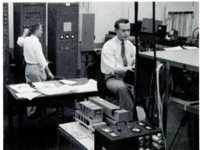
FLIGHT SIMULATOR, using analog computer, enables laboratory duplication of aeronautical conditions for analysis of airborne electronic systems.
