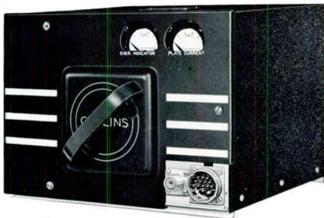
**180M-1 ANTENNA TUNING UNIT TEST SET** — A manually adjustable network used to minimize the time required to determine the circuit elements which must be wired into the 180K-3. Circuits and values of capacitance and inductance selected by front panel controls. *Size: 7 $\frac{3}{4}$ " H, 10 $\frac{1}{4}$ " W, 9 $\frac{7}{8}$ " L.*
