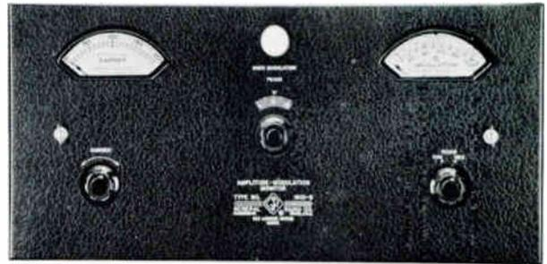
**1931-B AM MODULATION MONITOR** — Measures percentage modulation on positive or negative peaks, indicates over-modulation, monitors program level and measures transmitter audio frequency response and carrier shift when modulation is applied. Operates in either 0.5 to 8 mc range or 3 to 60 mc range, depending on input coil used. *Primary Power:* 105-125 v, 50/60 cps, 50 watts. *Size:* 19" W, 10" D, 8 3/4" H. *Weight:* 32 lbs.
