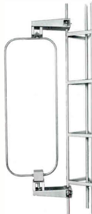
**564A-1 PHASE SAMPLING LOOP** — For accurate sampling of currents in directional arrays. Two loops of wire, connected in series or parallel, inside a copper tubing shield which eliminates electrostatic coupling. Connects with air or solid dielectric line. *Size:* Approx. 30" W, 7'6" H. *Weight:* 50 lbs.
