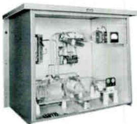
**81M PHASORS** — Custom designed Collins phasing equipment for directional antennas features easily adjusted networks, high stability, maintenance ease, safety and economy. Power dividing circuits and T phase shift networks utilize heavy edge-wound copper ribbon inductors and ceramic cased mica capacitors. Amplitude and phase adjustment controls are recessed counter dials with accurate resetability.
