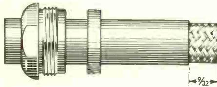
Place nut and gasket over cable and cut off jacket  $\frac{9}{32}$ " from end.
