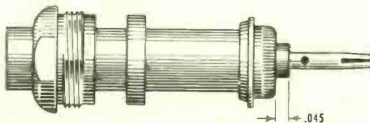
Fold back braid wires as shown, trim to proper length and form over clamp as shown. Solder contact to center conductor.
