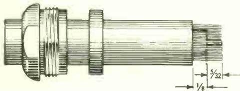
Comb out braid and fold out. Cut off cable dielectric flush  $\frac{1}{8}$ " from end of jacket.
