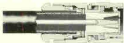
Insert cable and parts into connector body. Make sure sharp edge of clamp seats properly in gasket. Tighten nut.
