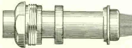
Pull braid wires forward and taper toward center conductor. Place clamp over braid and push back against cable jacket.
