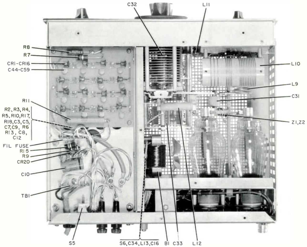
Figure 6-1. R-F and Power Supply Compartments, Parts Location
