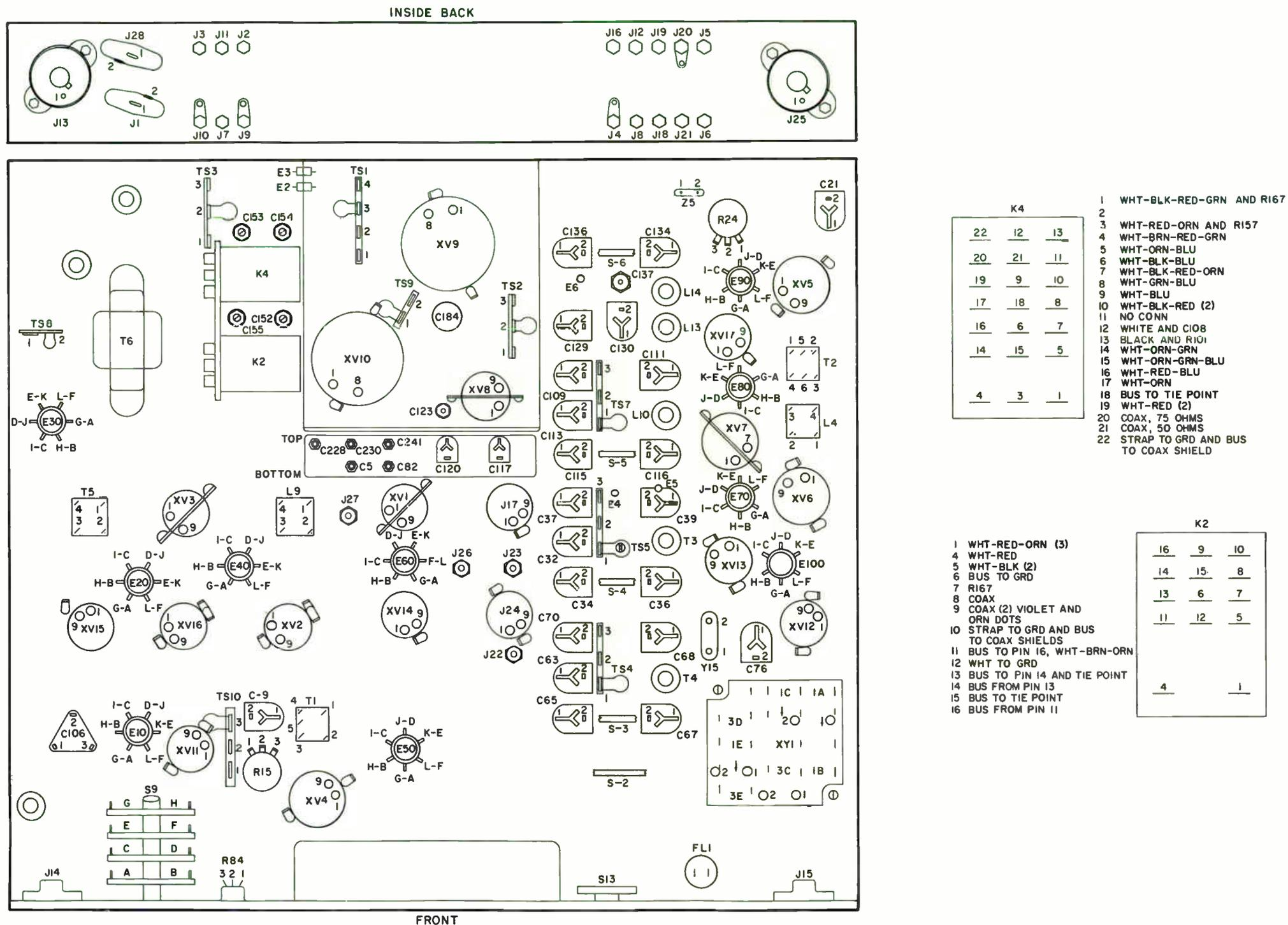
Figure 7-2. KWM-2 and KWM-2A, Location of Chassis Mounted Components, Bottom View
