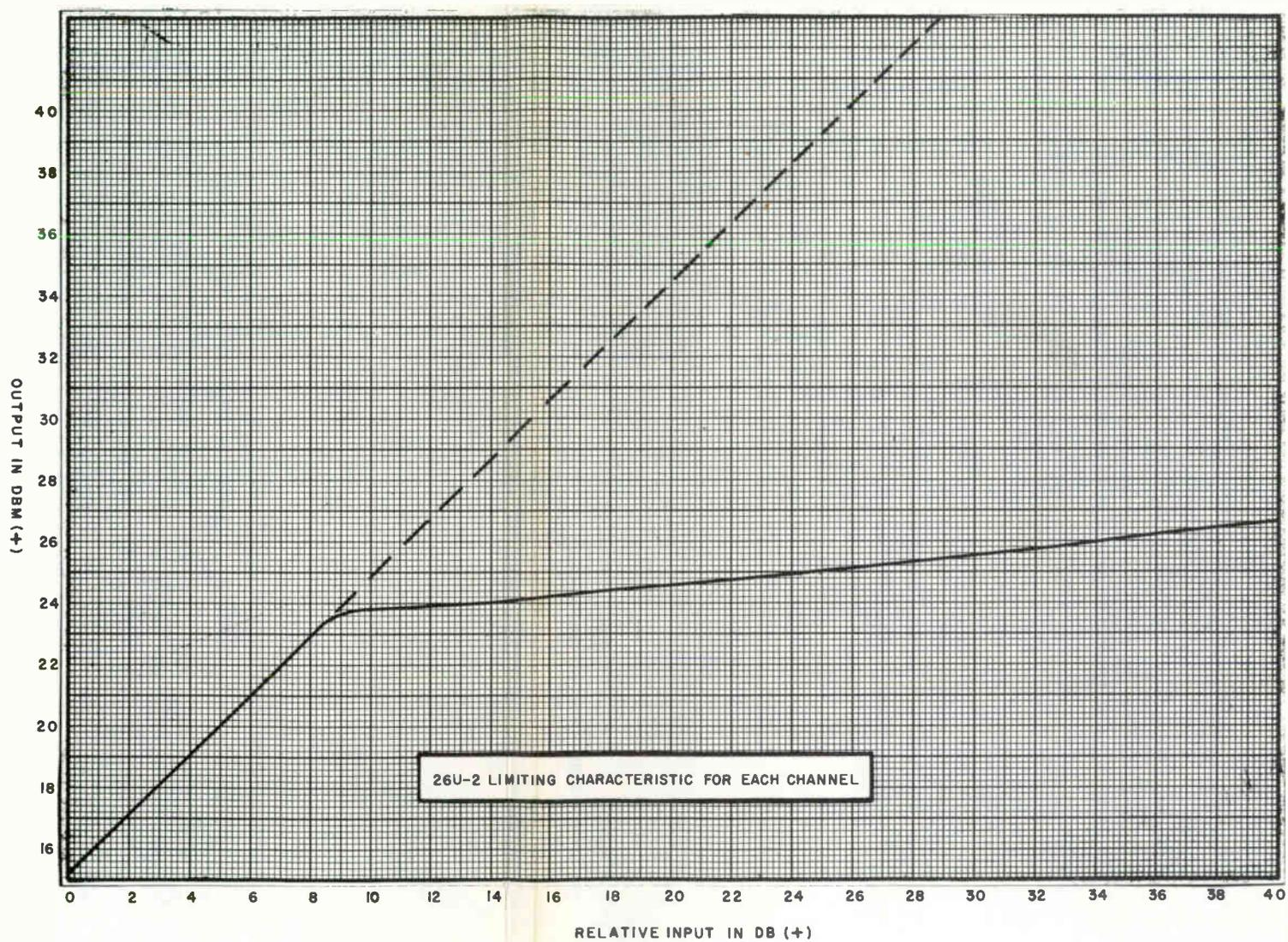
Figure 1-3. 26U-2 Stereo Peak Limiter,
