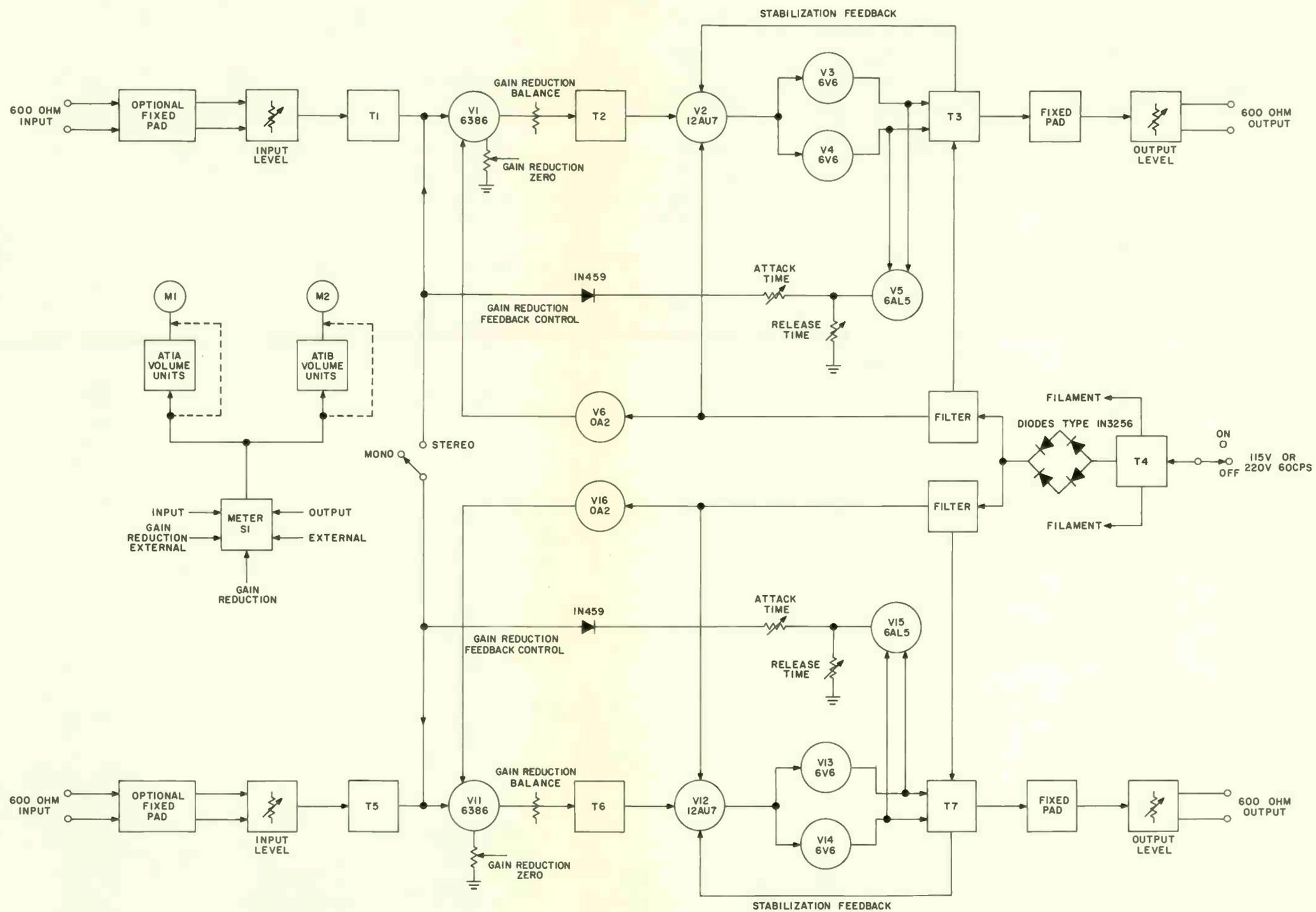
Figure 4-1. 26U-2 Stereo Peak Limiter, Block Diagram
