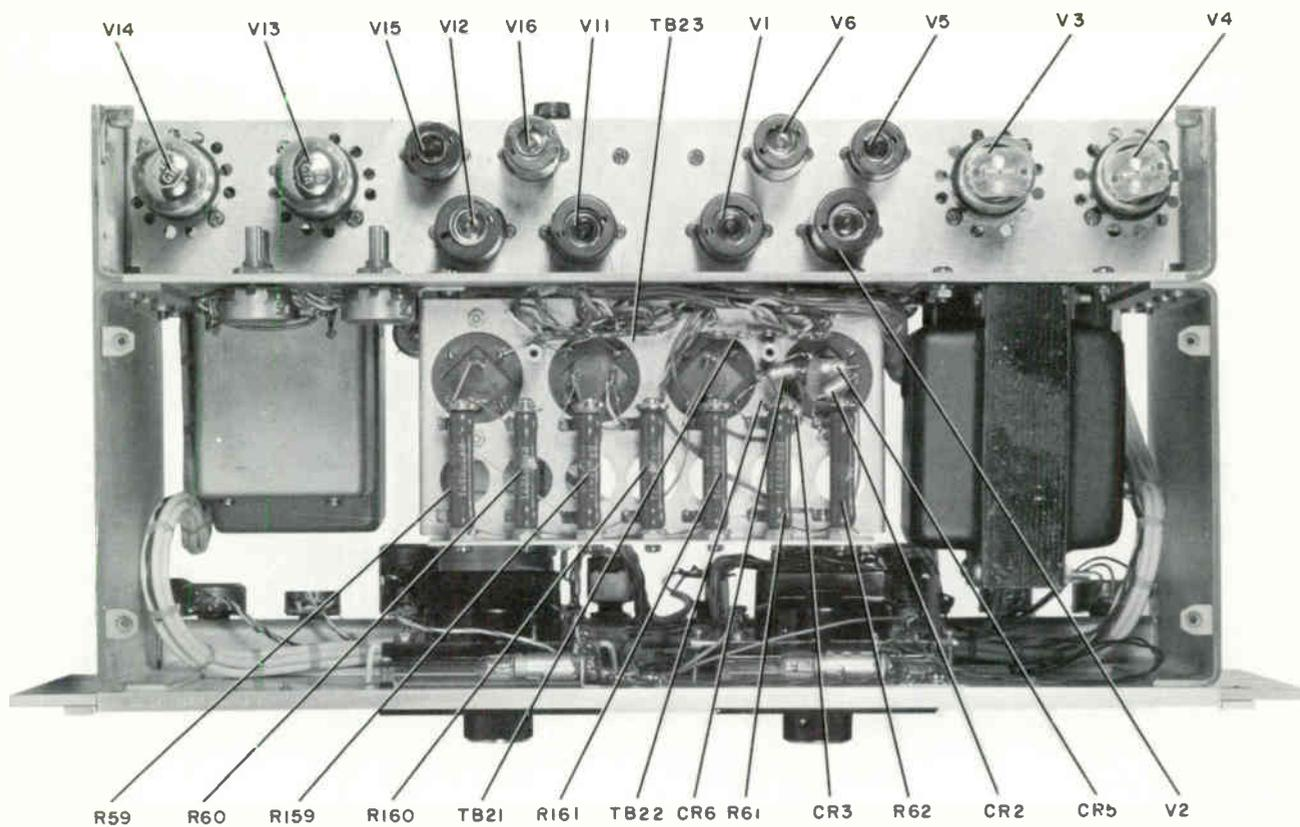
Figure 6-4. 26U-2 Stereo Peak Limiter, Top View
