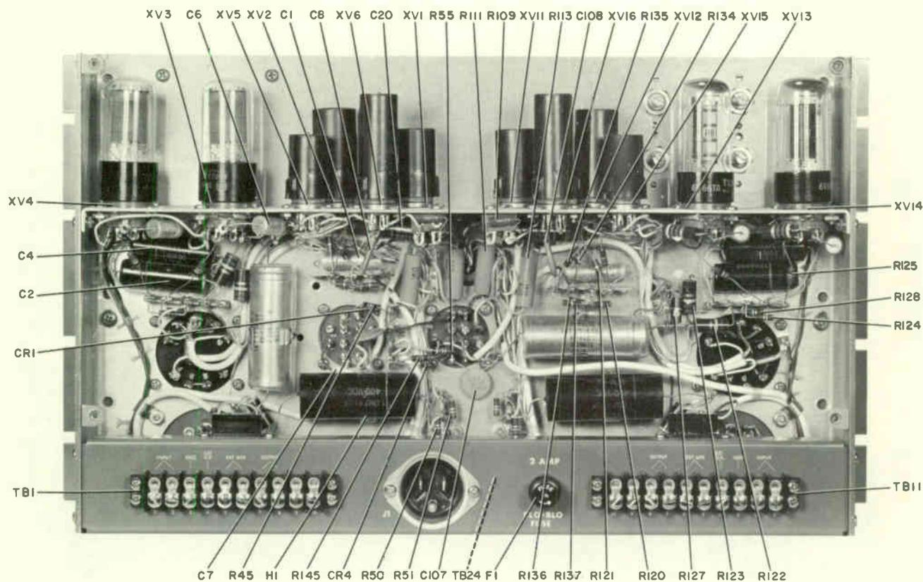
Figure 6-2. 26U-2 Stereo Peak Limiter, Inside Back View
