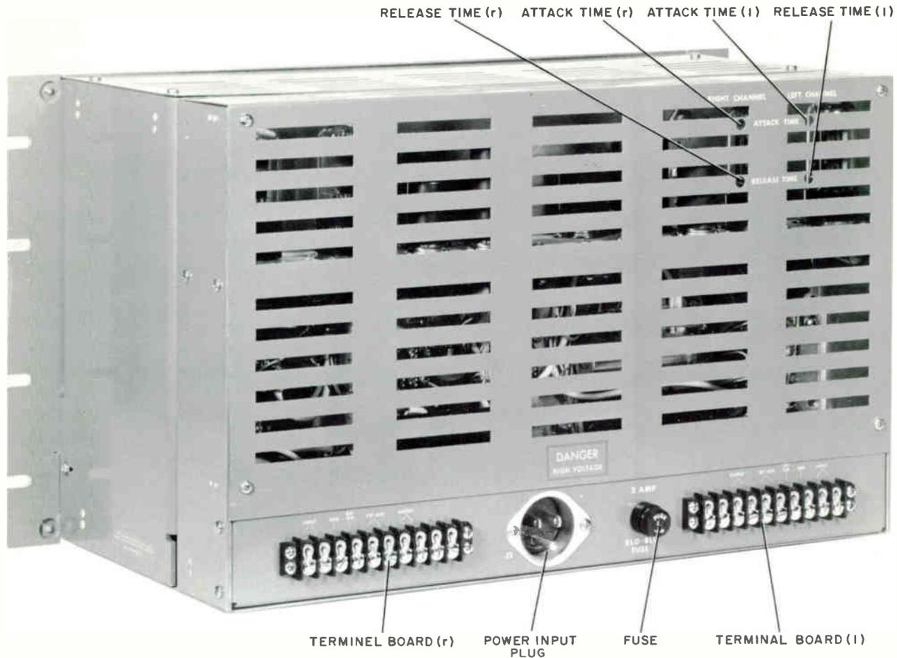
Figure 3-2. Operational Controls, Rear View
