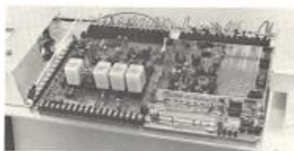
- One solid state board controls the transmitter and pulse width modulation.
