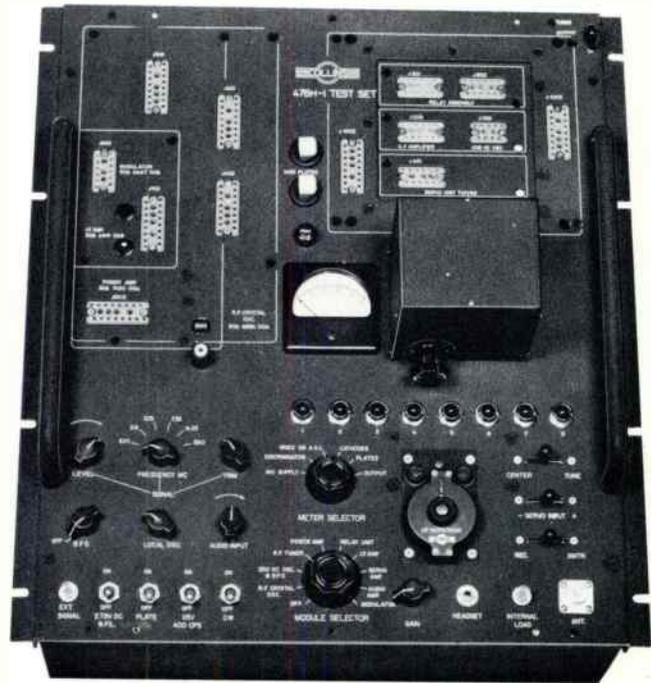
**478H-1 618S TEST SET** — The 478H-1 and associated 413F-1 Power Supply provide complete self-contained facilities for testing modular subassemblies of the 618S. Also provides a convenient test station for detailed circuit checks. The lower portion of the test set panel carries all operating controls required to simulate functions of the complete 618S Transceiver. *Weight: 35 lbs. Size: 19 $\frac{3}{4}$ " H, 17 $\frac{1}{2}$ " W, 8" D.*
