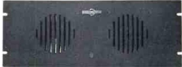
**271B SPEAKERS** — The 271B-3 is a dual speaker panel; the 271B-4, a single speaker panel. Each speaker has a 600-ohm-to-voice-coil-impedance matching transformer and a terminal board. *Size:* 19" W, 4" D and 7" H. 271B-3—6.3 lbs. 271B-4—4 lbs.
