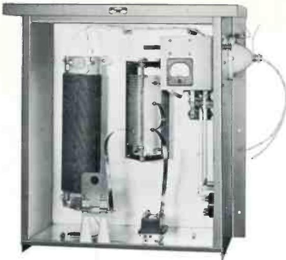
**42E-7, -8 ANTENNA COUPLING UNITS** — Use a low pass T network to match a series fed vertical radiator to an unbalanced transmission line. The 42E-7 (pictured) is used up to 1 kw; the 42E-8, 5 or 10 kw. Includes antenna current meter and line current meter jack and will house tower lighting filter choke and antenna current transformer. *Size:* 42E-7 — 29" W, 18" D, 28" H. 42E-8 — 36" W, 22" D, 28" H. *Weight:* 42E-7 — 64 lbs. 42E-8 — 124 lbs.
