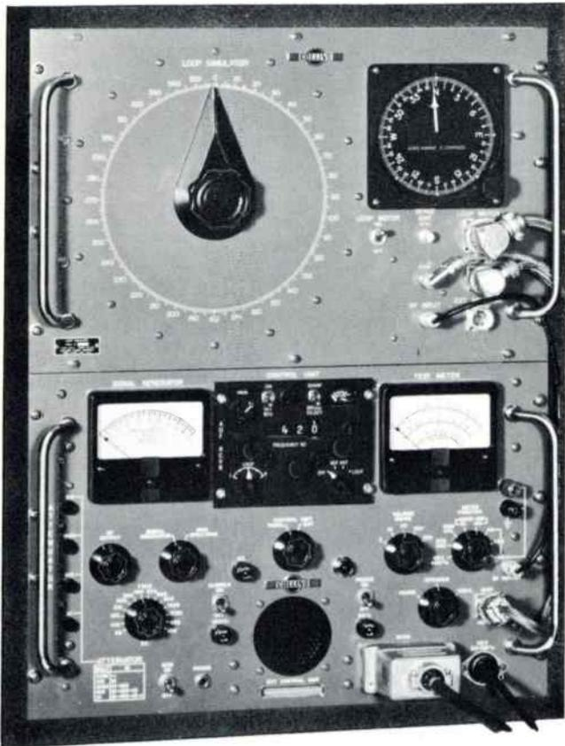
**477U-1, 477V-1 ADF TEST SET** — Provides complete test and simulator signals for the DF-201 ADF. The 477U-1 ADF Loop Simulator generates a calibrated RF field and excites a contained loop antenna. Receiver bearing indications are displayed on the front panel. The 477V-1 tests antenna, loop, ADF aural and ADF bearing sensitivity, dial calibration, bearing speed, AVC and gain control characteristics, and makes test point measurements on individual modules. *Mounting:* Rack or carrying case.
