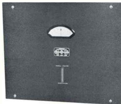
**1181-B FREQUENCY DEVIATION MONITOR** — Gives direct indications of magnitude and direction of frequency deviation of AM transmitter. Positive indication is provided for failure of either transmitter carrier or monitor crystal oscillator. *Frequency Range:* 0.5-2 mc (specify crystal frequency). *Deviation Range:* ± 30 cps. *Primary Power:* 105-125 or 210-250 v, 50/60 cps, 125 watts. *Size:* 19" W, 13" D, 15 3/4" H. *Weight:* 51 lbs.
