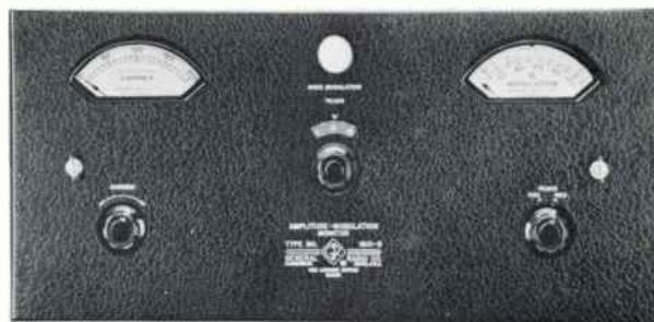
**1931-B AM MODULATION MONITOR** — Measures percentage modulation on positive or negative peaks, indicates over-modulation, monitors program level and measures transmitter audio frequency response and carrier shift when modulation is applied. Operates in 0.5 to 8 mc range. *Primary Power:* 105-125 v, 50/60 cps, 50 watts. *Size:* 19" W, 10" D, 8 3/4" H. *Weight:* 32 lbs.
