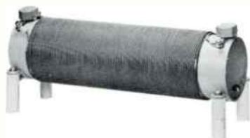
**TOWER LIGHTING FILTER CHOKES** — Solenoid wound chokes with high impedance in broadcast band. Wound with #10 wire, available 2 or 3 wire. *Power Rating:* 120 v, 1 phase, 2,000 watts.
