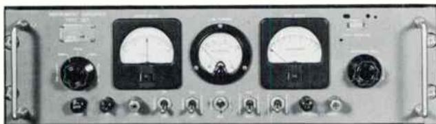
**477M-1 INSTRUMENT AMPLIFIER TEST SET** — Simulates signals identical to those in the 344C-1 Instrument Amplifier input circuits under actual flight conditions. Separate meters measure line currents, servo amplifier output and flag currents. Rack mounting.
