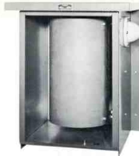
**144A-1 ISOLATION COIL** — Coil provides isolation for the sampling line in directional arrays, presenting a high impedance for the line across the base insulator. Unit consists of a phenolic coil form which will accommodate 37 turns of RG8/U or similar solid dielectric sampling line. May be mounted on wall of tuning shack or in 49U-1 Housing (pictured). *Inductance:* Approx. 180 microhenrys. *Size:* 10" dia., 18" L. *Weight:* 6 lbs.
