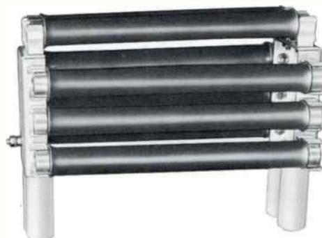
**172G-1, -2 DUMMY LOADS** — This air-cooled unit provides a load to dissipate transmitter output for off-the-air testing. Consisting of 8 ferrule type, non-inductive resistors, with insulated end brackets and clips, it may be mounted on the transmitter or adjacent wall. The 172G-1 has an impedance of 52 ohms; the 172G-2, 73 ohms. *Power Rating:* Up to 1 kw. *Size:* Approx. 6" W, 12 1/2" D, 9" H. *Weight:* 5 lbs.
