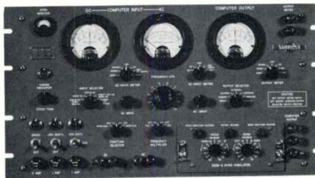
**478C-2 FD-104 IFS TEST SET** — Provides accurate simulated aircraft heading signals, lateral and vertical displacement signals, attitude signals, and rate of change of these signals as necessary for bench testing and calibrating the Collins 562A Steering Computers and components of the FD-104 IFS. Provides .001 to 10 cps signals for testing meter responses and servo mechanisms. No vacuum tubes are used. *Power Requirements:* 230 watts max. *Size:* 10½" H, 19" W, 12" D.
