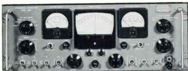
**477N-1 STEERING COMPUTER TEST SET** — Simulates selected heading, bank and course datum signals normally supplied to the 562A-5 Steering Computer. All important circuit functions may be tested and adjustments implemented. Complete test takes 15 min. Rack mounting.
