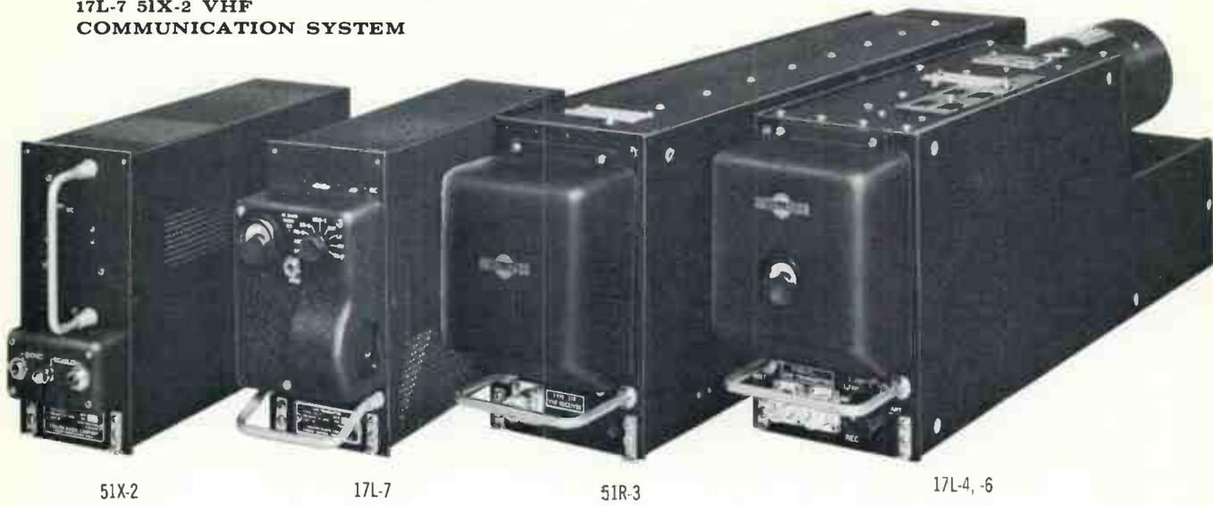
**51R-3 VHF COMMUNICATION/NAVIGATION RECEIVER** — A 280 channel crystal-controlled receiver with 100 kc spacing between 108.0 and 135.9 mc. Receives all VOR/LOC and communication frequencies and with the accessory frame and accessories provides full instrumentation facilities. *Shockmount:* 350E-3A. External power supply required.
