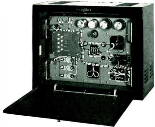
A wall mounting Power Supply for the 212A console, it contains three supplies which furnish d-c power for preamplifiers, monitor and line amplifiers, and 12 volts for relay operation. In addition, it furnishes 6.3 volts a-c to operate all tubes in the console.
