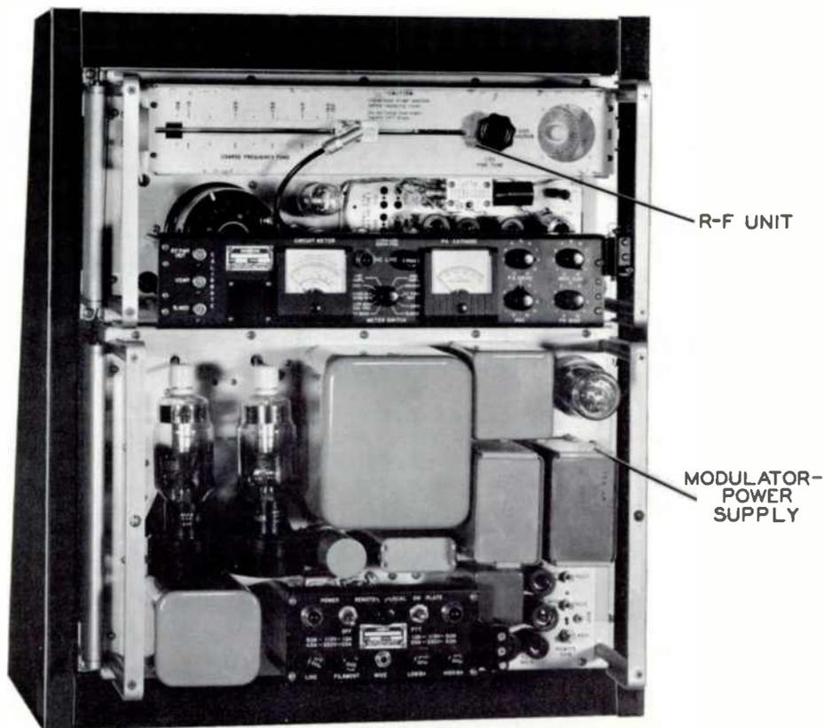
Figure 2-1. VHF Transmitter 242F-5CL, Hinge Mounted
