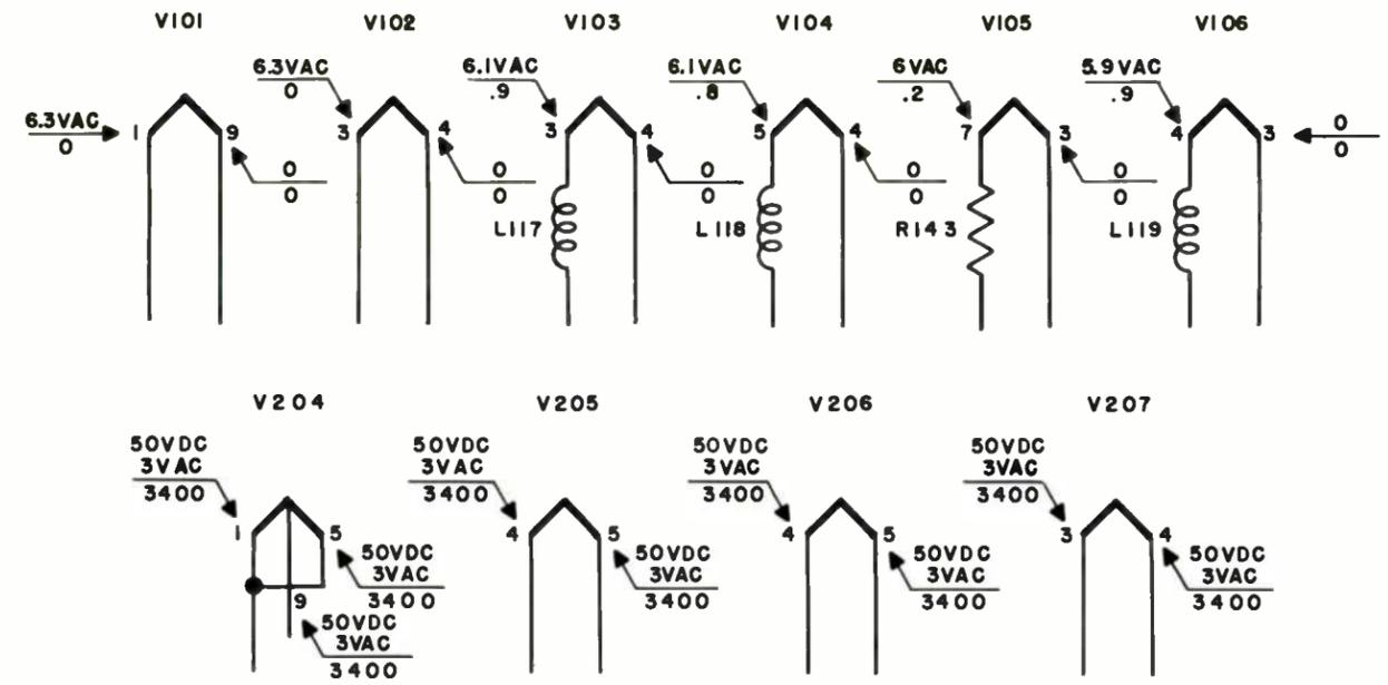
Figure 6-2. Filament Voltage and Resistance Measurements
