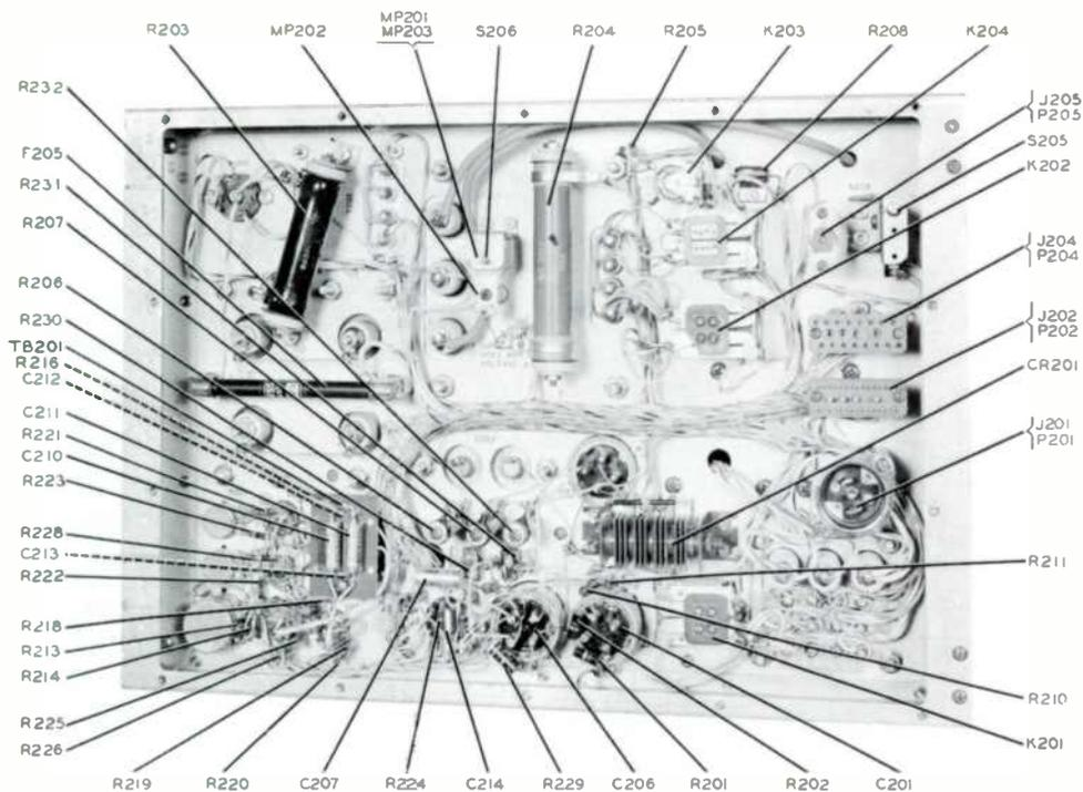
Figure 7-7. Modulator-Power Supply, Rear View, Dust Cover Removed
