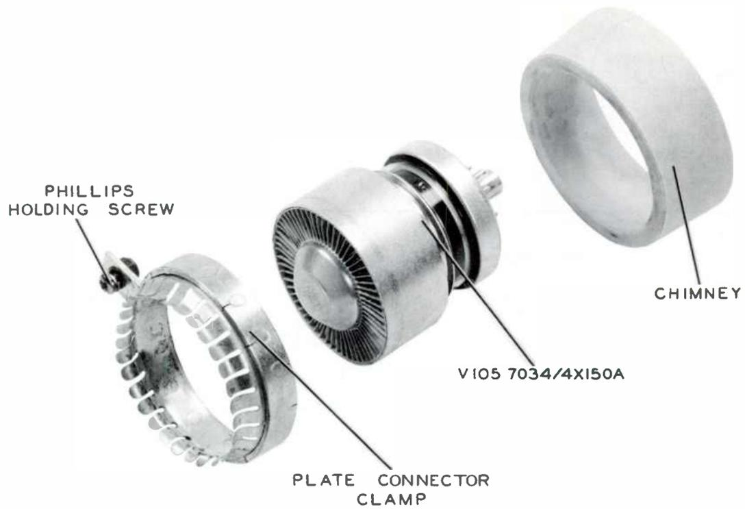
Figure 6-4. Power Amplifier Tube Assembly
