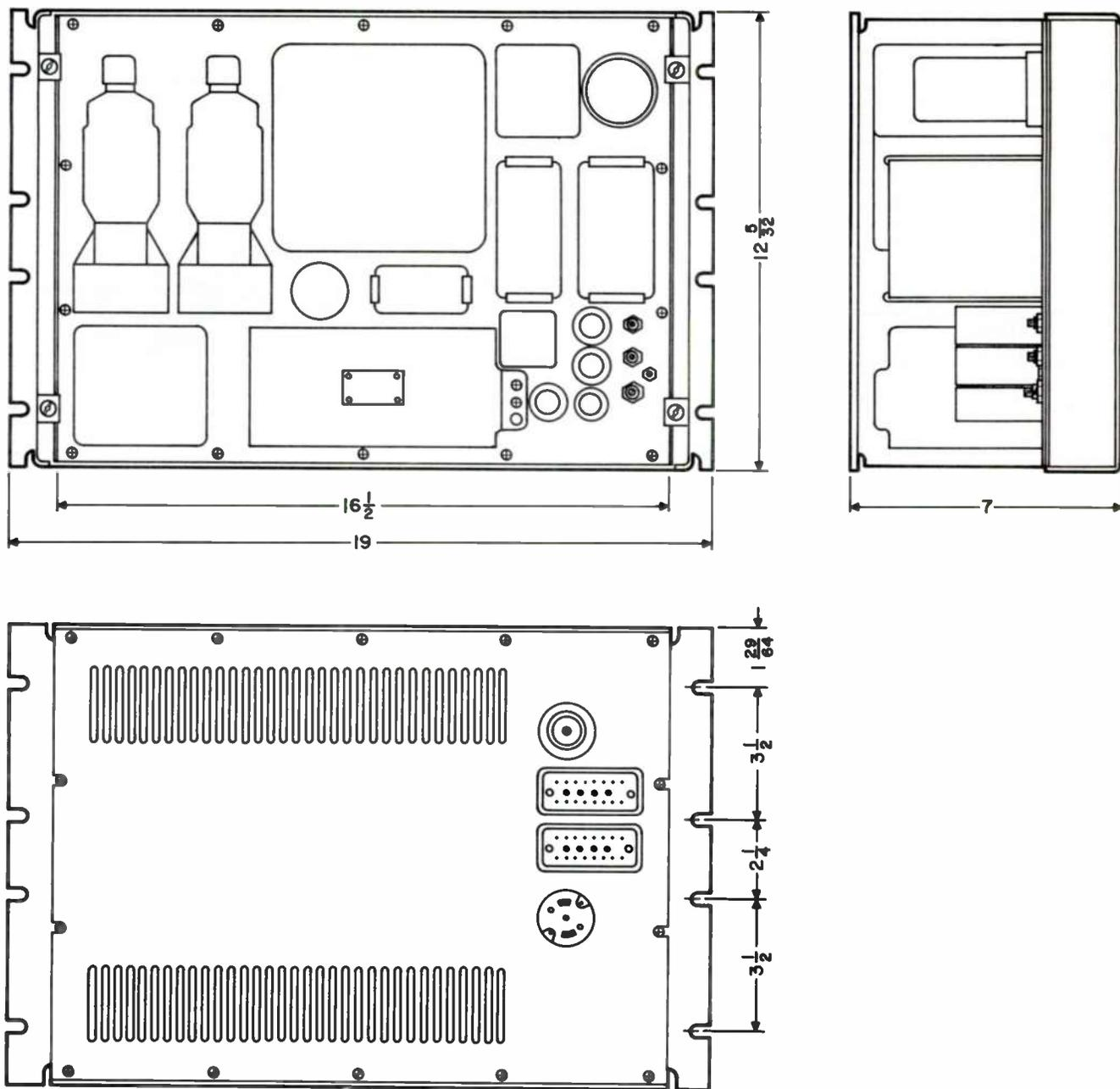
Figure 2-5. Modulator-Power Supply, Flush Mounting Installation Diagram
