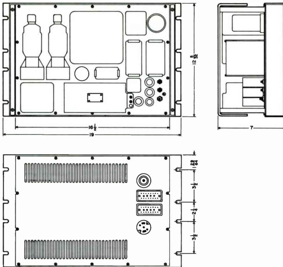
Figure 2-3. Modulator-Power Supply, Midrail Installation Diagram
