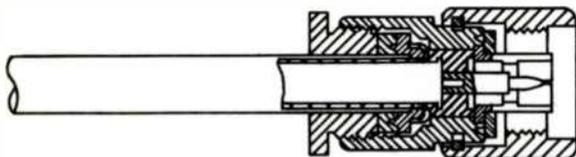
THE ASSEMBLY FOR PLUGS IS THE SAME AS ABOVE EXCEPT FOR THE USE OF FEMALE CONTACTS AND A JACK BODY.
