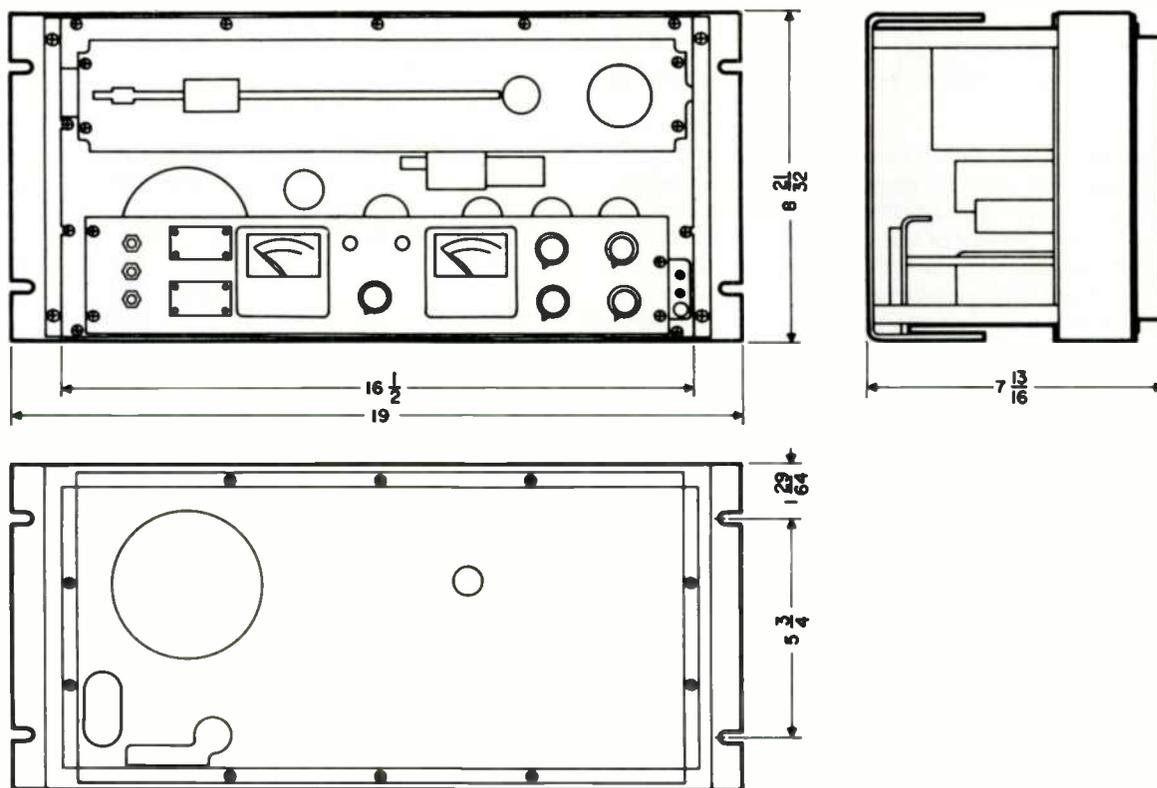
Figure 2-2. R-F Unit, Midrail Installation Diagram
