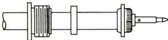
4. FOLD BRAID BACK OVER CLAMP AND TRIM. TIN INSIDE HOLE OF CONTACT. SLIP CONTACT INTO PLACE AND SOLDER. REMOVE EXCESS SOLDER. BE SURE CABLE DIELECTRIC IS NOT HEATED EXCESSIVELY AND SWOLLEN EXCESSIVELY SO AS TO PREVENT DIELECTRIC ENTERING BODY.
