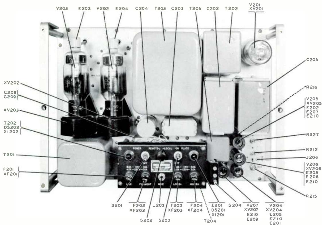
Figure 7-6. Modulator-Power Supply, Front View Dust Cover Removed
