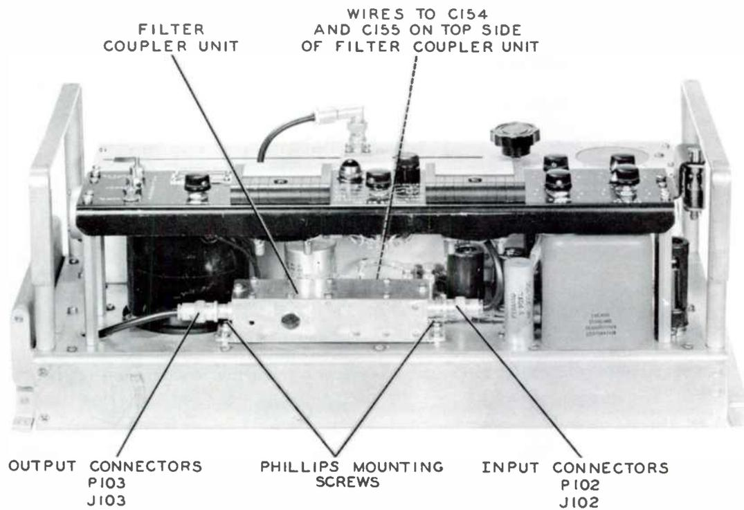
Figure 6-5. R-F Unit, Bottom View Showing Filter Coupler Unit
