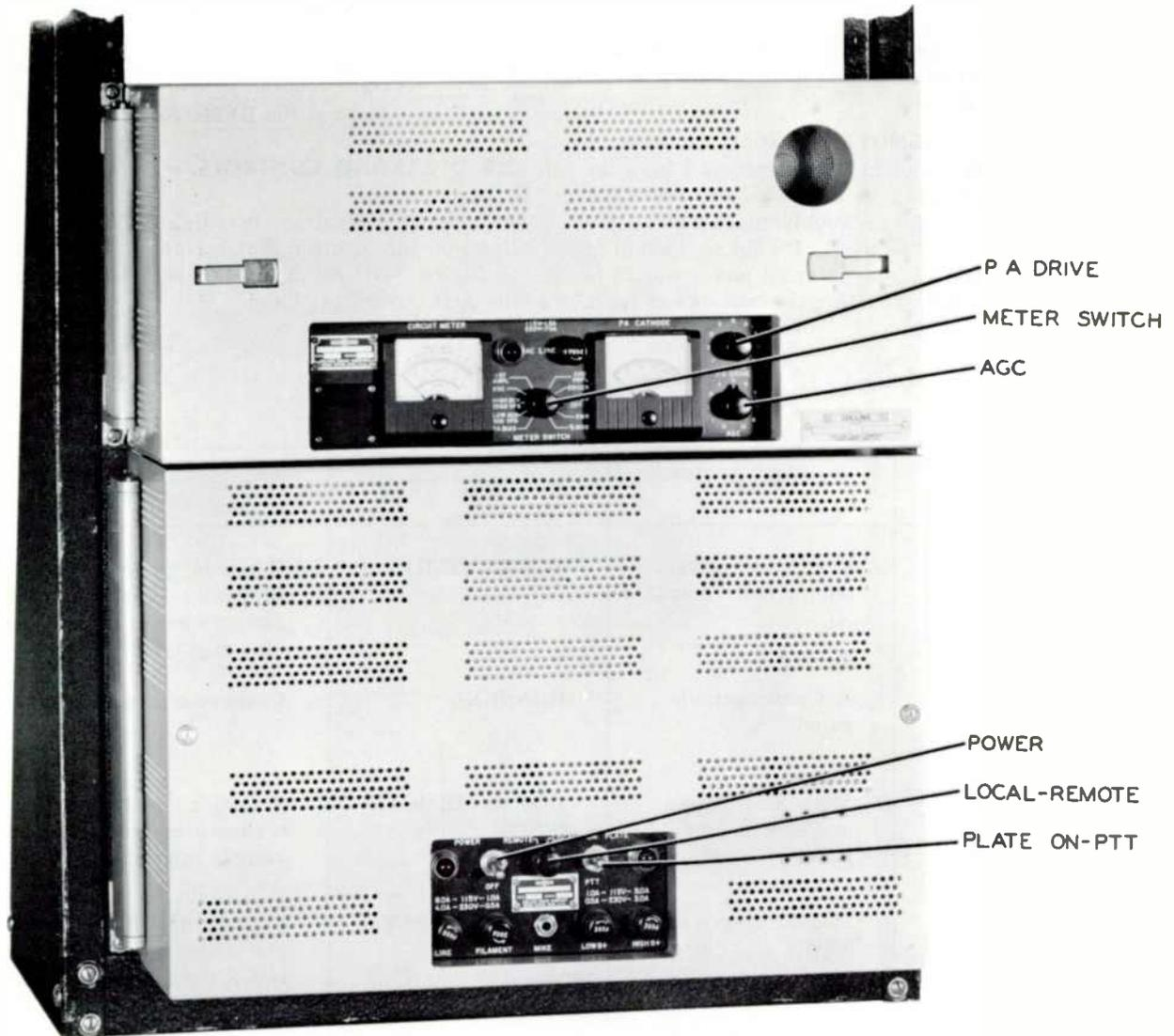
Figure 3-1. VHF Transmitter 242F-5CL, Operating Controls
