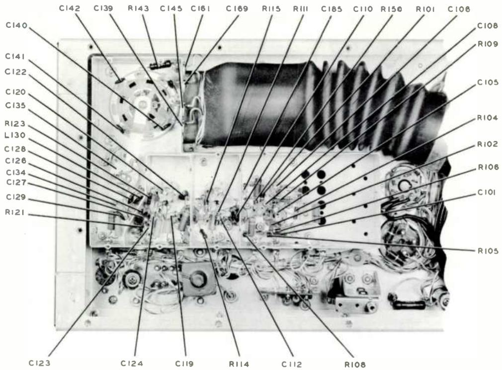
Figure 7-4. R-F Unit Subassembly, Cover Plate Removed
