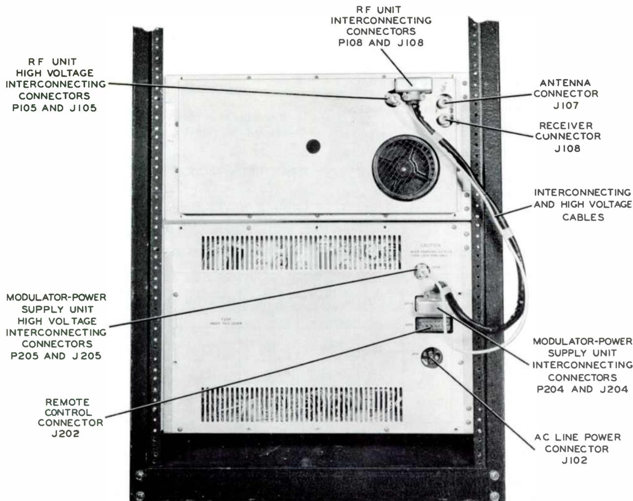
Figure 2-7. VHF Transmitter 242F-5CL, Cabling Connections
