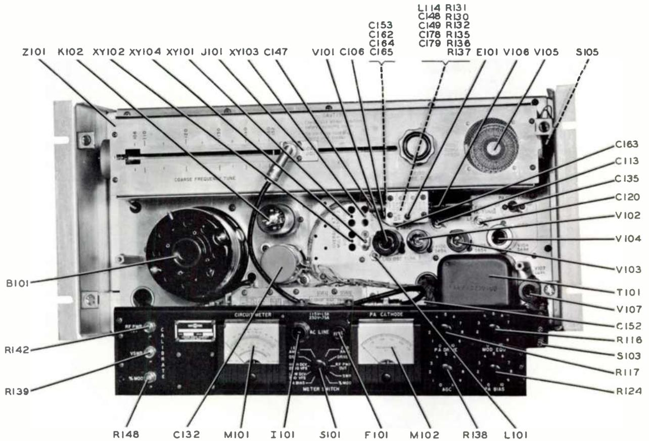
Figure 7-1. R-F Unit, Front View, Dust Cover Removed, Control Panel Dropped
