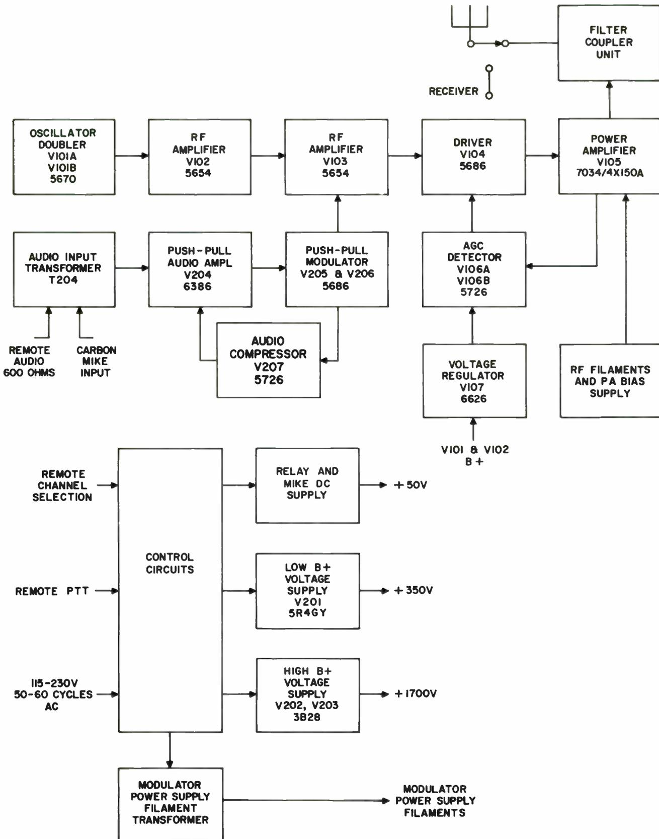
Figure 4-1. VHF Transmitter 242F-5CL, Block Diagram
