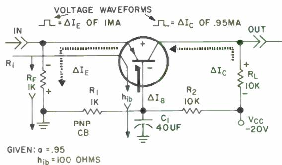
$$R_i \cong \frac{R_E \times h_{ib}}{R_E + h_{ib}}$$
