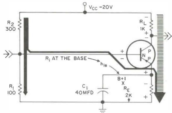
NOTE:  $V_{BE}$  IS NOT DEPENDENT UPON THE TRANSISTOR AS THE  $R_1$  AT THE BASE IS  $> 10 \times R_1$
