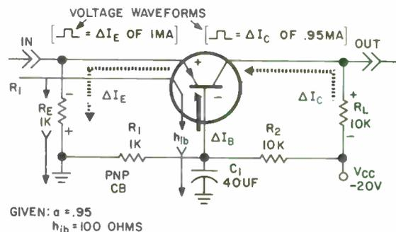
$$\left[ \begin{array}{l} R_i \cong \frac{R_E \times h_{ib}}{R_E + h_{ib}} \\ h_{ib} \cong 25 \text{ TO } 100 \text{ OHMS} \\ \text{IF } R_E \leq 10 \times h_{ib} \text{ THEN } R_i \cong h_{ib} \\ R_i \cong 100 \text{ OHMS} \end{array} \right]$$
