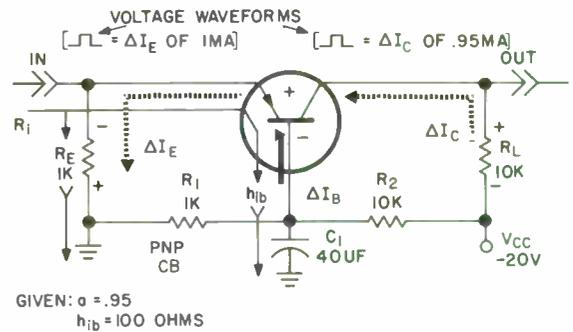
$$R_i \cong \frac{R_E \times h_{ib}}{R_E + h_{ib}}$$
