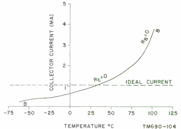
The fact that this is an undesirable effect of the transistor, that must be compensated for, is shown by the curve shown in figure 3-43. As can be seen, with  $R_E$  equal to zero and the base resistance,  $R_B$ , which equals the parallel values of  $R_1$  and  $R_2$  equal to approximately zero, the collector current changes by a large amount for a given change in temperature.
