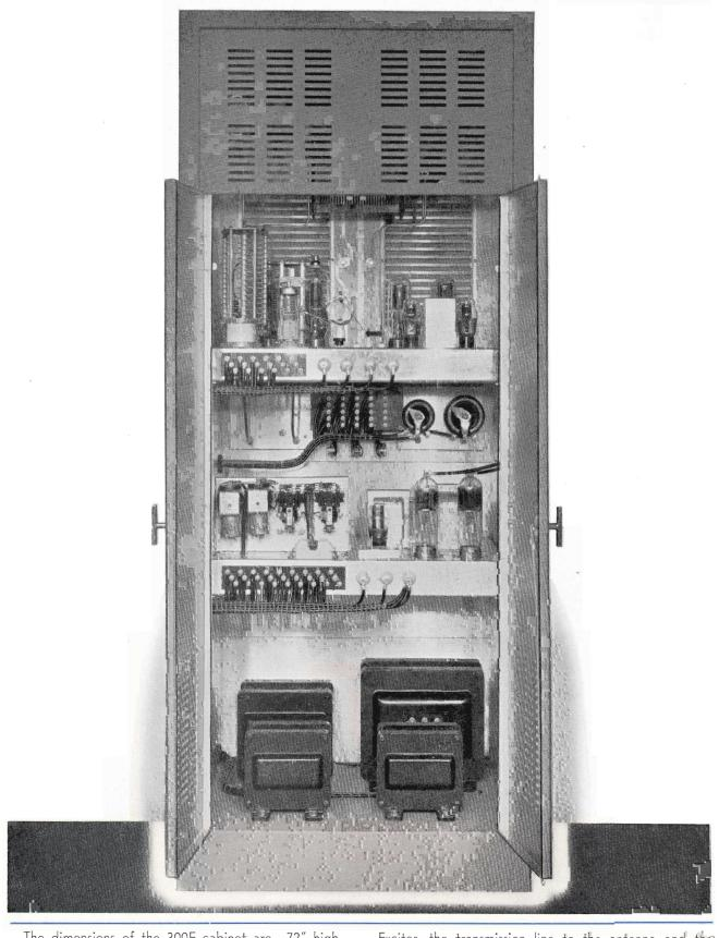
The dimensions of the 300F cabinet are—72" high, 30" wide and 24" deep. The sides of the cabinet are removable and expose the internal cabling and provide space for the incoming leads. Installation of the transmitter consists merely of connecting the power leads, the audio input leads, the transmission line to the 40C
