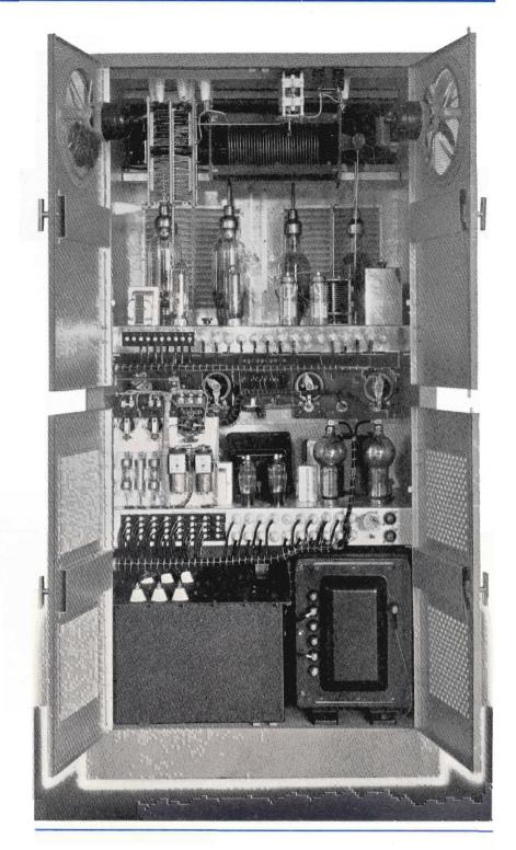
power interlocks as a safety measure, and the upper rear doors carry the blowers which assure proper ventilation.
