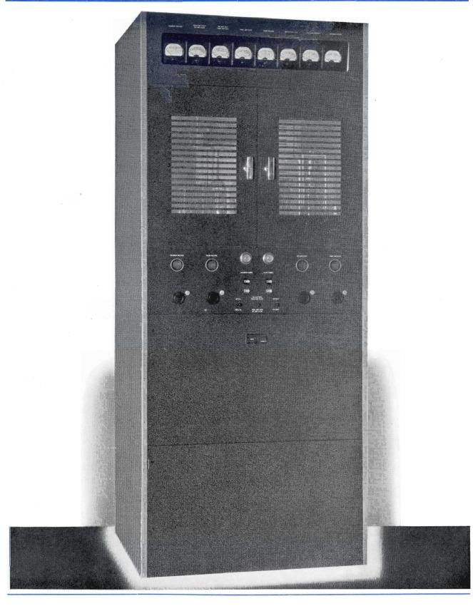
Communications Commission. The frequency response is uniform within plus or minus I db. from 30 to 10,000 c.p.s. and the total r.m.s. harmonic content is less than 5% of the fundamental at any percentage of modulation. Carrier noise is more than 55 db. (approximately 70 db. weighted value) below 85% modulation. The out-
