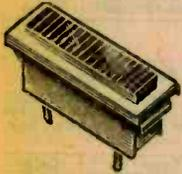
Rectangular neon indicator lights—excellent for new equipment design or for modernizing existing equipment. White nylon housing with chromed bezel. Have 6" insulated leads. Require 1.281-.395" mtg. hole. Built-in series resistor. Rated 1/2 watt at 125-250 volts. Size, 1 1/4 x 1 3/8 x 1 1/2". Shpg. wt., 5 oz.
