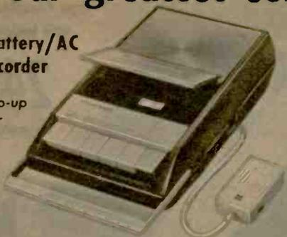
Model RQ-2095. Versatile recorder features pushbutton controls with pop-up cassette ejection for fast loading and removal of cassettes. Fast forward and rewind. Plays on 4 "C" batteries or 117 VAC. Automatic level control prevents distortion on voice recordings. Response, 80-8000 Hz. Built-in speaker. Mike and aux. inputs. Monitor output. With remote start-stop mike, pre-recorded cassette, earphone, batteries.  $2\frac{3}{4} \times 5\frac{1}{2} \times 10\frac{1}{4}$ ". Japan.
