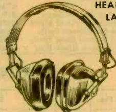
AP-5. Lightweight headset for prolonged use in language labs and for communications. Vinyl-covered ear cushions. Frequency response: 80-12,000 Hz. Factory connected for hi-impedance 600-ohm output. Leads may be changed to 4-16 ohms. Supplied with 7' 4-conductor cord, 1/4" phone plug. Shpg. wt., 3 lbs. 17 A 6302.....24.95
