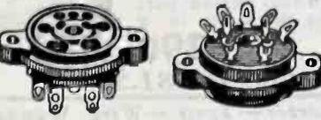
Its placement of 9 holes permits all types of tubes to be tested or used in this one socket. The filament holes are common to all types; the cathode, plate, grid and suppressor holes are individual for each type. Can be mounted in a 1 1/4 in. diameter cut-out socket hole. Can be mounted above or below panel! Solid bakelite moulded—vari-colored identification feature incorporated. **35c**
