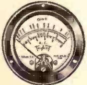
Scale reads: 0-1500 ohms; 0-1.5 megohms; 15-150-750 volts A.C., D.C., 1000 ohms per volt; D.C. 15-150 Ma. The copper-oxide unit with a D.P.D.T. toggle switch for A.C. and D.C. is housed with shunts for the 0.4 milliammeter in a separate case.
