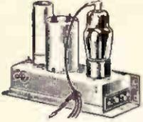
This unit is a small broadcast band oscillator. It may be used with any standard receiver. Solves most difficult problems in phonograph modernization work. No chassis wiring changes are necessary. All parts mounted on a radium plated metal chassis. Shpg. Wt. 6 lbs.
