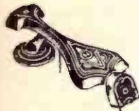
Used in Models R-80, RE-17, RE-57, RAE-68 and T-5 Electrola. Assembly comprises Head No. 7085; Arm No. 8643 with stop rod and connecting cable. Impedance of head 20 ohms. Fine response. Finished in dull silver. Shpg. Wt. 7 lbs.
