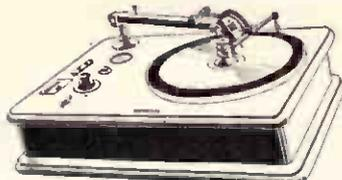
For up to 12-inch recording on Universal blank aluminum discs. Powerful motor. Weighted turntable, two speeds—33 $\frac{1}{2}$  and 78 R.P.M. rubber mounted. Fitted with volume indicator, volume control, off-and-on switch. Cuts 80 lines per inch. Fitted with
