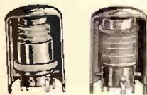
Wound on a 1" diam. by 2 1/4" long coil-form. The proper relation between the shield and coil insures the minimum of loss. Can size is 1 1/2" diam. by 2 1/4" high with 1 3/4" mtg. centers, utilizing two 6/32 spade bolts. Shield can be soldered to the chassis.
