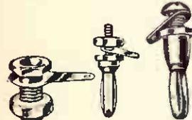
For use with all types of transmitting equipment. All milled of solid brass, nickel plated and furnished with lugs. Plugs have alloy contact springs secured over a pin, making them non-collapsible. Giant plugs and jacks have capacity of 25 amps, others 8 amps. The construction of these jacks and plugs insure perfect electrical contact, and consequently makes them also ideal for use with test equipment.
