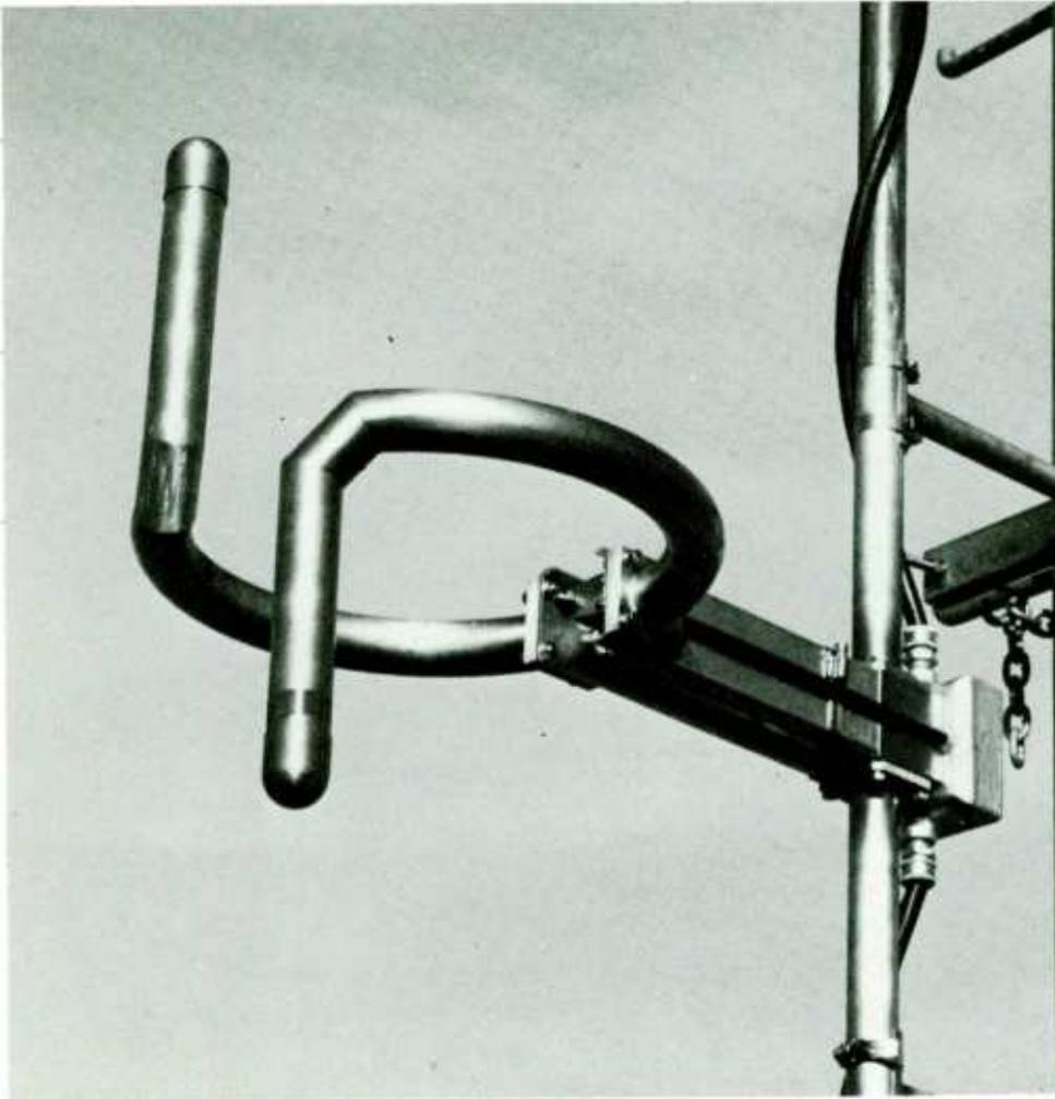
The rings of the antenna are mounted on 1-5/8" line and are end fed. A 6 ft. matching transformer extends below the lower bay and terminates in a 1-5/8" EIA, 50 ohm flange.
