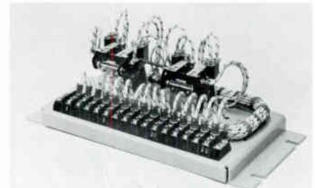
**TYPE 31123-B, MOMENTARY OUTPUT RELAY UNIT.** Connects between TRC-T unit and transmitter for control of circuits locally controlled by push-buttons, such as pattern change, and existing motors. Two sets DPDT contracts rated 15a, 115 vac, non-inductive.
