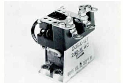
DOSX-7T: 115 vac coil, DPDT 15 amp, 115 vac non-inductive contacts. DOSX-12T: same as DOSX-7, except with 230 vac coil. DOSX-59T: same as DOSX-7, but has 110 vdc coil.
