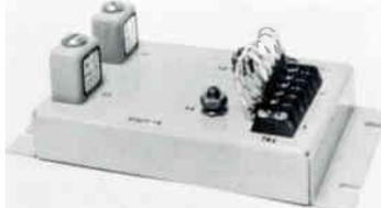
**TYPE 31129-B, LINE VOLTAGE METERING UNIT.** To be used if hum and noise exist in telephone lines from either side to ground.
