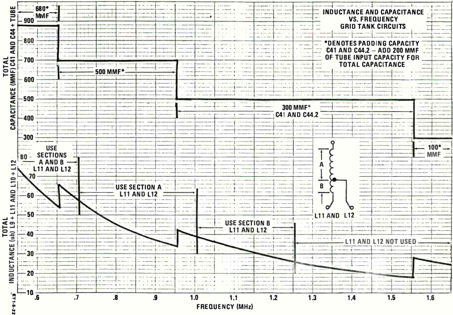
Figure 5-22. Grid Tank Circuits - Alignment Chart
