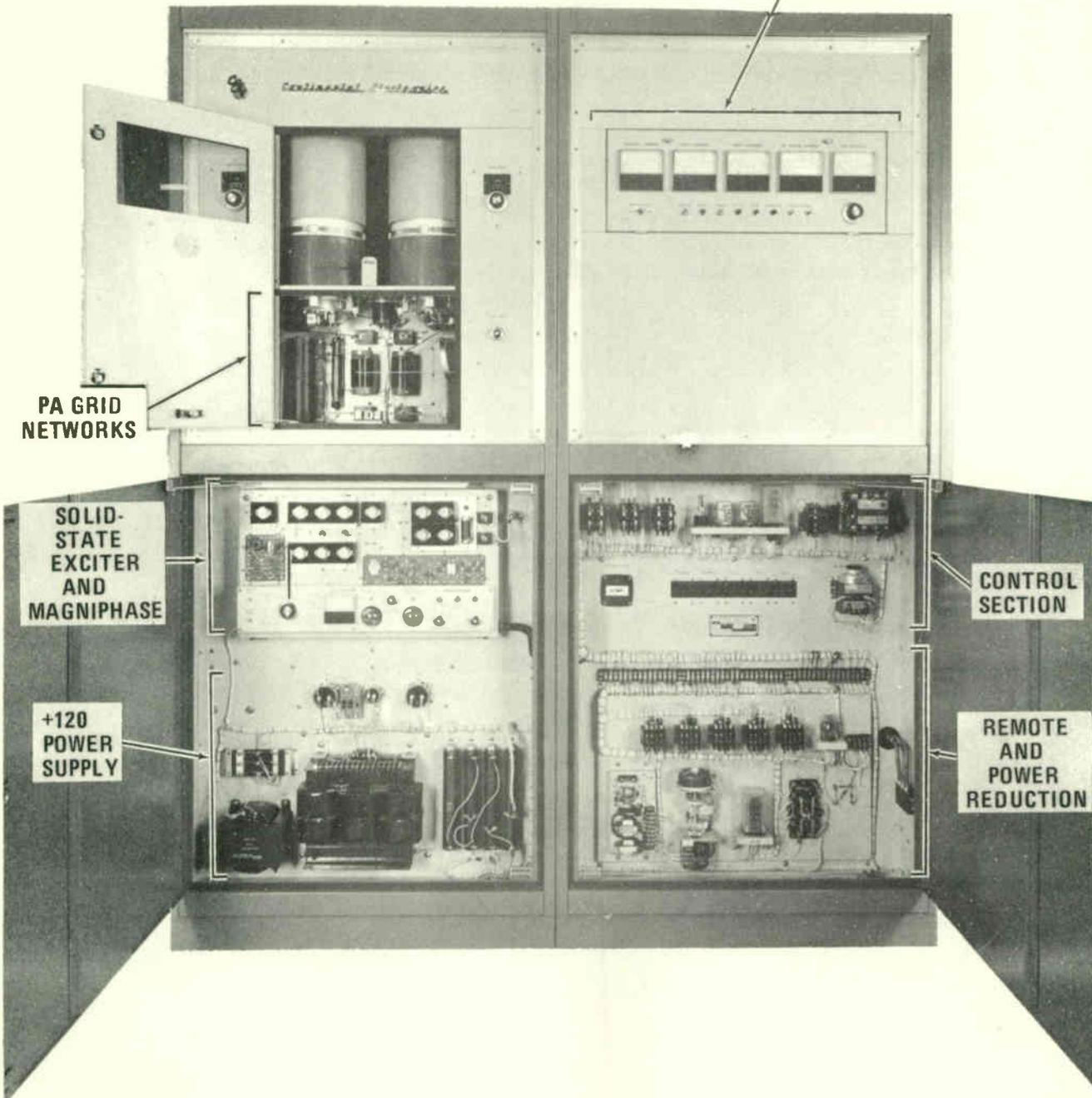
Figure 5-1. Transmitter Overall Front View, Showing Major Sections, Doors Open
