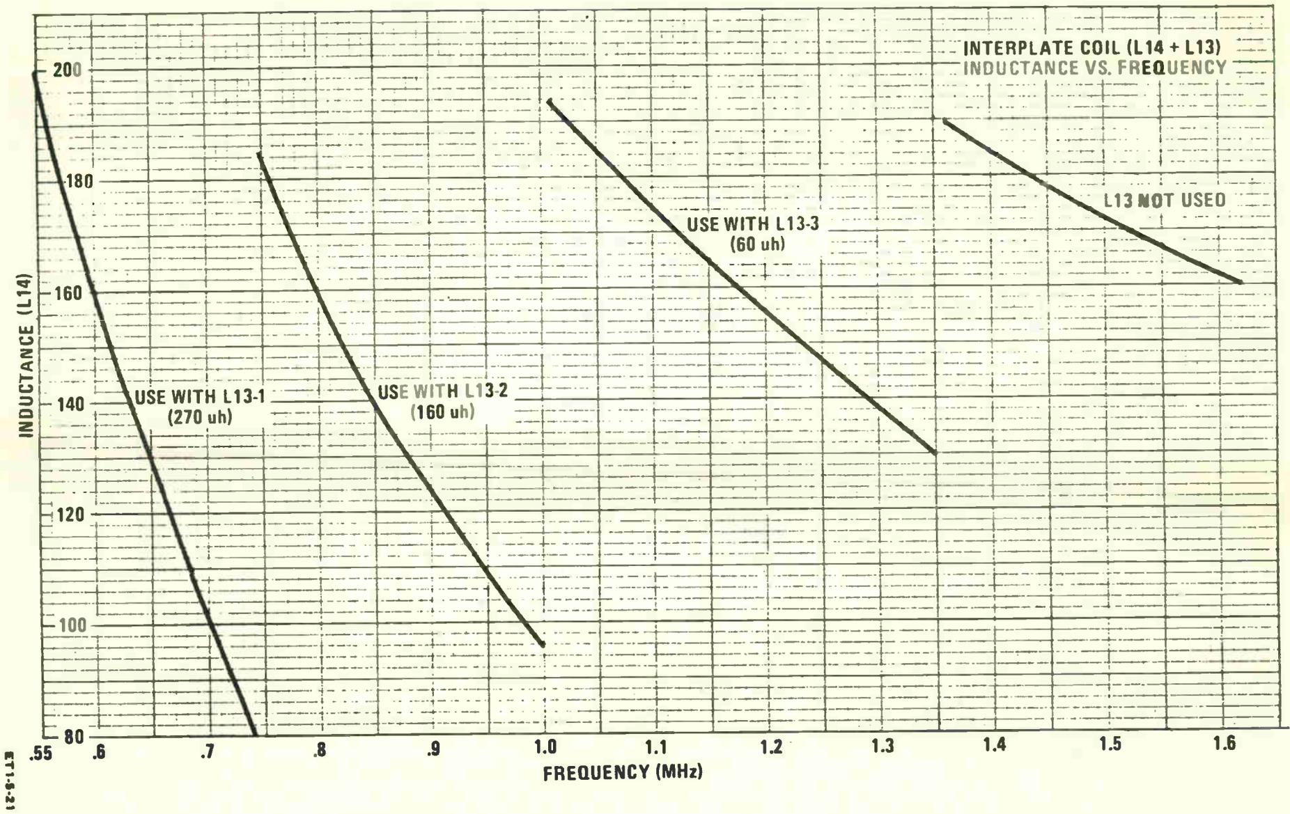
Figure 5-21. Interplate Coil (L14 and L13) – Alignment Chart
