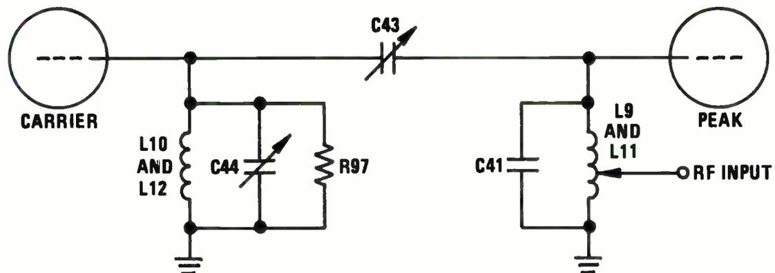
The simplified circuit doesn't show the bias connections which are series fed at the low voltage ends of the grid tank coils as shown in the complete schematic drawing.
