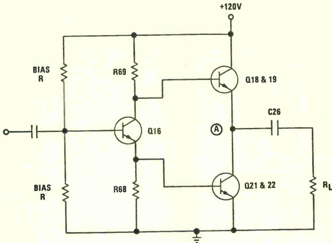
Figure 4-2. Modulator and 2nd Amplifier, Simplified Schematic
