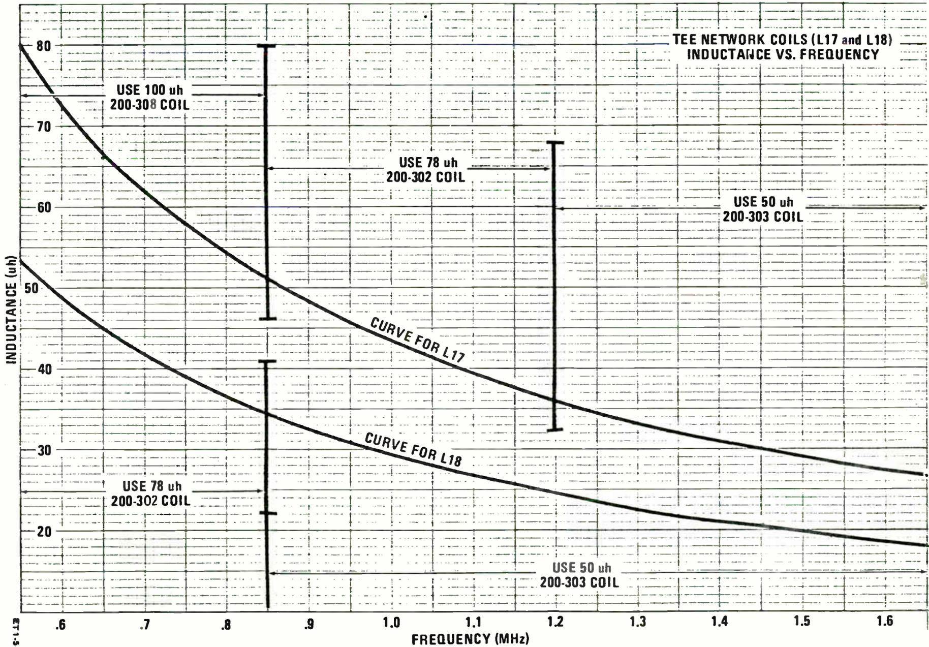
Figure 5-16. Tee Network Coils (L17 and L18) – Alignment Chart
