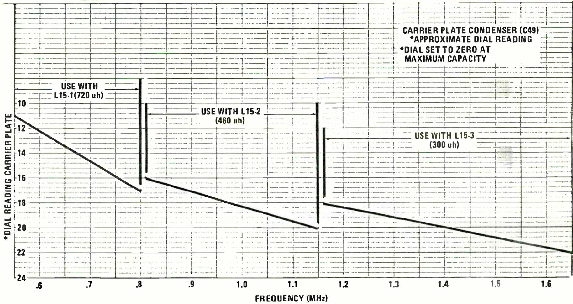
Figure 5-20. Carrier Plate Condenser (C49) – Alignment Chart
