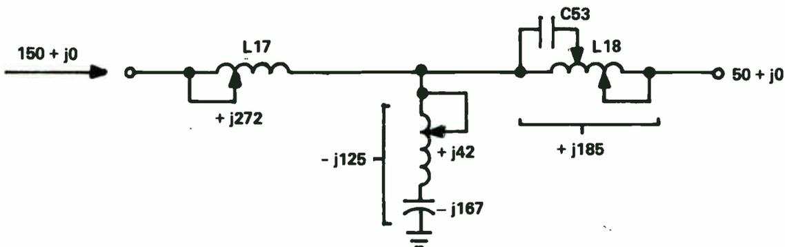
Typical reading for 50 ohm load.
