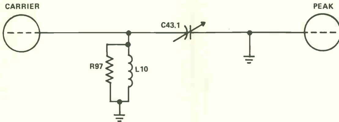
5. Remove the short from the peak tube grid and connect a 1000 ohm non-inductive resistor (a small composition resistor is suitable) from peak tube grid to ground.
