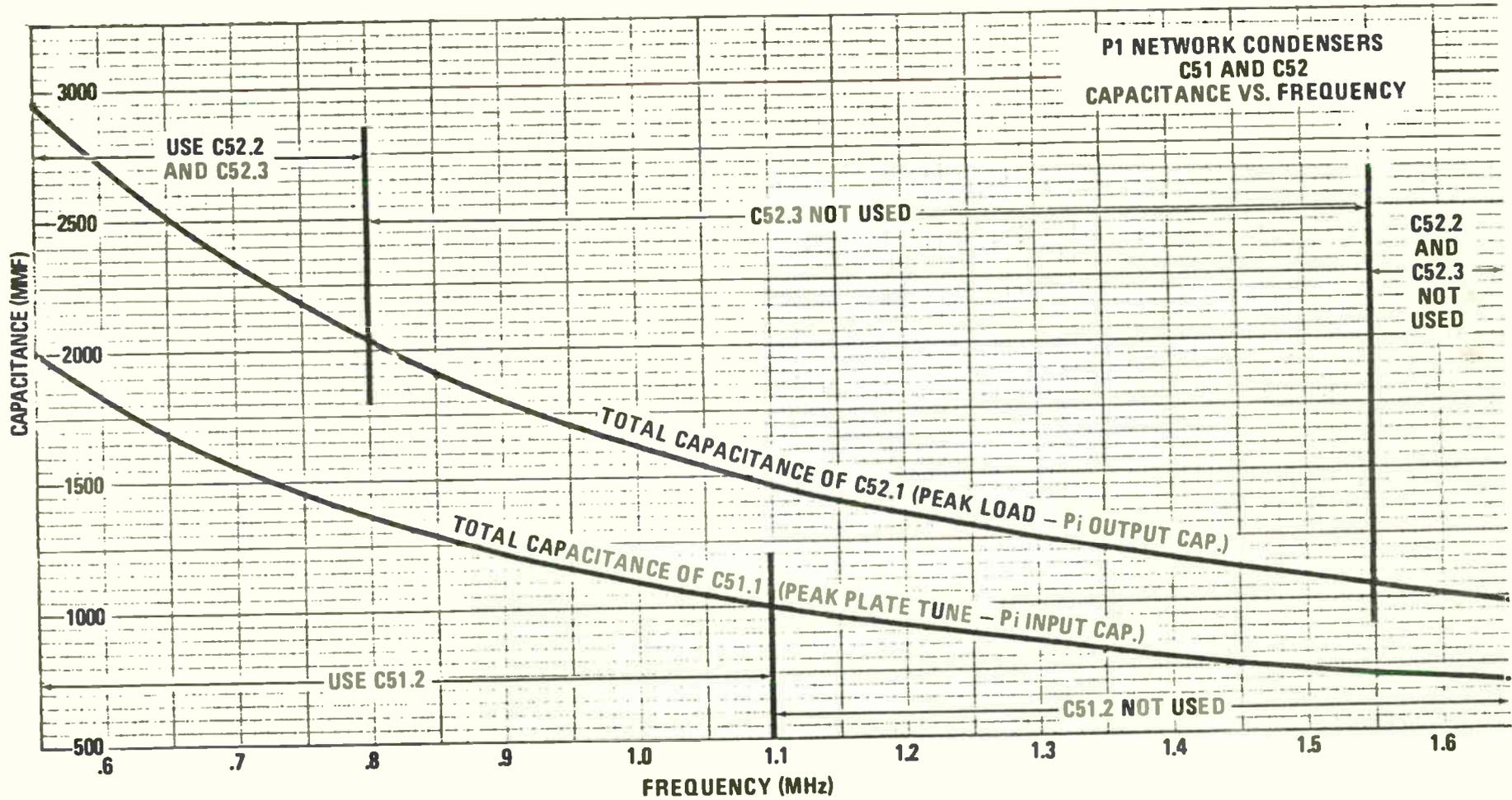
Figure 5-18. Pi Network Condensers (C51 and C52) – Alignment Chart
