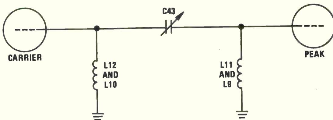
This is the basic 90° network. If capacitance is placed in parallel with the inductances, the network becomes:
