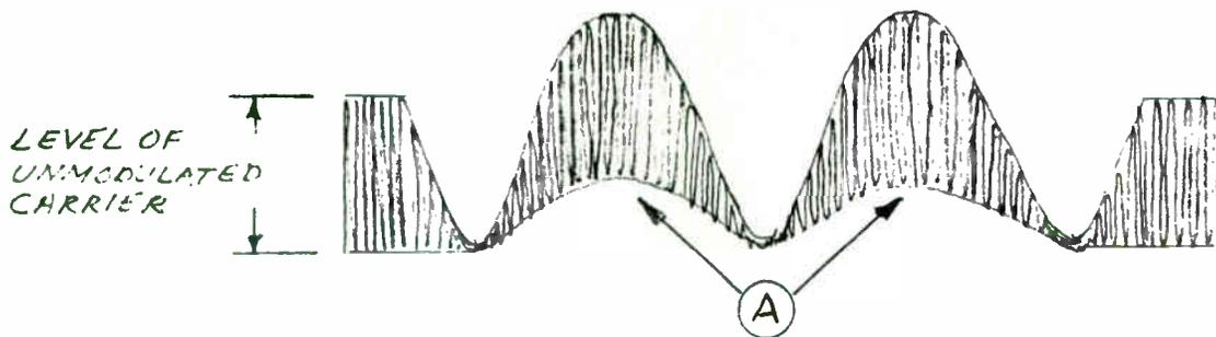
At point (A) in the modulation cycle, the transistors have insufficient base drive to maintain saturation at the time the DC collector voltage doubles its unmodulated value (100% modulation).
