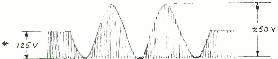
\* Level of unmodulated carrier.
