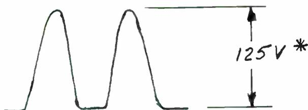
\* Limits are 2.5 to 3.5 times the collector DC supply voltage (position No. 5 on the test meter). For example, if the collector voltage is 40 VDC, the RF swing should be from 100 to 140 volts peak to peak. The flattened negative portion is the transistor "ON" time and should be from 30 to 50% of a full cycle.
