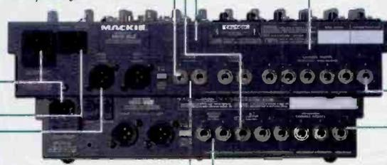
Control Room outputs feed monitor speakers without tying up the headphone jack.
