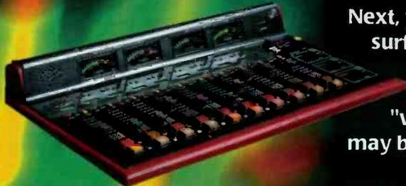
Next, you have your choice of several versatile console control surfaces. The ROC-10 (shown here) gives you ten fully assignable faders. Other choices include the modular Numix, with a range of 6 to 24 faders, the compact ROC-5 or our Vmix "virtual" PC-based control surface. Up to three control surfaces can be run from one Audio Engine.
