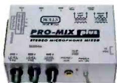
The PROMIX PLUS (MX545) mixes three microphones into one transformer balanced XLR output. It has three XLR inputs, each with individually switchable phantom power, low cut switches and level control. A 1/4" aux/headphone output has been provided along with a clip indicator, power indicator and power switch, and the unit is powered by two 9-Volt alkaline batteries.
