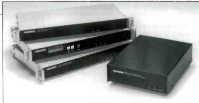
The Comrex MusicLine digital audio compression devices use ISO/MPEG Layer II audio coding, which allows transmission of full bandwidth stereo audio, 15kHz or more, along digital transmission paths of 112kbps or more. This lets a broadcaster, recording studio, or music service transmit high quality stereo audio using a Basic Rate ISDN phone line or a pair of Switched 56 lines, or mono (10kHz) audio on a single SW56 or 64kbps link. Compare to the cost of running traditional equalized phone lines!
