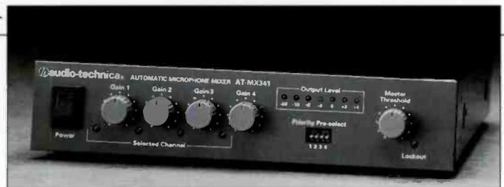
Need hands-off audio? Here's a programmable automatic mic mixer with four channels. The priority pre-select feature is ideal for moderator- or chairman-over-ride. It lets you set the mixer one of three ways: With all DIP switches down, the SmartMixer only allows the first voice to pass, overriding the other channels until the speaker is done. With one or more switches up, those voices can cut in at any time over the other channels. With all switches up, all mics are given equal priority.
