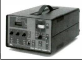
Three deviations (5, 10, and 25kHz) are internally selectable, depending on the frequency in use. Full output power is 25 watts, but two lower ranges are selectable for battery conservation.
