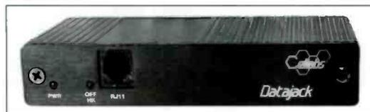
Cellabs' Datajack lets you do all of these. A standard RJ-11C telephone jack means compatibility with all standard fax machines and modems. A cellular phone adapter cable, available for most cellular phones, is required at extra cost.
