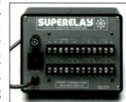
Superrelay can be controlled by any external momentary or maintained switch, or by CMOS/TTL. It provides six double pole relays used for low-voltage and audio switching, and a switched AC output will directly power up to 300 watts of warning lights (without buzz, pops, or arcs) and make them flash using the built-in, defeatable flasher. Superrelay can also be connected to any dial-up telephone line for control of equipment when the line rings. Keep an extra one handy for those emergency jobs.
