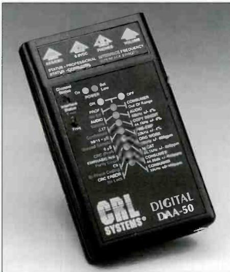
The DAA-50 can identify the digital signal format from any source (including AES/EBU, IEC958, S/PDIF, and EIAJCP-340), and give the user information like frequency, pro/consumer mode, emphasis status, and more. Is the source material copyright inhibited? The DAA-50 will tell you. The analyzer is hand-held, powered by two "AA" alkaline or Ni-Cad cells, and easy to use. Accepts balanced and unbalanced inputs. Belt clip and AC adapter included.
