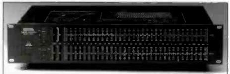
The Q2031A is a sophisticated stereo 1/3 octave graphic equalizer. In only two rack spaces, Yamaha puts 31 filters on two channels, each of which also has a sweepable 12dB per octave high pass filter, a 6dB or 12dB cut/boost range switch, a filter bypass, a peak indicator, and channel gain control. Inputs and outputs are both balanced (XLR) and unbalanced (1/4" TS), and the Q2031A operates from -20dBV to +4dBm. Sockets for output transformers are included on the rear panel.
