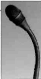
The subcardioid pickup pattern of this quality talkback microphone reduces pickup of unwanted noise. The gooseneck allows easy positioning. Response is 200Hz to 5kHz. A low-Z XLR male connector on the base of the gooseneck plugs directly into your console.
