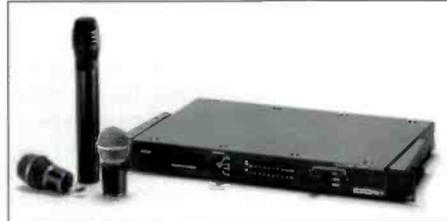
Pos-i-Phase true diversity circuitry operates over long distances reliably. The noise type squelch circuit maintains overall system quieting. The receiver is a half rack space wide, one space high, and includes a balanced mic-level output with attenuation control. Each hand-held or belt-pack transmitter has silent ON switch, audio mute, and low battery indicator. Frequency response is 50-15kHz  $\pm$ 1dB, with S/N of 110dB. All are covered by the Telex three-year warranty.
