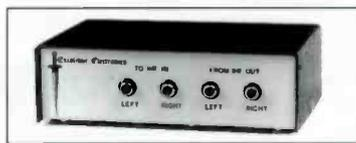
Don't let level and impedance mismatches keep you from connecting good, affordable consumer equipment to your pro gear. This is a compact two-way, stereo unit with adjustable I/O levels. Frequency response is  $\pm 0.2$ dB, DC to 25kHz; THD <0.006%; noise >90dB below operating level; and >75dB common mode rejection on the balanced input stages. Barrier strips provide gas-tight connections on the balanced inputs and outputs, with RCA phono jacks on the unbalanced I/O.
