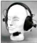
Circumaural, air filled, double layered cushions provide isolation and comfort. The microphone's pattern is tailored so that it provides the best response when offset to the side of the mouth. The HMD 224 weighs under one pound.
