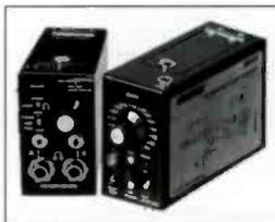
The FP11 battery operated mic-to-line amplifier provides gain of up to 84dB, adjustable in 6dB steps. The unit has both a balanced XLR mic level input and a 1/8" TS mini input for a high level, high impedance source. The output is transformer balanced and appears on both an XLR connector and a set of spring contact binding posts. A smooth, switchable peak limiter and belt clip are included in this rugged, dependable unit. Powered by a single 9V battery.
