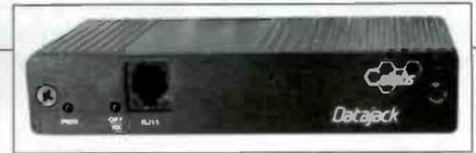
The Cellabs Datajack gives you the power to send a fax or plug your laptop computer's modem into your cellular phone. A standard RJ-11C telephone jack means compatibility with all standard fax machines and modems. A cellular phone adapter cable, available for most cellular phones, is required at extra cost.
