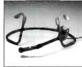
The hypercardioid condenser mic takes 12-28V phantom power and provides 20-20kHz response, 200 ohms, with preamp/XLR connector. The headphones check in at 30-18kHz, 200 ohms, with 1/4" stereo plug. A ten foot cable and windscreen are provided.
