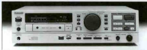
The Panasonic SV-3700 is built on a massive die-cast chassis that ensures stability and reliability. Important features include: shuttle wheel, high performance one-bit A/D conversion, high resolution 4-DAC system, and 4-digit error rate display. The analog inputs/outputs are balanced XLR's, digital ins and outs are AES/EBU Professional Format and IEC 958 SPDIF. The SV-3700 comes with an infrared remote control and 3U rack kit.
