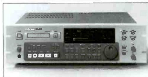
The Tascam DA-60 DAT recorder features 4 heads for confidence monitoring; a 2 second RAM buffer for instant start; accurate dial search capability, auto cue, auto punch in/out with rehearsal capability; gapless punch in and out,  $\pm 12.5\%$  pitch control on playback; two locate points; absolute time, start, end and program numbers which can be recorded independently in the sub-code area; user-selectable
