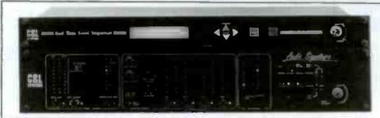
The CRL Real-Time Event Sequencer is a time-based external controller used to automate, or "daypart" the CRL Audio Signature processor. The Event sequencer stores up to 200 events occurring over a seven day clock. The unit can also
