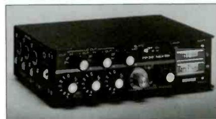
Shure FP32A is a stereo version of the FP31 audio mixer, with a center-detented stereo pan pot for each input channel, plus a concentric clutched stereo master gain
