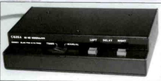
The Conex 25Hz tone generator has front panel LEDs to indicate the duration of the tone and silence intervals. The CG-25A has plug-in type terminal strips with 600  $\Omega$  balanced bridging inputs and can be remotely controlled.
