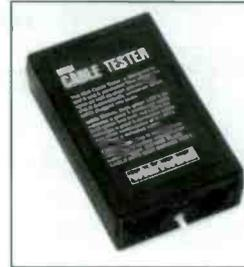
This Cable Tester can test cables with any combination of XLR, 1/4" or RCA phono plugs for shorts, opens and phase. The handsfree design allows manipulation of cable to locate intermittents. An on/off switch is provided, with LED to indicate sufficient testing power. Belt clip included.
