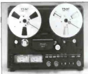
The Tascam 22-2 is a recorder for user's who don't require micro-processor control or large reel capabilities. It has front panel left and right 1/4" microphone jacks/controls and has a great deal in common with the more costly open reel machines.
