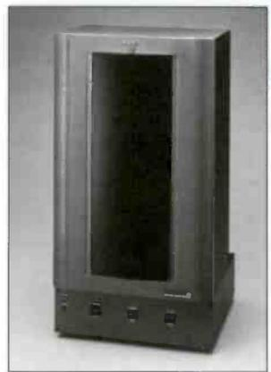
The Sony CDK-3600 CD Auto Disc Loader can handle the storage, loading and playback of up to 360 compact discs. An external computer provided by the user is connected through the RS-232C or RS-422A interface for automated playback and overall control. In addition to quick access and smooth loading, the CDK-3600 incorporates built-in dual players to ensure
