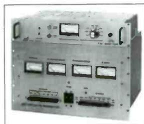
The QEI 675T Series are tunable PLL FM transmitters using 100% solid-state technology with an adjustable RF output. They meet all requirements of the FCC for educational or commercial mono, stereo and SCA applications. They are remote control/ATS compatible; fully protected against high VSWR; have convenient push-button operation; and can be housed in a desk top height cabinet. Prices include a spare parts kit and 675 Exciter.
