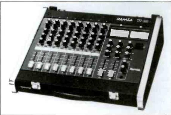
The Ramsa WR-133 compact, 8x2 channel portable mixer comes with a carrying handle and detachable hard cover making it perfect for taking on the road. It comes complete with balanced mic/line and phono inputs, effect, monitor, and mono outputs, and balanced stereo XLR outputs.
