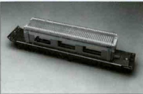
Gentner EasyTerm/FB-1 is a 2U punch-down wire termination panel with a snap-on bracket and a dust cover. Wires are routed from inside the rack. Its hinged panel allows you to swing the termination out of the way to access your equipment and cable. It is a stranded wire punch block that offers high density and reliability with simple connections. 320 terminals are provided with 2 connection points per terminal; each connection point accepts 2 solid or stranded wires, 22 to 26 gauge.
