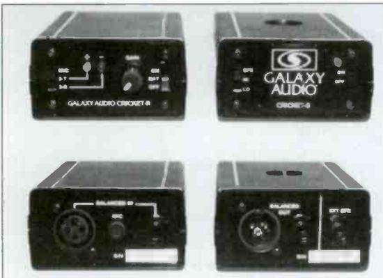
A test instrument, for the audio installer or soundman, which indicates absolute polarity of most audio devices or may be used as a cable tester. The send unit has balanced 1/4" and XLR jacks, an unbalanced 1/4" speaker out jack and an internal speaker. The receive unit has 1/4" and XLR jacks, a sensitivity control, and an internal microphone. Both units are housed in high impact padded ABS case and are powered by a 9 volt battery.
