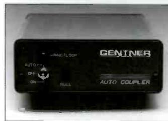
The Gentner Auto Coupler can send or receive line level audio sources. It will automatically answer after one complete ring and disconnects when the caller hangs up. Use the Auto Coupler for information lines, IFB, or any use requiring automatic operation.
