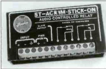
Radio Design Labs ST-ACR1M audio controlled relay is designed to switch on low-level sources, such as microphones or mic-level sources. The ST-ACR2 is designed to switch on line-level sources with extended release delay. The ST-ACR2 is widely used as a Silence Sense Relay.
