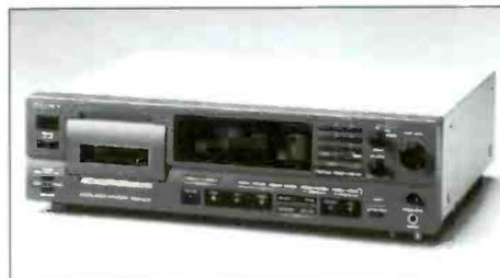
The Sony PCM-2300 professional digital audio tape recorder /player has balanced analog and coaxial digital IEC-958 ins and outs, long play mode, auto fader, margin display, records absolute time, supports three sampling frequencies, and is supplied with a wired/wireless remote and rack mount adapters. In the long play mode it can hold up to four hours of 12 bit non-linear 32kHz audio.
