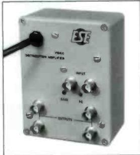
The ESE 207 and 208 compact video distribution amplifiers are portable and easy to install. Controls are easily accessible for video gain, DC level and HF equalization. The amplifiers are clamped to provide a consistently stable output signal to the output terminals. A single pair of BNC connectors are wired for a loop-thru input with provisions for a terminating resistor if desired.
