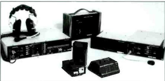
The Telex Audiocom is a headset intercom system consisting of modular components that can be connected with conventional wiring to form a simple party line communication system or a more sophisticated network using "director controlled" multi-channel configurations.
