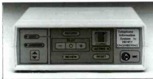
The Henry Telephone Information System (TIS) can store up to 10 separate messages in its digital memory. When the unit is called, a "Menu" message plays, telling the caller which messages are available. The caller may then select any message(s) for instant playback by simply pressing the buttons on a Touch-Tone® telephone. Messages are easily updated by re-recording
