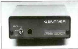
Gentner's Hybrid Coupler connects directly to the telephone line and is used to send or receive audio or other information. Its passive design allows you to "tap" the phone line, using the telephone and coupler simultaneously, or it can seize the line. Use it for news or producer feeds, or sending a church service broadcasts.
