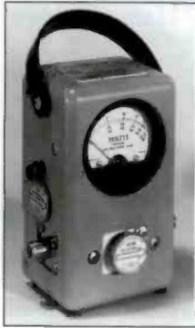
The Bird Model 43 thru-line directional wattmeter accurately measures forward or reflected power in coaxial transmission lines under any load condition. This wattmeter consists of a line section and meter housed in an aluminum case. Quick-change-type connectors and plug-in elements are required for operation.
