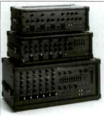
Toa MX-401 is a compact, 4-channel self-powered mixer with 150 watts into 4 ohms. Each input channel has its own level control, a two-band equalizer, pre-EQ and post-EQ sends, and balanced/unbalanced inputs. One program and one foldback output are provided. The master control section features a patchable 5-band graphic equalizer, a 3-spring reverb, a full patch bay with phone and tape inputs. Power amp protection circuitry and Auto Comp compression, both include LED status indicators.
