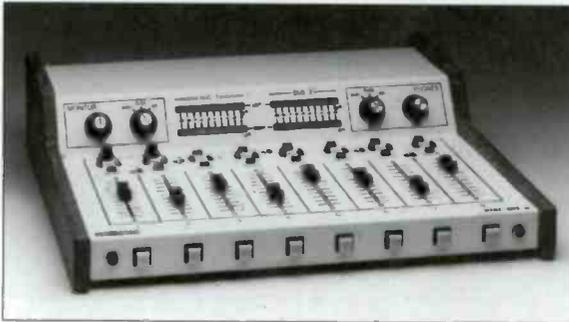
Autogram's MiniMix 8 professional audio console features: • Aluminum case w/oak endbells • 2 stereo output buses • mono output • 8 slide plug-in pots • 2 dedicated mic slide pots • 12 stereo inputs • 6 unbalanced stereo for CD/cassette/tape/etc. • 6 high level balanced pro-stereo inputs • all VCA operated • cue amplifier/speaker • made in the USA.
