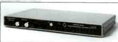
The PB2X8 provides two XLR inputs which can be individually switched or mixed into any of eight isolated line level outputs. Each input may be individually switched for microphone or line levels with phantom power and low cut filters available for the microphone inputs. A calibrated test tone oscillator can be switched
