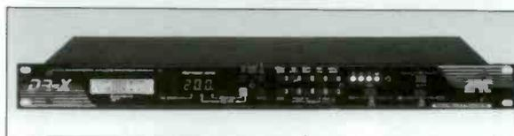
The Art DRX-2100SE will perform 10 simultaneous audio functions; features 24 bit DSP; is a full function dynamics processor with compressing, limiting, programmable EQ, noise gate and expander; studio reverberator; and multi-effector. It gives you over 2 1/2 octaves of pitch shift, 12 reverb programs, 12 reverse and gated algorithms, over 20 types of delays, stereo panning, and complete MIDI Interface.
