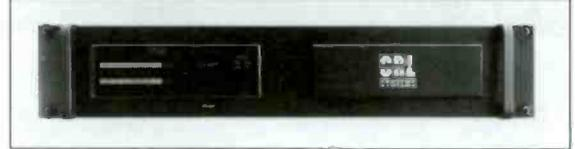
Designed for Stereo-TV, the CRL TVS-3001 is a two-channel tri-band AGC having a capability of up to 30 dB of gain reduction. Integral Fh filters are also included as is an exclusive CRL/CBS loudness controller that "tames" loudness problems. The TVS-3001 also senses and corrects phase reversal problems on program material. The TVS-3001 is placed at the studio and prevents audio overload of the STL/telco feeds.
