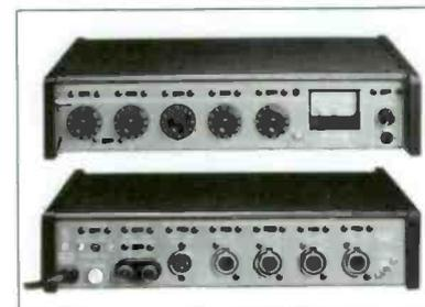
Shure's M267 features include: a switchable limiter, phantom power, LED peak indicator, headphone jack with level control, automatic muting circuit, battery check function, tone oscillator, mic line switches on each input and output, low-cut switches on each of four transformer-balanced inputs, and is powered by three standard 9-V batteries or AC.
