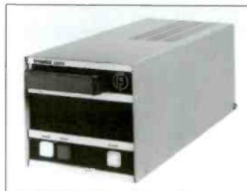
The Fidelipac ESD10 achieves an erase depth of 75dB, or more. It uses dual, high quality erase heads, a patented splice find system and requires no sensitivity adjustments.
