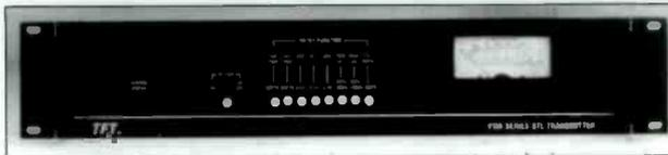
The TFT 8300 is designed for the major market's RF signal environment where it becomes increasingly difficult to operate composite STL's due to spectrum congestion. It has components such as S.A.W. filters, low noise RF front end, variable bandwidth IF amplifiers and cast aluminum RF shielded housings for critical circuits.
