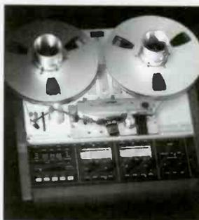
The Studer A807 was conceived as a multipurpose tool for recording studios and broadcasters. The A807 has a highly perfected tape transport design with advanced drive technology features: two rugged, direct drive AC spooling motors, brushless DC capstan motor, comprehensive function selection and digitally controlled analog technology.
