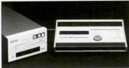
The Tascam CD-701 has a full size disc turntable with a vibration free rigid disc clamp. This presents the pickup with a non-vibrating surface, to help eliminate tracking errors. In
