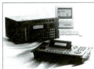
The Akai DD1000 is a "virtual" four track digital editing system with the capability to record two tracks while playing two tracks and simultaneously play four tracks. The removable two-sided MO disk has 325 megabytes of storage per side which equates to 30 minutes stereo per side at 44.1KHz. You get the convenience of instant access and full non-destructive editing, with no need to run back-up and restore routines. The medium is easy to
