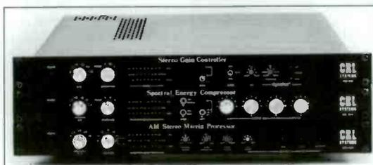
The CRL SGC-800 is a stereo AGC/compressor which is used before an STL or telco lines to eliminate system overloading. The AGC can be operated as "dual-band, wideband or both" and allows for up to 30 db of gain reduction. Dynafex® noise reduction is also included.
