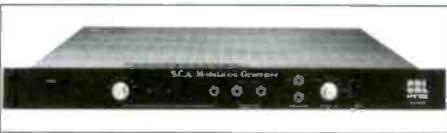
The CRL SCA-300B is a digitally synthesized subcarrier generator with integral two-band audio limiter. The SCA-300B subcarrier frequency is user-selectable from 40 to 110 kHz. Either voice or data can be transmitted; two direct data input ports are provided. Also, the SCA-300B can be fully remote-controlled.
