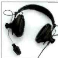
The Sennheiser HMD 224 has a closed headphone with 16-20,000 Hz response and a supercardioid dynamic mic with 50-12,000 Hz response. Sealed ear cushions and directional mic reduces surrounding noise. Serviceability is assured by easy disassembly of all components. The cable ends in pigtails to permit stereo or dual mono connection. Weight 26 oz.
