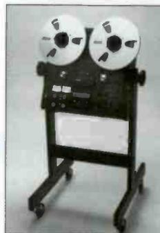
The Otari MX-50IIN is an affordable audio recorder. It has a built-in 5-digit tape timer displays, search to cue locator with one cue point memory, zero locate,  $\pm 7\%$  vari-speed, and transformerless active balanced XLR inputs and outputs. An independent reel size selector switch allows supply and take-up reel sizes to be intermixed.
