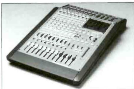
The Tascam M1500 series recording mixers are designed for 4 and 8 track studios. They feature: balanced XLR mic and 1/4" line inputs for each channel • top access connector panel for easy patching • 3-band mid-sweep EQ on each channel • 3 aux sends with independent send controls • 2 stereo and 2 mono assignable effects returns • insert and direct out patch points on channel 1 - 8 • bargraph meters for group and monitor outputs • and PFL facility.
