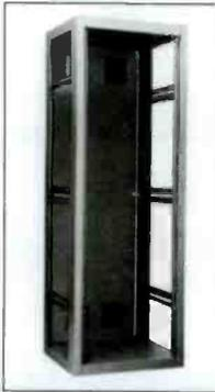
House of Metal Enclosures, HOME makes a comprehensive range of cabinets, enclosures, racks and consoles. Panel mounting hardware is supplied. The WRE Series is 18 1/2" deep, 22 3/8" wide and comes with fixed 11ga rack rails drilled and tapped for 10/32" screws in the standard grey hammertone unless specified. A rear door with lock is included.
