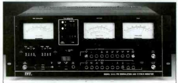
The TFT 884 is a cost effective alternative to the 844A. All proof measurements can be made along with incidental and residual synchronous and asynchronous AM noise. It includes a convenient front panel test output. The 884 has a one year manufacturer's warranty.
