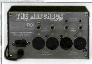
The Henry Matchbox interconnects consumer equipment with professional studio gear. It is a bi-directional unit, with four independent amplifiers providing full stereo input and output interface. The gain is adjustable to accommodate either +4 or +8 system levels.
