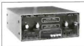
The ATI EM1000 Emph'a sizer has a program controlled input gate, a compressor/ limiter and a four band preset parametric equalizer all in one box. Use it as a DJ mic processor, on remotes, or for telephone
