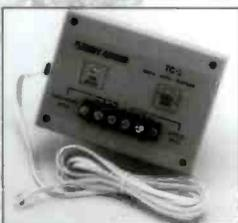
The Indy Audio TC-1 is an auto-answering phone coupler. It can feed audio down the line to the caller, take audio off the line for broadcast, or can be connected to a hybrid for bi-directional communications. The TC-1 is powered by the phone line, a front panel LED indicates when the unit is in use, and a dry relay closure is provided to start a cart deck and alert the control room operator, etc. A voltage reversal or temporary open circuit is required for auto disconnect
