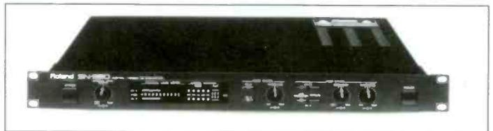
The SN-550 is a fully digital noise elimination system that employs exclusive DSP circuitry to remove all types of noise without "breathing" or changing the tonality of the overall sound. This is achieved with two separate noise reduction circuits that handle noise and hum independently. The SN-550's single-ended design can perform noise cancellation in real time, making it ideal for broadcasting, sound reinforcement and other professional applications.
