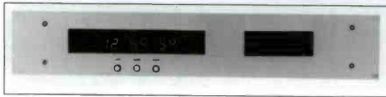
The ESE 750E Series of thumbwheel programmer/comparators is both economical and easy to use when programming 1 or 2 output events. A thumbwheel switch is set to compare the time information from an ESE clock or timer. Output occurs each time the switch setting agrees with the time display.
