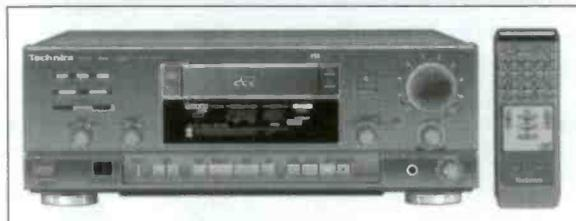
The Technics RS-DC10 auto-reverse digital compact cassette deck records on digital compact cassette (with SCMS) and plays on both analog and digital cassettes. Featuring 1-bit ADC/DAC, four dedicated PASC chips, and built-in Dolby™ B/C NR for analog tape playback compatibility. There's a 29-key wireless remote included.
