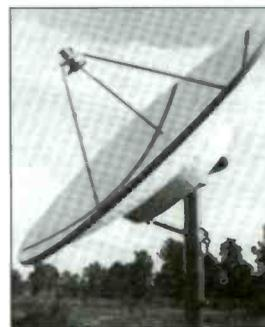
Comtech's 3.0 and 3.8 meter antennas keep installation costs down with a single pole mount and three-piece reflector design. The use of Comtech's unique splice-strap system yields a superior surface tolerance. The 3.8 meter has a gain of 42.9dB, ideal for SMATV, radio SCPC and Cable TV applications. The El/Az mount permits 360° azimuth adjustment without costly foundation alignment. The elevation jack provides smooth elevation adjustment from 0 to 70°. The polar-mounted system
