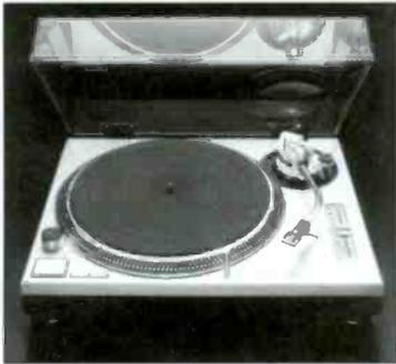
The Technics SL-1200MK2 is a quartz-locked direct drive turntable that is virtually feedback-proof because of its special base design. The platter is damped on both sides to avoid ringing. Its high starting torque brings the platter to rated speed within 0.7 second. Includes base, tonearm and dust cover. 33 1/3 and 45 RPM ± 8% pitch control.
