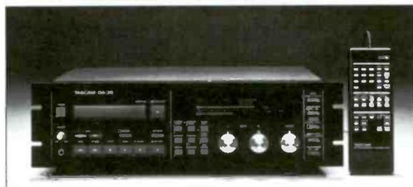
The Tascam DA-30 is ideal for professional digital mastering applications. The DA-30's analog inputs include balanced XLR and unbalanced RCA jacks. The analog outputs include variable balanced XLR, unbalanced RCA, and fixed RCA. Digital inputs and outputs are AES/EBU XLR and coaxial RCA. It comes supplied with a flexible wired remote control and a 15 pin parallel I/O port for external transport remote control.
