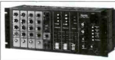
The Ramsa WR-M10A, multiple source mixer has four balanced XLR Mic/Line inputs and two stereo input channels. Each stereo channel accepts three pairs of line level signals, and one pair of RIAA-equalized phono inputs. Eight stereo and four mono sources can be connected to the WR-M10A. A built-in compressor can be switched to 'level' all mono inputs. There is priority muting for voice overs. Both stereo input faders are
