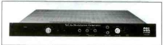
The CRL SCA-300B is a digitally synthesized subcarrier generator with integral two-band audio limiter. The SCA-300B subcarrier frequency is user-selectable from 40 to 110 kHz. Either voice or data can be transmitted; two direct data input ports are provided. Also, the SCA-300B can be fully remote-controlled.
