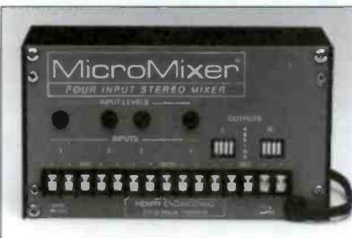
Henry's Micromixer will accept up to four balanced or unbalanced line-level inputs and will mix them to a stereo output. A level control for each input provides adjustment from "off" to +10dB of gain. "Micro-Assign" switching permits each input to be assigned to the left, right, or both outputs in any combination. All circuitry is active and direct coupled for exceptional sonic accuracy.
