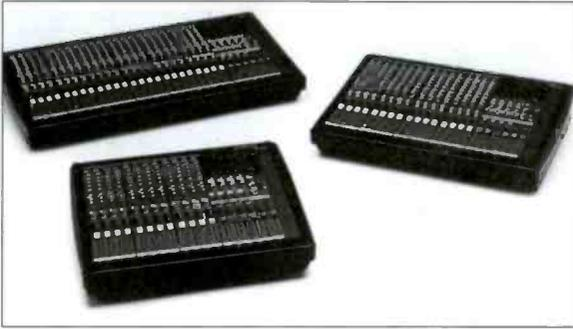
The Ramsa WR-S4400 Series consists of 12, 16 and 24 channel professional 4-Bus mixers with professional length faders, two selectable inputs per channel, individually switchable 48-volt phantom power, flexible 3-band EQ with sweepable midrange. This 4-Bus mixer has four "main groups" plus left and right stereo masters from channels or groups and four "aux sends."
