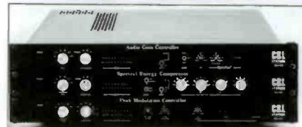
The CRL AGC-400 is a mono, gated, dual-band/wideband AGC providing up to 30 dB of gain reduction
