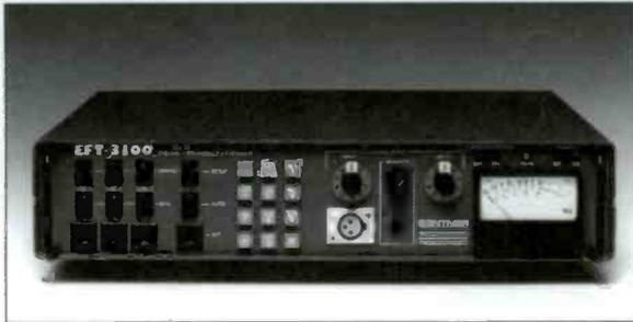
High quality audio on standard phone lines is possible with Gentner's EFT-3100. This DSP-based frequency extender uses three dial-up lines to deliver 50 Hz to 7.5 kHz audio. Auto-answer, auto-setup, built-in touch-tone pad, and automatic correction of differential line delay are just a few of its capabilities. The EFT-3100 may also be used as a two-line extender to provide 5 kHz audio.
