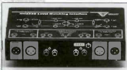
The Valley HH 2 x 2B Level Matching Interface resolves the level and impedance matching problems associated with interfacing -10dB equipment to the studio and broadcast equipment standards of +4dB and +8dB. It also ensures immunity from RF pick-up and hum due to electronic balancing of the +4/+8 inputs and outputs.
