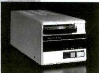
The Broadcast Electronic's Splice Trak 90 with its dual erase heads will erase any standard NAB cart to a typical erase depth of 90dB. Ignoring tape colorations which might fool an optical system, the splice finder senses the tape thickness at the splice.
