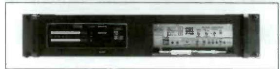
The CRL TVS-3003 is a MTS-stereo generator and audio limiter. The TVS-3003 also has a wideband AGC providing up to 20 dB of gain reduction. The stereo generator portion of the unit is digitally synthesized and therefore is drift free. Limiting is handled by a two stage "variable transfer function" limiter which smoothly handles peak transients without generating distortion products. A "stereo enhance" feature dramatically improves your viewer's received stereo effect.
