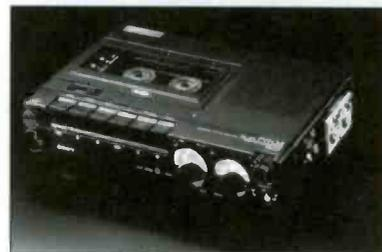
The Sony TC-D5PROII portable stereo cassette recorder features reliable mechanisms including disc-drive capstan, a servo tape transport with coreless motor, twin VU meters, LED peak level indicator, built-in monitor speaker,
