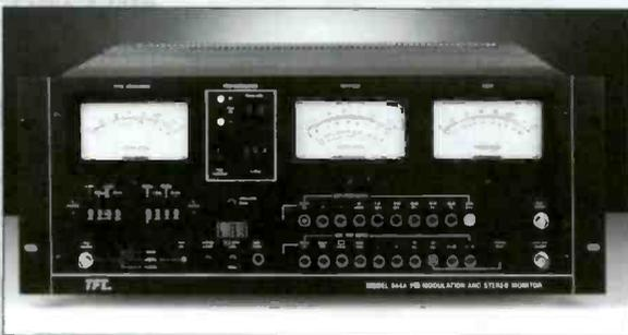
The TFT 844A is an FM stereo mod monitor that has a frequency agile RF pre-selector, baseband demodulator and stereo demodulator. The 844A can be used for off-air monitoring or direct transmitter proof measurements. This monitor can be used for complete measurements of total, right and left channel modulation, channel separation, main
