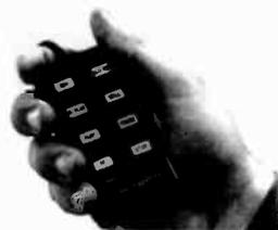
These functions are at your fingertips: ▪ Reverse while pressed, returns to play when released ▪ Reverse-Play while pressed, returns to play when released ▪ Slow-Motion ▪ Reverse-Slow-Motion ▪ Still Frame ▪ Reverse-Frame ▪ Fast View ▪ Play ▪ Rewind ▪ Stop ▪ On/Off ▪ Record/Record Pause ▪ Lighted buttons let you operate in dark offices and conference rooms ▪ 3-year warranty
