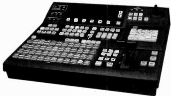
**DVS-8000C/1 Component/DVS-8000/1 Composite Digital Video Switchers**
