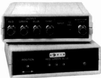
input selection: 1) horizontal and vertical sync, 2) composite sync or 3) sync on green input
