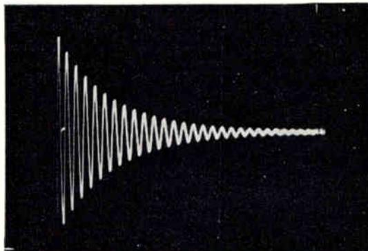
Figure 3-19. Waveform similar to that of Fig. 3-18. Increased accelerating potential of Type 304-H (3000 volts) rendered entire pattern visible
