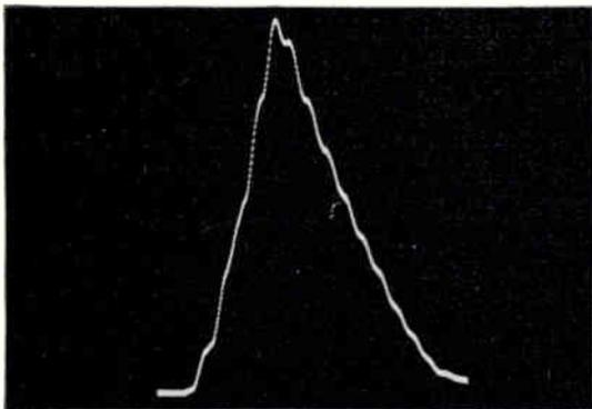
Figure 3-15. Indication of variation of volume of liquid in a retort. Signal, applied through d-c amplifier channel, was displayed on a 10-second sweep
