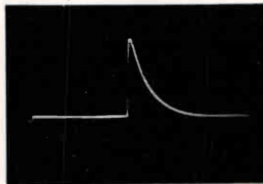
Figure 3-24. Observation of nerve potentials is an application requiring many features of the Types 304 and 304-H. Nerve potential below was recorded from Type 304
