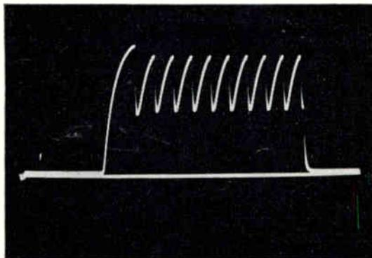
Figure 3-16. Voltage from oscillating neon bulb, applied through d-c amplifier channel. D-C voltages may be measured directly (base line represents zero volts)
