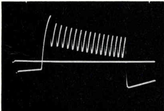
Figure 3-17. Waveform similar to that of Fig. 3-16, passed through a-c amplifier. Note tilt due to time constant of coupling circuit, and shift of reference axis
