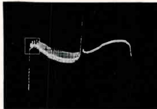
Figure 3-22. An oscillogram of the voltage field in the vicinity of a fluorescent lamp, displayed with no expansion of sweep. Compare with Fig. 3-23
