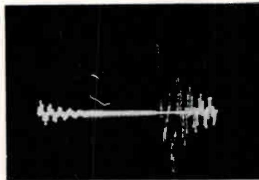
Figure 3-21. Vibration similar to that of Fig. 3-20, displayed on recurrent sweep. Phenomenon begins toward end of trace, with much of the signal lost entirely
