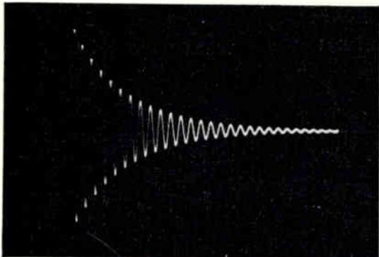
Figure 3-18. Relatively-high-speed transient in form of damped oscillation. With accelerating potential of 1780 volts, high-speed portion of trace was not recorded
