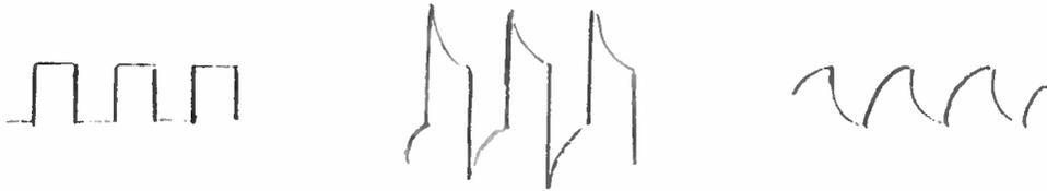
FIGURE 4-4 - WAVEFORMS ENCOUNTERED IN ADJUSTING THE Y ATTENUATOR
