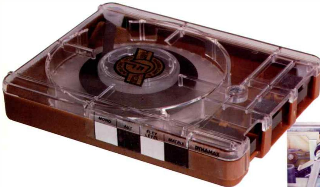
The DYNAMAX CARTSCAN System allows cartridges recorded at elevated level, mono and matrix stereo to be intermixed with carts recorded in standard level and discrete stereo formats. It also provides a method of coding cartridges so that insertion of specific cartridges into the machine will activate an external function, such as noise reduction, tally lights, EBS equipment, etc.
