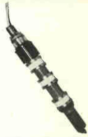
The Eimac 3K20,000LK is a three cavity, cascade, magnetically focused, power amplifier klystron intended primarily for UHF television broadcast service. A single 3K20,000LK operating as a television visual r-f amplifier will deliver 5.5 kW of peak synchronizing power output with a power gain of 20 to 25 decibels. The cavities of the Eimac UHF television klystron are completed by tuning boxes external to the tube.
