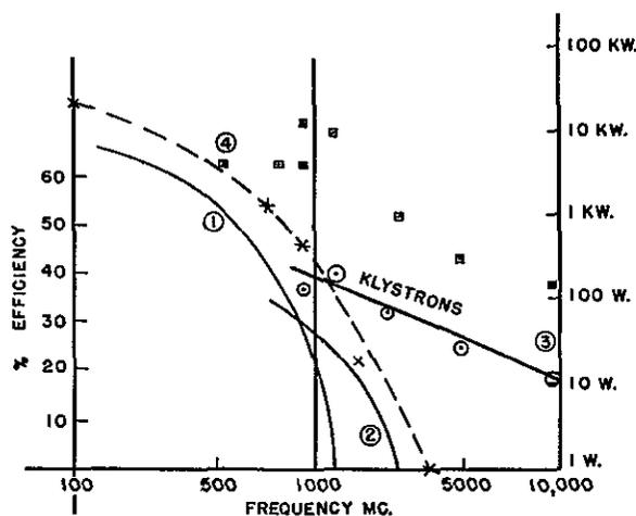
Fig. 2—Curve (1): Efficiency versus frequency for typical uhf tetrode—4X150G. (Plate dissipation 150 watts.)
