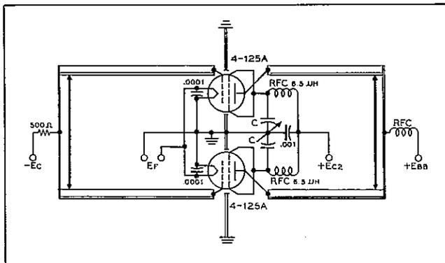
Screen-tuning neutralization circuit for use above 100 Mc.
