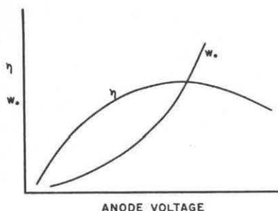
Fig. 5—Power output and efficiency versus anode voltage.
