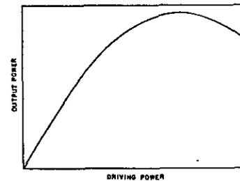
Fig. 3—Output power versus driving power for klystron.
