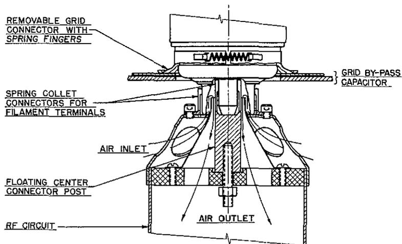
TYPICAL TUBE CONNECTORS AND STEM COOLING
