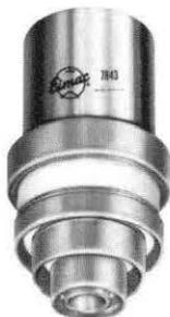
The 7843 is a small coaxial power tetrode designed for UHF power amplifier and oscillator service up to 1200 MHz. The coaxial construction makes this tube suitable for cavity circuits.
