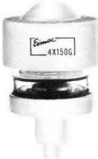
One of the forerunners in external-anode coaxial-based tetrodes, the 4X150G continues to deliver long life and high reliability in VHF and UHF applications. It is intended for use in CW service at frequencies up to 1200 MHz and is useful in pulse service at frequencies up to 1500 MHz.
