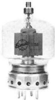
The 175A is a beam pentode which incorporates a unique vane-type suppressor grid. The suppressor grid terminates in the tube shell and is designed to operate at zero voltage. The base shell must be grounded to the chassis by means of suitable spring clips.
