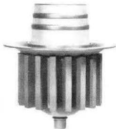
A vapor-cooled version of the popular 4CX5000A, the 4CV20.000A has a plate dissipation rating of 20 kilowatts. Two of these tubes in a push-pull, Class-AB<sub>1</sub> amplifier will produce 35 kilowatts output. A full complement of vapor cooling accessories is available for this and all other Eimac vapor-cooled tube types.
