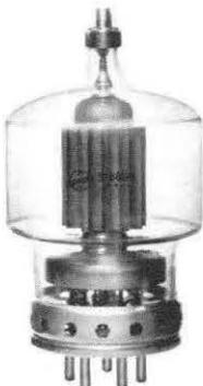
The 5-500A is a compact, ruggedly constructed radial-beam power pentode with a maximum plate dissipation rating of 500 watts. It is intended for use as an amplifier, oscillator or modulator. The high plate-current rating, low grid-plate capacitance and low driving power requirements permit maximum power capability to be combined with circuit simplicity and economic driver requirements.
