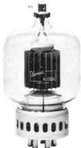
This high-power general-purpose tetrode is capable of dissipating 1000 watts from its radiation-cooled anode. Maximum ratings apply through the FM broadcast band but its low drive-power requirements make it an ideal choice for audio and low-frequency applications as well.
