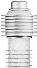
The 4CX125C is a horizontally-finned version of the 4CX300A and is intended for use where transverse air cooling is desired. It is also useful where anode power is dissipated by liquid immersion. Its electrical characteristics are identical to those of the 4CX300A with the exception of plate dissipation which is established at 125 watts with air cooling. It is ideally suited for applications where shock and/or vibration are experienced. The 4CX125F is an identical tube with a 26.5 volt heater.
