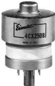
A 250-watt general purpose external-anode tetrode featuring ceramic-metal construction. This compact power tube can be used at maximum ratings at frequencies up to 500 MHz. It is recommended for use in equipments of new design. The 4CX250F is identical in all respects except for a heater rated at 26.5 volts.
