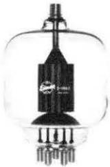
The Eimac 3-1000Z is a zero-bias triode intended for linear amplifier applications. This tube may be used as a class-B R-F amplifier in either the grid-driven or cathode-driven connection, or two 3-1000Z's may be used in push-pull as a grid-driven class-B audio amplifier or modulator. At a plate voltage of 3000 volts, 2KW PEP input can be run with a single 3-1000Z, providing a power gain of over 20 in the cathode-driven connection.
