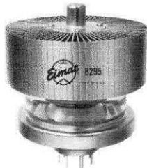
This tube is an air-cooled, glass and metal beam pentode capable of high power gain and excellent efficiency at relatively low plate voltages. The tube is especially suited for low-distortion Class AB<sub>1</sub> linear RF amplifier service.
