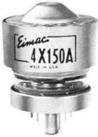
The veteran of external-anode tetrodes, and an Eimac original, continues to enjoy its deserved popularity. Recent tube improvements have made possible increases in maximum plate-voltage and plate-dissipation ratings. In Class-AB or Class-C service an input power of 500 watts is now allowed at frequencies up to 150 MHz. The 4X150D is a 26.5 volt heater version of the 4X150A.
