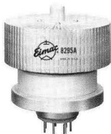
The 8295A is an air-cooled, ceramic-metal beam pentode capable of high power gain and excellent efficiency at relatively low plate voltages. The tube is especially suited for low-distortion Class AB<sub>1</sub> linear RF amplifier service.
