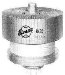
The 8432 is a ceramic-metal beam pentode featuring compact construction. The tube is especially suited for low-distortion Class AB<sub>1</sub> linear RF amplifier use where a single tube will deliver over 1500 watts of useful power output. The tube also provides outstanding performance in Class AB<sub>2</sub> and Class B service.
