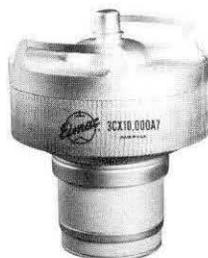
The Eimac 3CX10,000A7 is a ceramic-metal zero-bias triode intended for use in grounded-grid linear amplifiers delivering 20 kilowatts of useful output power. Because of its low intermodulation distortion characteristics the 3CX10,000A7 is particularly well suited for single-sideband amplifiers. Two tubes operating in a push-pull audio amplifier under class B zero-bias conditions will deliver up to 45 kilowatts of useful output power.
