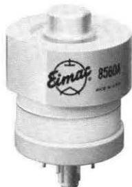
The 8560A is a conduction cooled, general purpose tetrode. This compact power tube can be used at maximum ratings at frequencies up to 500 MHz. It is recommended for use in equipments of new design.
