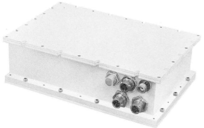
Model EM4567 is a complete transmitter, including a pre-regulated DC-DC converter. All circuits are solid state, except the rf power oscillator, which is a single stage rugged ceramic planar triode. RF is generated at the output frequency. The complete transmitter is packaged in less than 110 cubic inches, and weighs less than 8 pounds. Modulation is true FM. Major features of this transmitter include:
