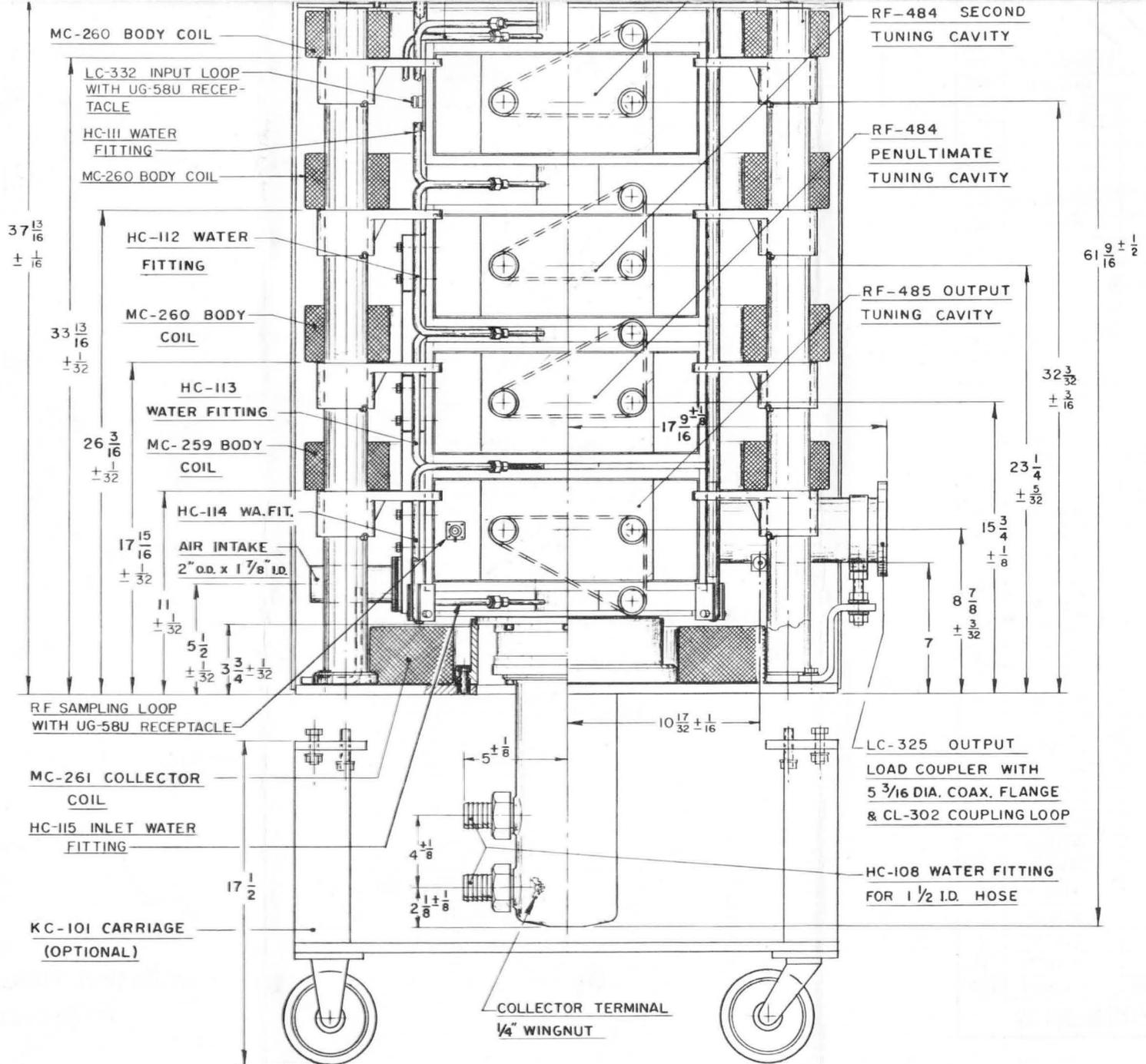
H-133 KLYSTRON AMPLIFIER CIRCUIT ASSEMBLY
