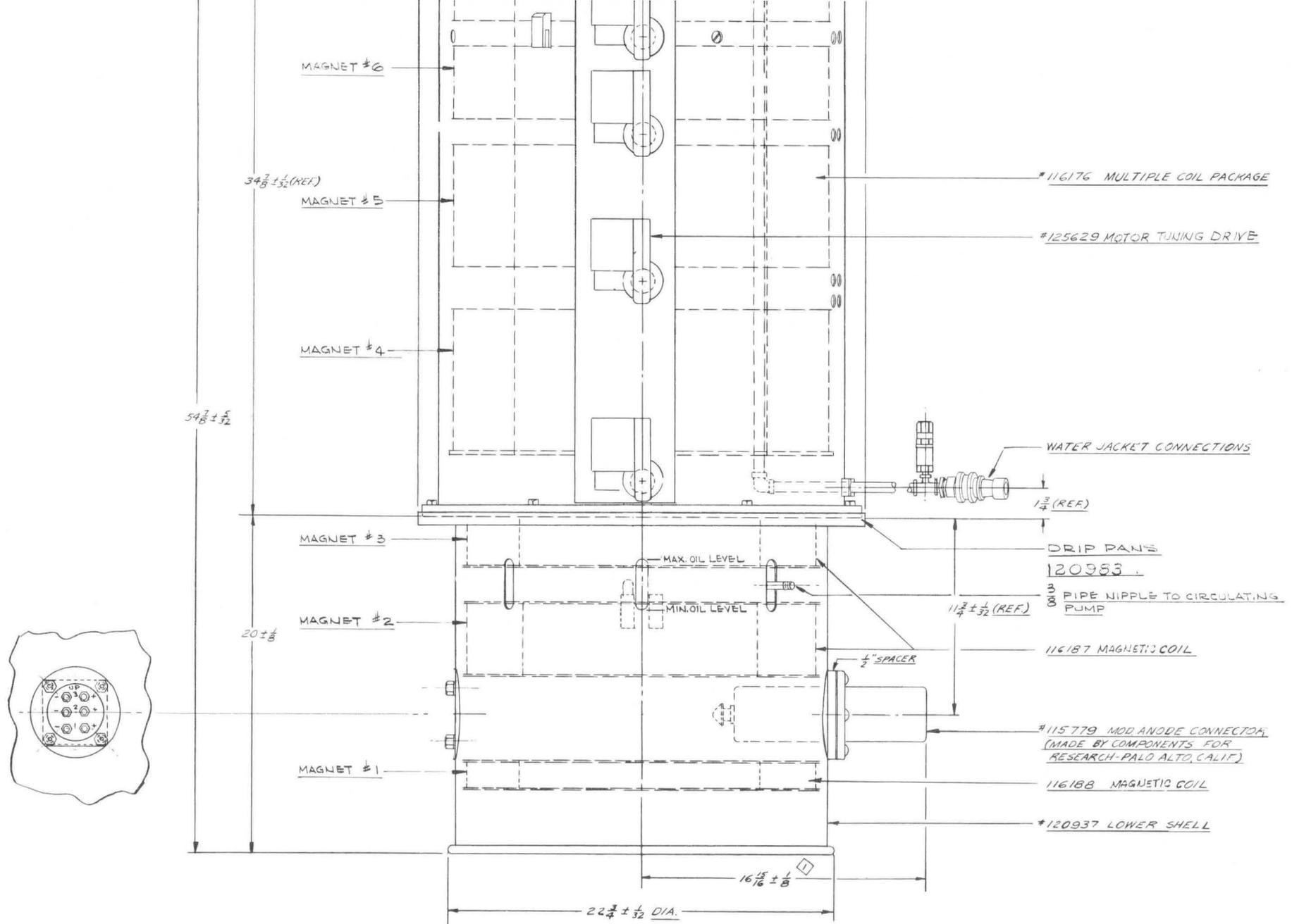
H-145 KLYSTRON AMPLIFIER CIRCUIT ASSEMBLY
