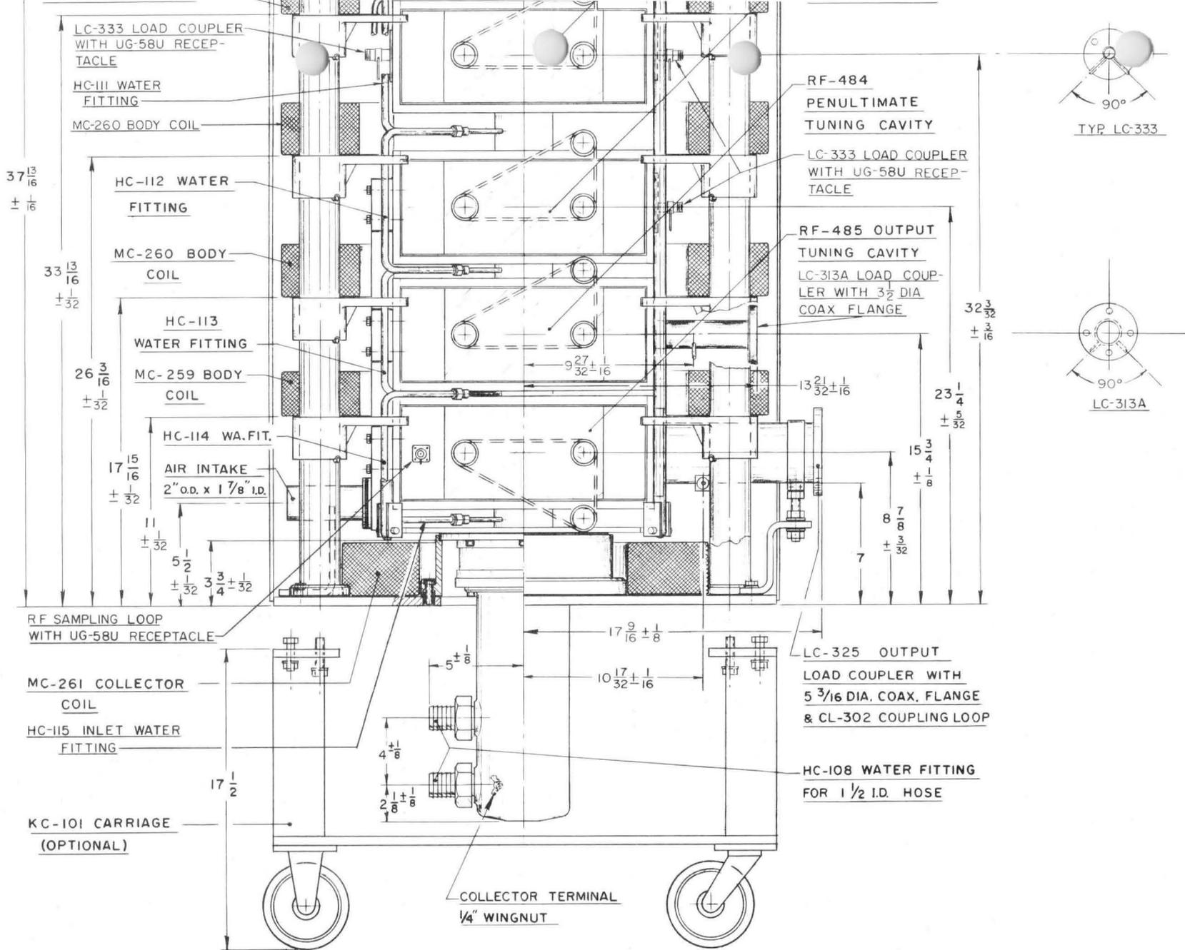
H-133 KLYSTRON AMPLIFIER CIRCUIT ASSEMBLY
