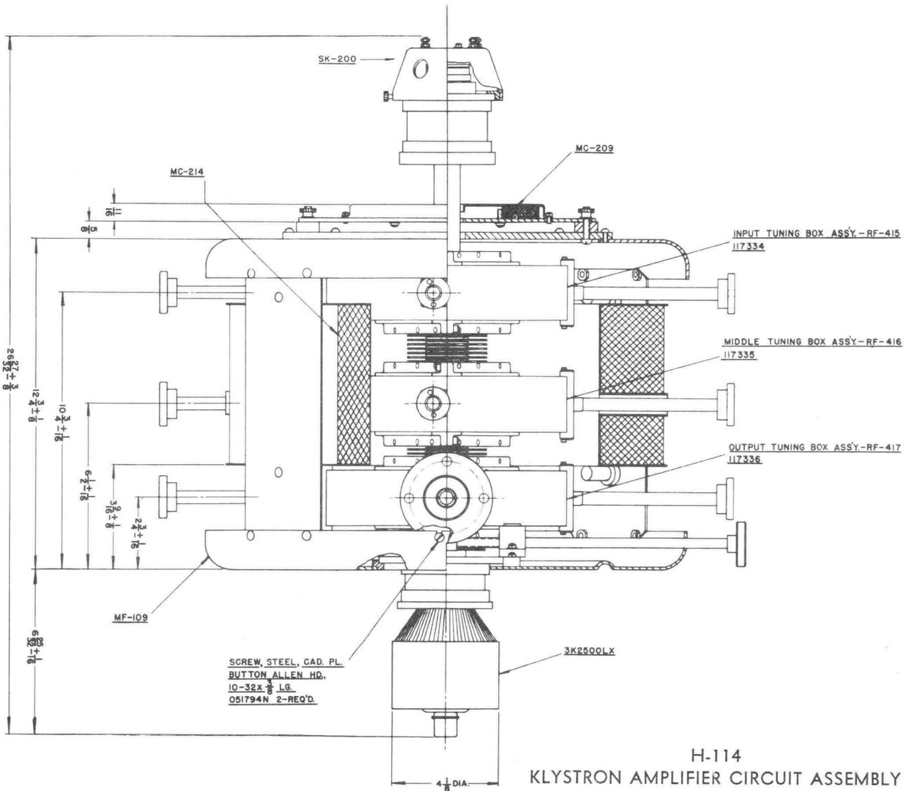
H-114 KLYSTRON AMPLIFIER CIRCUIT ASSEMBLY
