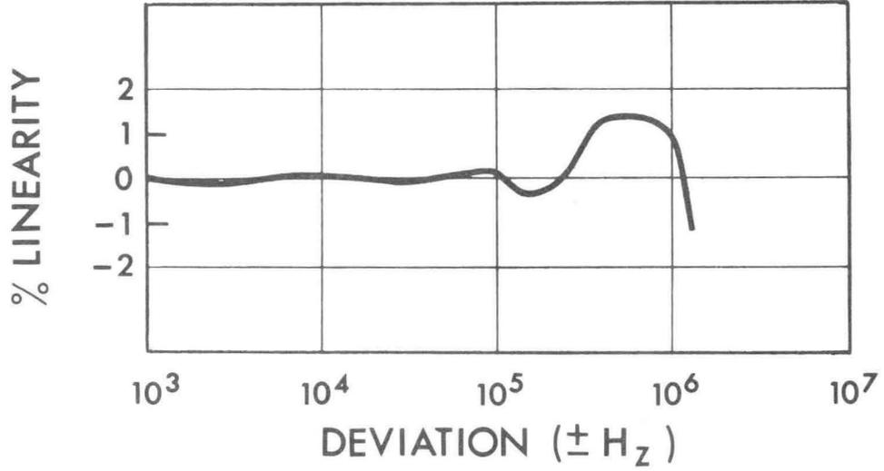
TYPICAL MEASURED MODULATION FREQUENCY RESPONSE
