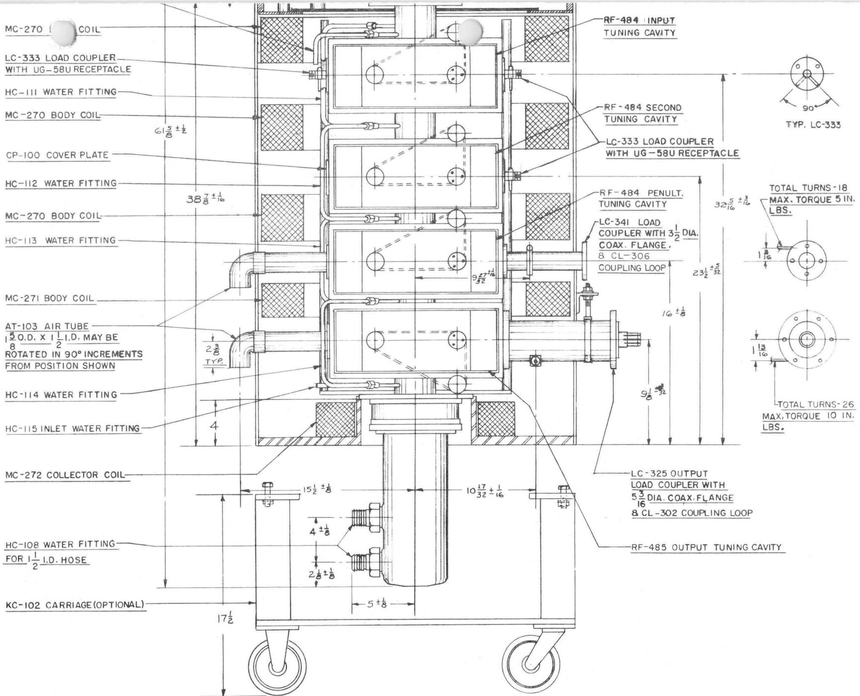
H-163 KLYSTRON AMPLIFIER CIRCUIT ASSEMBLY
