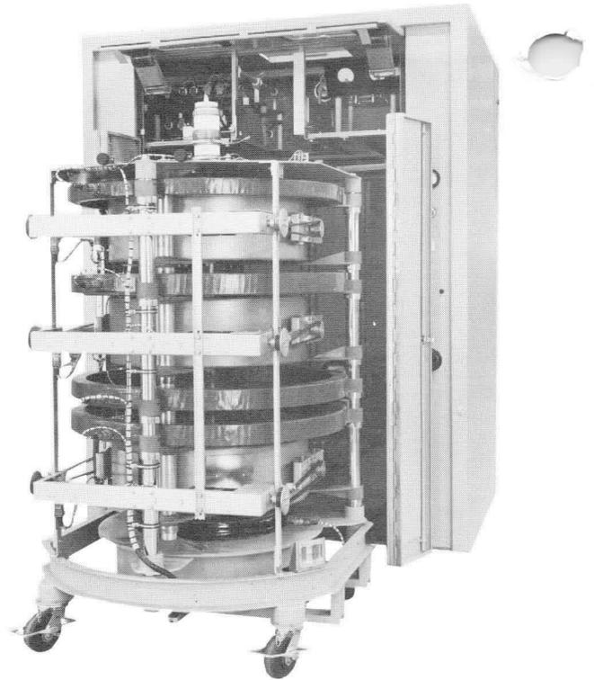
Collins Radio Company's 240D-2 amplifier, which uses an Eimac 10 kW power klystron. These power amplifiers are part of the ground command control network used for control of Project Mercury manned space capsules. Additional 240D-2 amplifiers will be used to control Project Gemini two-man space flights.
