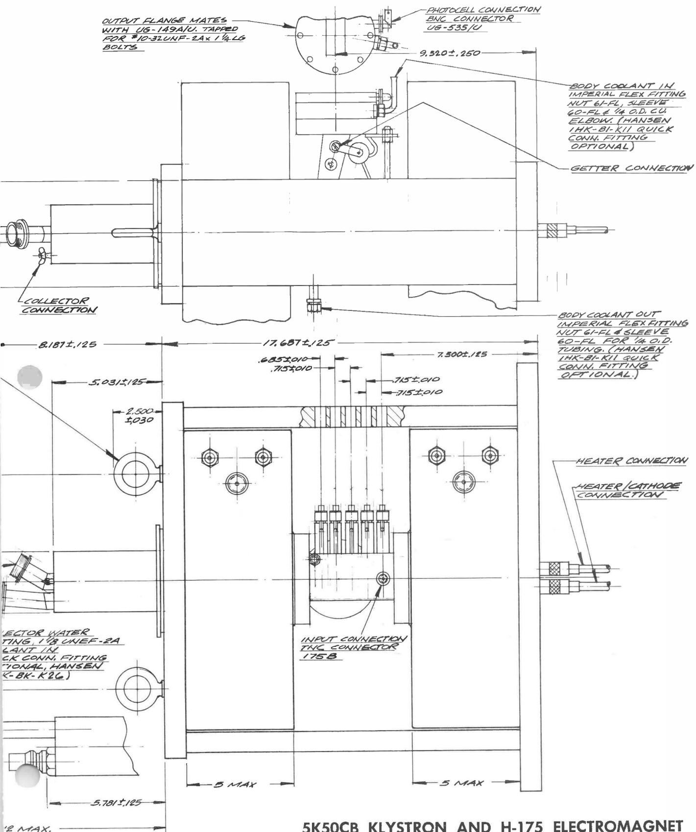
5K50CB KLYSTRON AND H-175 ELECTROMAGNET
