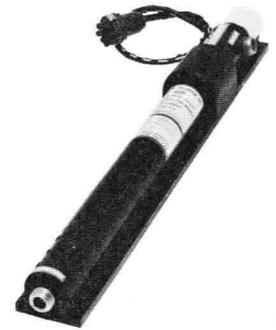
The EM-1050 features rugged ceramic and metal construction and focusing is provided by built-in periodic permanent magnets. These magnets are fully temperature compensated to allow operation from -55 to +85°C. No additional cooling is required at these temperatures due to the integral heat sink/mounting flange supplied with the tube.
