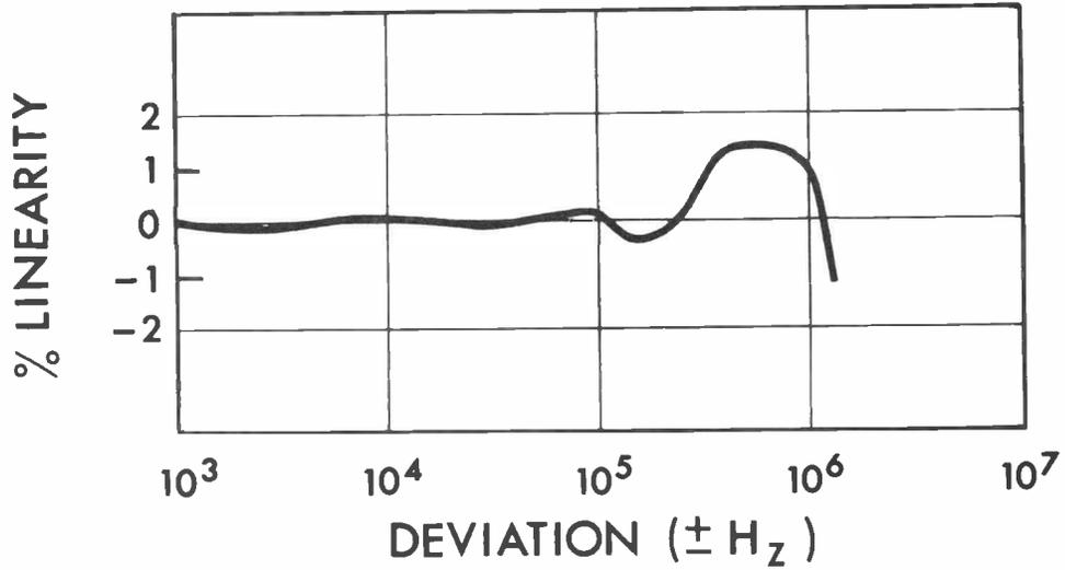
TYPICAL MEASURED MODULATION FREQUENCY RESPONSE
