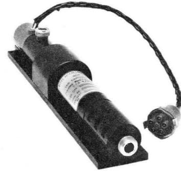
The EM-1016 features rugged ceramic and metal construction and focusing is provided by built-in periodic permanent magnets. These magnets are fully temperature compensated to allow operation from  $-55^{\circ}\text{C}$  to  $+85^{\circ}\text{C}$ . No additional cooling is required at these temperatures due to the integral heat sink/mounting flange supplied with the tube.
