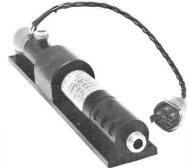
The integral heat sink/mounting flange allows operation to ambient temperatures of +85°C without additional cooling. Flexible leads provide electrical connections to the tube.
