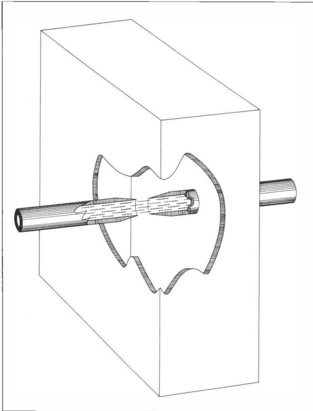
Figure 6—Simplified View of Resonant Cavity.
