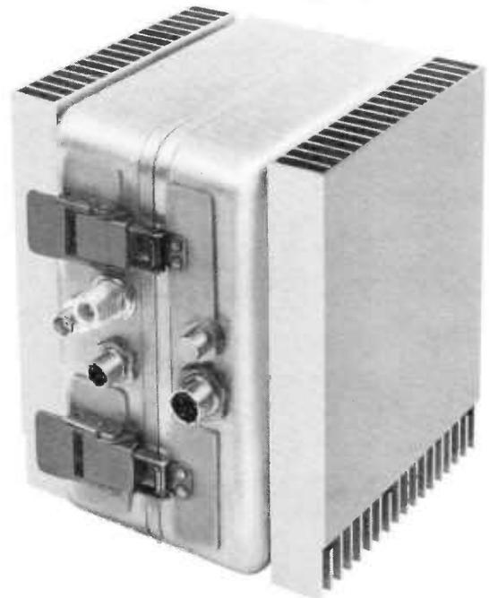
Model EM4575 is a complete transmitter, including a 400 CPS 115V power supply. All circuits are solid state, except the rf power oscillator, which is a single stage cavity using a rugged ceramic planar triode. RF is generated at the output frequency. The complete transmitter is packaged in less than 300 cubic inches, and weighs less than 11 pounds. Major features of this transmitter include:
