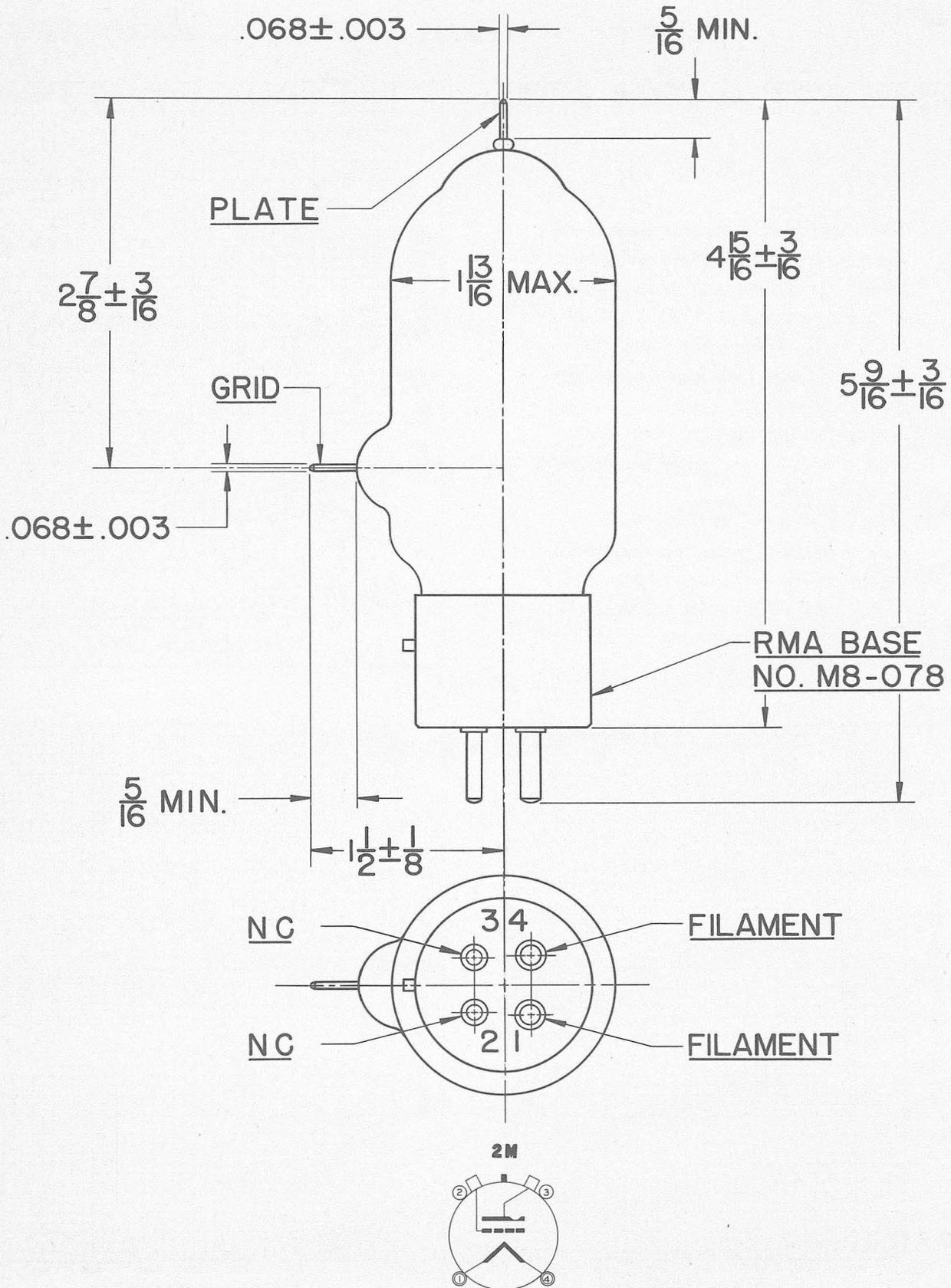
The Eimac 75TH is a medium-mu, high-vacuum transmitting triode intended for amplifier, oscillator and modulator service. It has a maximum plate dissipation rating of 75 watts. Cooling of the 75TH is accomplished by radiation from the plate, which operates at a visibly red temperature at maximum dissipation, and by air circulation around the envelope.
