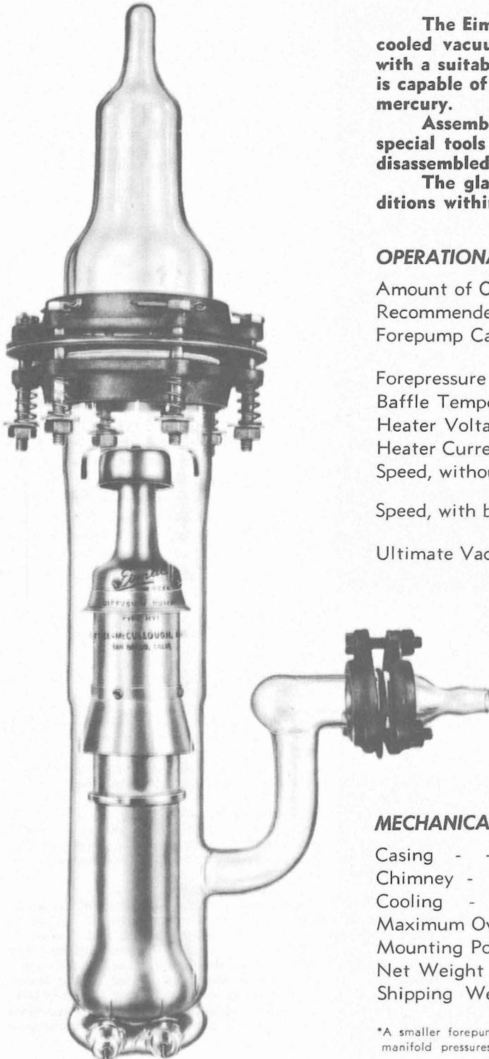
The Eimac HV-1 Diffusion Pump is a fast, triple-jet, air-cooled vacuum pump of the oil-diffusion type. When used with a suitable mechanical forepump and Eimac type A oil it is capable of reaching an ultimate vacuum of  $4 \times 10^{-7}$  mm of mercury.
