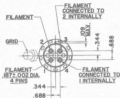
**NOTE:**—The grid terminal on the new 450TH and TL type tube is now .563" in diameter. To accommodate existing equipment which uses the 450TH or TL tubes with the old style .098" grid terminal, an adaptor pin is provided. This adaptor pin, if not needed, may be removed by unscrewing.
