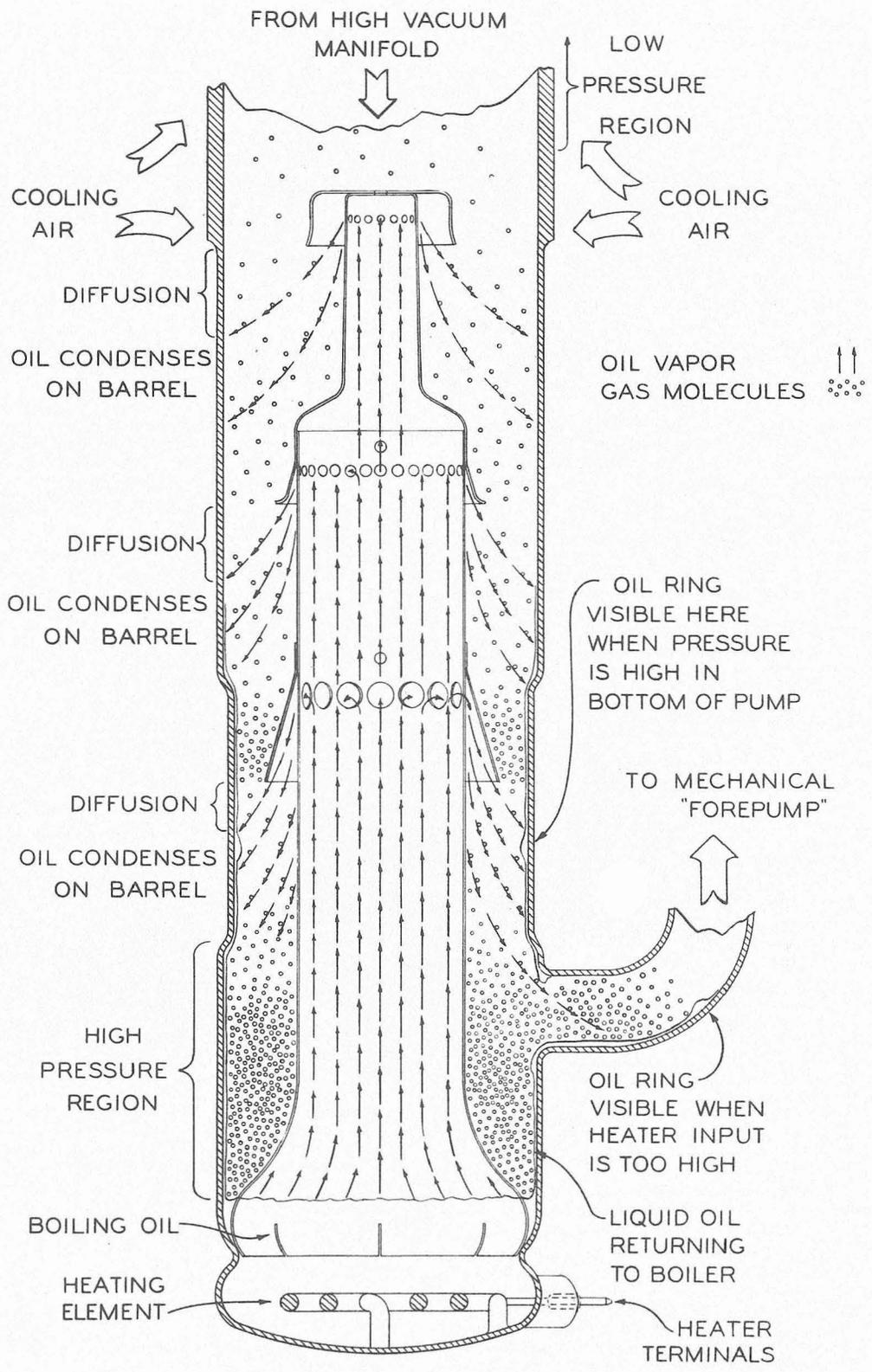
1. Pour 150 milliliters of Eimac Diffusion Pump Oil, Type A, into the pump barrel (917).
