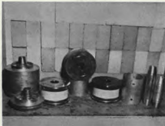
Fig. 7—Tube cavity parts and drift tube sections.
