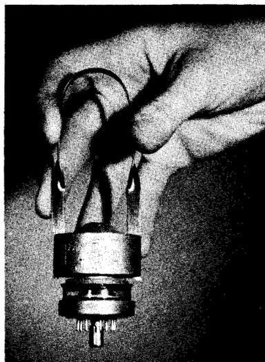
The Eimac 4X150 tube extractor may be used as pictured for inserting or extracting the 4X150A, 4X150D and 4X150G from normal or deep cavities. The prongs of the extractor are placed through the radiator of the tube and permit quick handling of tubes. The spring steel construction allows the tube to be gripped firmly without scoring the cavity walls. Only normal cavity wall clearance is required.
