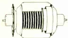
Eimac variable vacuum capacitors are intended principally for use as plate tank capacitors in radio frequency amplifiers and oscillators. The capacitance variation is linear with respect to shaft rotation and return to previously indexed settings is positive. The low-torque tuning mechanism is designed with adequate bearing surfaces to provide long life.
