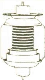
Eimac variable vacuum capacitors are intended principally for use as plate tank capacitors in radio frequency amplifiers and oscillators. The capacitance variation is linear with respect to shaft rotation and return to previously indexed settings is positive. The low-torque tuning mechanism is designed with adequate bearing surfaces to provide long life.
