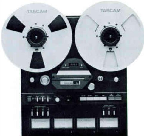
A 4-track 1/4" recorder/reproducer with 15-7 1/2 ips speeds, 10 1/2" reel capacity, full frequency response in sync mode, function and output select and punch in/out recording. The 34 also features ±12% pitch control, dump edit, cue control, FL tape counter and zero return.
