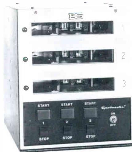
The Model 5300B is the most advanced multi-deck cartridge machine on the market. It is a top-of-the-line pro machine that features solid-state integrated circuit design, a direct drive hysteresis synchronous motor, air damped solenoid, 1/2" thick machined aluminum deck and long life NORTRONICS DURACORE heads. Features unique to this multi-deck design are plug in decks, computer ribbon cabling, rear panel LED service aids, and run lights adjacent to each deck.
