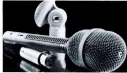
Literally born in a TV studio, the performance and reliability of the RE-15 have made it a workhorse directional microphone for broadcast. Two nulls at 150 degrees off axis provide greater average rejection over the microphone's rear hemisphere than a traditional single-null cardioid pattern, particularly useful on the boom and on-stage.
