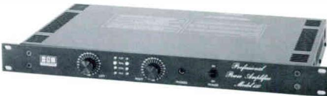
The BGW 150 is a rack mounted power amplifier rated at 50 watts per channel into 8 ohms, 150 watts into 8 ohms mono, with intermodulation distortion of less than .02%, a frequency response of -.25 dB 20 Hz to 20 kHz and is designed for any load impedance equal to or greater than 4 ohms.
