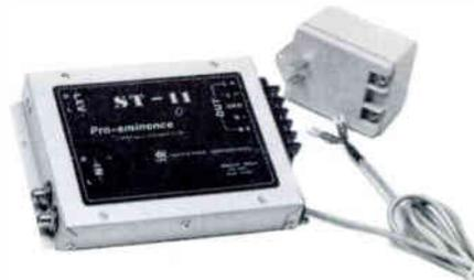
The ST-11 Pro-eminece phono pre-amp by Micro-Track is a super high performance unit. It is RFI resistant for use in AM, FM or TV. It is very compact and designed to match a 47K ohm magnetic stereo phono cartridge. Provision for a nominal 0 dBm output with headroom to a max. of +22 dBm. Distortion is .05 or less, THD and IM. The signal to noise ratio is -72 dB or better, also has a jumper selectable rumble filter internally.
