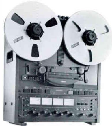
1/4" four channel, quarter track recorder/reproducer. DC-servo capstan with  $\pm 7\%$  vari-speed. 15-7 1/2 ips speed. +4 or -10 dB input/output level select. Real time tape counter with LED display. Zero return. Headphone output with channel select. Test oscillator (1 kHz or 10 kHz). Microprocessor controlled transport logic. Dynamic braking. Integral splicing block. External machine control interface connector for synchronizers.
