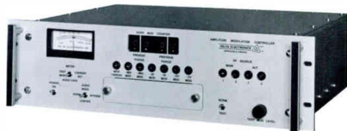
By continuously sampling the modulation levels at the AM transmitter output and comparing these levels with internal preset minimum and maximum modulation thresholds, the AMC-1 Amplitude Modulation Controller detects conditions of under or over modulation. The AMC-1 then uses a digital logic process to adjust the audio level of the transmitter. The audio control circuit is strictly linear so that no compression or asymmetry is added to the program.
