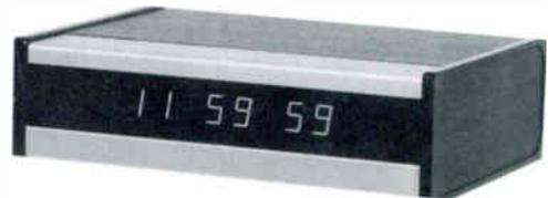
The ES-112E is a solid state 12 hour CMOS, six digit clock. It features three simple controls: fast advance, slow advance and hold which make setting to the precise second easy. The display is a bright orange, gas-discharge, seven segment, .55" high digital. An optional CMOS compatible BCD output can drive two .55" slaves or two 80 series slaves or one 90 series slave. Options prices are available upon request.
