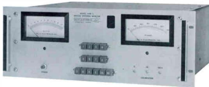
The AAM-1 Analog Antenna Monitor is designed specifically for measuring the parameters of AM broadcast frequency directional antenna systems. The monitor measures the relative current in each tower, the ratio of the current in each tower to that of a reference tower and the phase of the current in each tower relative to that of the reference tower. The AAM-1 can be equipped for up to eight input samples without external switching. Two reference towers can also be selected for DA-2 applications.
