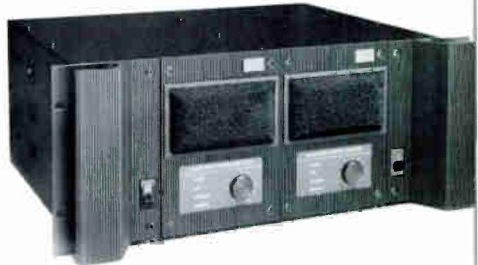
As opposed to the "fix-it-up-with-feedback" approach in common use today, UREI carefully departed from conventional design techniques. Each amplifier stage in the 6500 was engineered for optimum performance with no overall feedback. The 6500 features two channels on an independent, modular plug-in chassis with front panel access. The 6500 is rated at 275 watts into 8 ohms per channel output with .1 THD.
