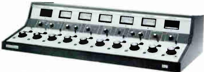
The LPB CITATION consoles come in only stereo and in only two configurations, 8 channel and 10 channel. The series features transformer balanced inputs and outputs, with three inputs per mixer, program, audition, mono mixdown, monitor, cue, headphone and tape outputs. The CITATION console features a signal to noise ratio of better than 74 dB below +18 dBm output with -50 dBm input 20 Hz to 20 kHz.
