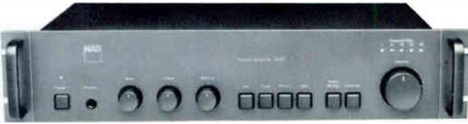
The NAD 3020B is a 20 watt state-of-the-art unit, offering totally uncompromised performance at a cost that buyers can afford. Among other things, the 3020B contains a unique "soft-clipping" circuit which allows it to play much louder than its rated power suggests. The 3020B has less than .02% of all types of distortion and a LED peak power indicator. Rack mount optional.
