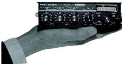
The Model FP-31 is a compact, portable microphone mixer specially designed for electronic news gathering (ENG) and electronic field production (EFP) use including film, video and remote broadcast applications. The FP-31 provides a wide, flat frequency response, low distortion, and up to +18 dBm output. The unit features extremely low internal noise and switchable low-cut filters for each input that effectively reject low-frequency handling and wind noise. 400 Hz slate tone, 1 kHz cue tone.
