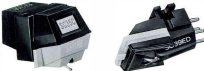
The SC35C is designed for use on the heaviest and most rugged tone arms which require a tracking force of 4 to 5 grams. The stylus assembly of the SC35C is rigid enough to withstand the punishment of continuous backcueing, yet compliant enough to offer excellent mid and high frequency reproduction. The SC35C is the spherical replacement stylus for this cartridge.
