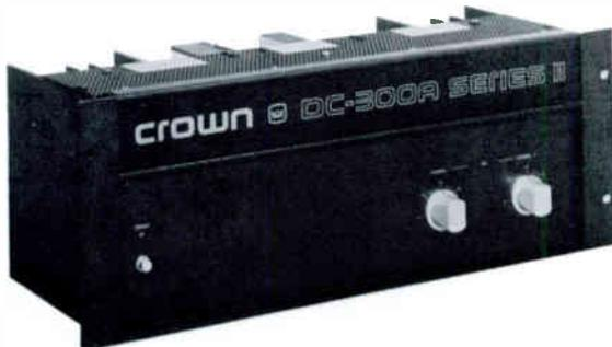
Since its introduction, the DC-300 and its modifications have been a standard of sonic accuracy, power and reliability. It is FTC rated at 250 watts per channel into 8 ohms; 500 watts into 8 ohms mono. The DC-300A Series II looks different from the front, with a scratch resistant, baked enamel front panel, new power switch, and relocated level controls.
