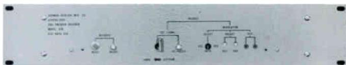
The CEB offers in a single rack mounting chassis, everything necessary for the two-frequency EBS system required by the commission except a receiver that can be tuned to the station monitored.
