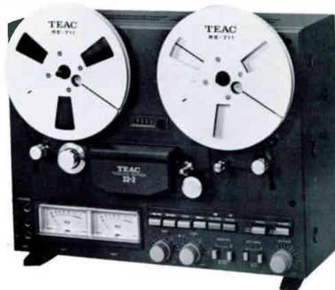
The basic half-track recorder/reproducer with independent record mode selector and 1 tape/source monitor for each channel. Independent mic/line mixing and output level control for each channel. Remote pause function for record and play. 7 1/2-15 ips speeds.
