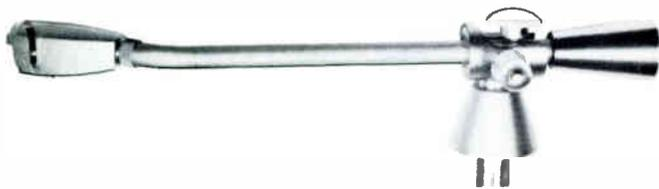
This attractive tone arm is constructed of tubular aluminum with a die-cast cartridge shell, that accepts all standard stereo or mono cartridges. It has a vertical height adjustment and friction-free chrome steel ball vertical movement. It tracks at 1 gram or less and includes a counterweight. Connects with standard plugs.
