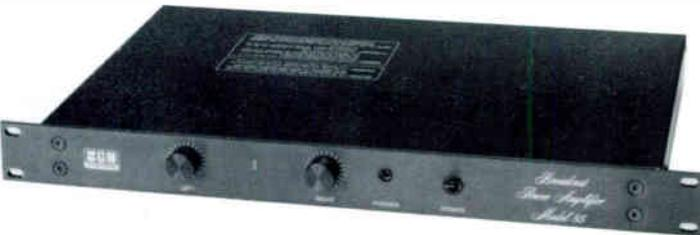
The BGW 85 is a rack-mounted power amplifier rated at 35 watts per channel at 8 ohms, with 0.1% T.H.D. 20 Hz to 20 kHz, 90 watts into 8 ohms mono, with 0.15% T.H.D. (The Model 85 features modular circuit assembly, toroidal mains transformer, packaged & cased transistors.
