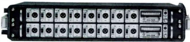
The "Press Corps 2" audio distribution package combines two DA-108 distribution amplifiers in a rugged carrying case. The two DA's may be bridged from a single input line using the cable supplied, or may be operated independently as separate 1 x 8 units. The carrying case has a detachable front and back cover to completely protect the distribution system during transportation. Transformer isolation on all inputs and outputs protects against AC ground loop current and RFI.
