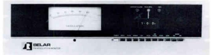
The FMM-2 sets new standards in accurate FM monitoring. It's the first to incorporate a sample hold peak modulation meter circuit independent of modulation polarity to allow the meter to respond to program peaks of the shortest duration. The heart of the FMM-2 is an ultra-linear digital discriminator which provides a distortionless baseband signal for accurate monitoring as well as precise stereophonic and SCA decoding.
