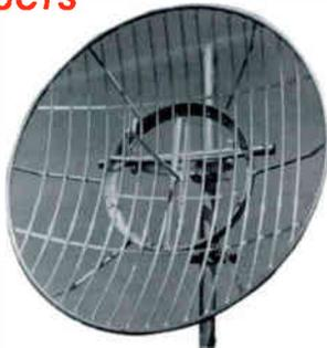
Mark Products offers a variety of sizes of Heli-Arc welded aluminum Multi-element Grid Parabolas for point to point relay operation in the 400 to 2700 mHz frequency range. The patented grid of construction is lightweight, yet extremely strong. One of the outstanding advantages of the grid antenna is that it has wind loading characteristics of only 25 to 40% of comparable size solid parabolas.
