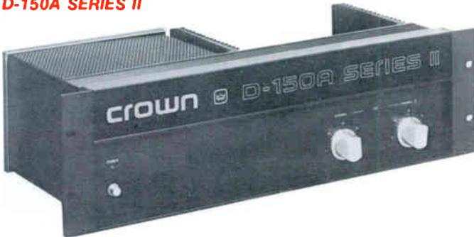
Retaining the D-150A tradition for sonic accuracy and reliability, the CROWN D-150A Series II is rated at 80 watts per channel into 8 ohms, 250 watts into 8 ohms mono. The frequency response is  $\pm 0.1$  dB DC to 20 kHz at one watt into 8 ohms;  $\pm 1$  dB DC to 100 kHz., less than .001% harmonic distortion, less than .01 I.M. distortion and 6 volts per microsecond slew rate.
