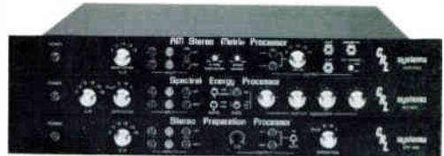
This four band system will outperform any other multi-band compressor. It provides maximum density to increase coverage and pre-emphasis for improved fidelity. The AM-4 stereo package contains the SPP800 PREPARATION PROCESSOR, a two band AGC unit that is gated to prevent noise pull-up, one SEP800 STEREO SPECTRAL ENERGY PROCESSOR, four band compressor/expanders with gating in each band, and an SMP900 AM STEREO MATRIX PROCESSOR, a state-of-the-art limiter which processes L+R and L-R separately.
