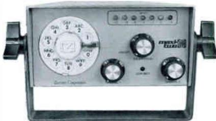
If a two channel mic/tape mixer will perform all the functions you need for remote broadcasting then the MAXI-TWO will fill the need. With two mic inputs or one plus a tape input for cassette, LED VU indication, battery or AC operation, and a telephone dial the MAXI-TWO is the maximum two channel mixer for your remote broadcasting program.
