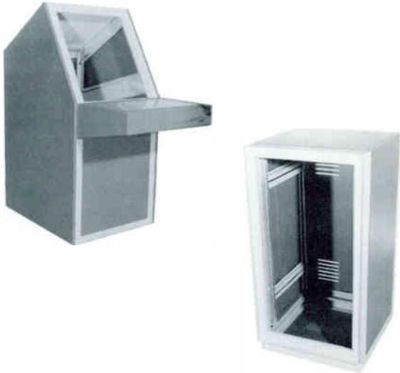
The DR series of H.O.M.E. 19" modular racks includes several features including sturdy welded construction of 16 gauge CRS, optional side panels that are removable for multiple bolt-together assemblies, adjustable 11 gauge angles tapped for 10-32 screws on standard EIA spacing that makes panel mounting easy. A cable opening is provided in the bottom panel. A rear door with lock and handle is provided. You can choose from 20 standard baked enamel colors. Depths to 24" available.
