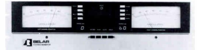
Working in conjunction with the FMM-2, the FMS-2 offers two independent peak modulation meters for simultaneous monitoring of left and right channels or L + R and L - R. It also has two independent auto-ranging voltmeters with LED displays for simplified automatic measurements of channel separation, crosstalk, sub-carrier suppression and noise.
