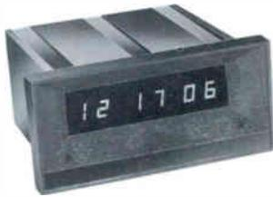
The ES-172 is a console mount clock/timer in compact enclosure, with bright easy to read six digit .4" red LED's. The controls consist of three settings: Fast Advance, Slow Advance, and Hold. The unit has access to control inputs on rear mounted connector and is entirely enclosed in a high impact black plastic case. Option prices are available upon request.
