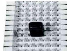
Where specific attenuation is needed the Allied "O" pad can provide a choice of 3, 6, 10, 17, or 23 dB attenuation.
