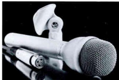
The RE-50 was designed expressly for hand-held ENG. It has the same tailored frequency response and high output level as the famous 635A. The RE-50 rubber shock mount "mike-within-a-mike" design achieves a degree of shock isolation never before known in the industry. The construction is also highly resistant to damage from mechanical shock.
