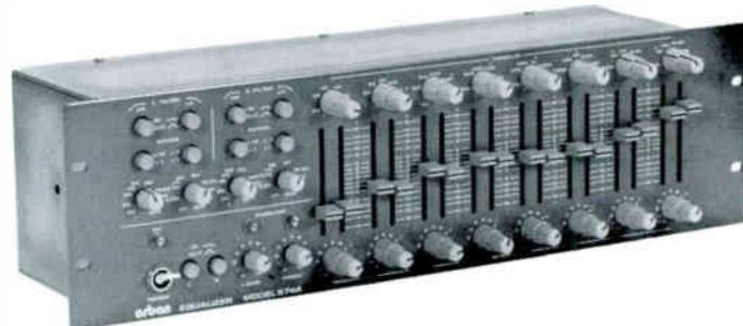
The ORBAN mono Model 672A and stereo Model 674A are cost effective, professional, quasi-parametric equalizers with the convenience of graphic type EQ controls. Wide range high and low pass filters with 12 dB/octave Butterworth slopes follow the graphic section for added versatility. Each feature has been thoughtfully
