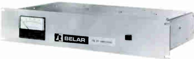
The RFA-1 FM RF Amplifier allows for remote monitoring of the transmitter in conjunction with Main and SCA FM modulation monitoring equipment. It offers a RF input sensitivity of 100 microvolt for full output, 50 to 75 ohms of input impedance and operates from 88 to 108 MHz.
