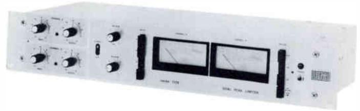
The UREI 1178 dual peak limiter is a two channel version of the 1176LN. The 1178 was designed for those applications where two channels of program material are processed and the balance of these audio channels must be maintained. The two limiters in the 1178 are perfectly matched to assure the high degree of tracking necessary for critical stereo applications. Limiting is accomplished by utilizing FET's as voltage variable resistors.
