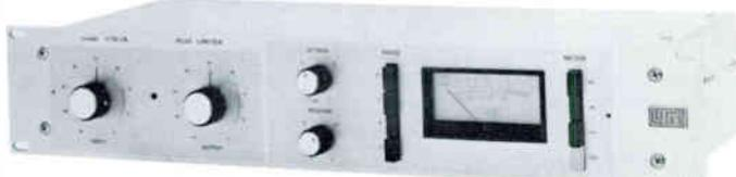
The UREI 1176LN single channel limiter features FET gain reduction ahead of the first stage. No tricky balancing required ever, there's no distortion adding active element in the gain reduction circuit, pushbutton selection of four different compression ratios and ultra fast attack time independent of peak duration or frequency and it's fully adjustable from the front panel.
