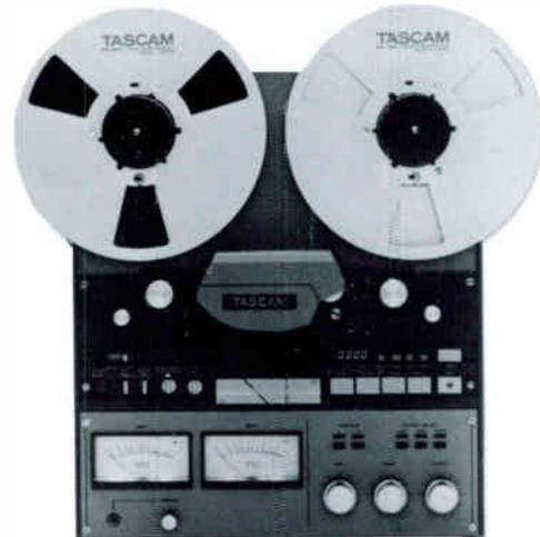
A 2-track 1/4" 2 channel half track mastering and broadcasting recorder/reproducer with 10 1/2" reel capacity, sync capability, full servo, SMPTE interlock capability through accessory connector and punch in/out recording. The 42 also features NAB or IEC equalization, dump edit, search to zero and search to cue, 7 1/2-15 ips speeds and +4/-10 input/output.
