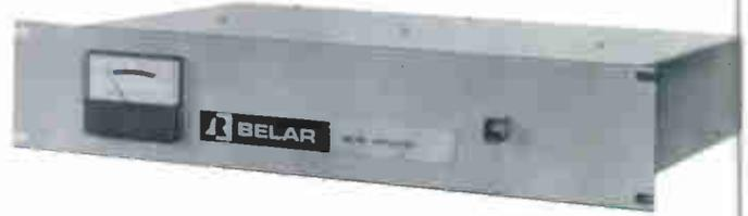
The RFA-2 AM RF Amplifier offers a selective, high gain, all silicon solid-state unit with AGC and makes it possible to monitor off-the-air AM signals accurately and conveniently without the problems associated with changes in transmitter power level, antenna patterns and signal fading. The RFA-2 when used in conjunction with AMM-2A, AMM-3 or AMM-4 allows monitoring of modulation characteristics at a remote point.
