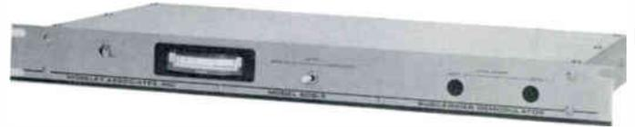
A Subcarrier Demodulator with automatic muting and front panel peak deviation meter, including a self contained power supply. Available for operation at a specific frequency in the 26 kHz to 186 kHz spectrum.
