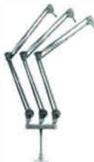
This unit was designed for those "around the table" conference and/or group interviews where multiple mics are required. The base — which rises approximately 9 inches, must be bolted to a supporting surface and contains 3 M2MD-U mic arms with standard springs. Each arm rotates 360° allowing various extension configurations.
