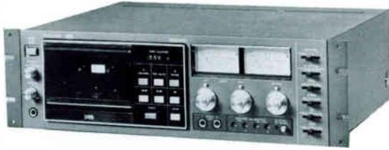
The 122B is a world standard cassette deck in broadcast studios. It has the same superb audio quality, reliability and features of the 122 except the 122B offers balanced XLR input and output connectors that operate +4 dBm nominal level/+18 dBm maximum. The 122 has unbalanced -14 dBV nominal level RCA input and -10 dBV output jacks.
