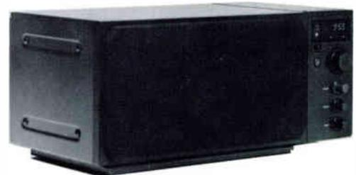
To achieve uncompromising fidelity with plenty of power, one 20-watt amplifier powers the 4 1/2 inch woofer, and a second 5-watt amp drives the efficient 1 3/4 inch dome tweeter. Since each amplifier functions best within its own portion of the frequency spectrum, the radio's 25-watts are equivalent to over 40 watts from a conventional amplifier. The Schotz variable bandwidth PLL detects or gives a revolutionary and dramatic effect on reception. Optional "ears" available for rack mounting.
