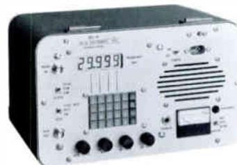
The RG-4 Receiver/Generator couples precision with reliable performance, providing an indispensable piece of test gear for broadcast engineers. An RF signal generator to excite the impedance bridge and a sensitive receiver for external null detection are housed in a single rugged case. With an OIB-1 or OIB-3, the RG-4 forms a portable impedance measuring system. Operates from 100 kHz to 29.999 MHz in 1 kHz increments. Runs off batteries, 115/230 VAC 50/60 Hz with 35 watts input power.
