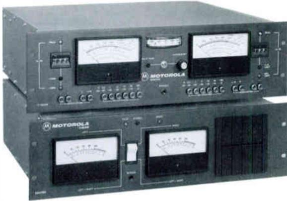
In the MOTOROLA C-QUAM AM STEREO SYSTEM, as in present AM broadcast standards, the angle modulated carrier is amplitude modulated with the sum of the audio information present in the program source. Thus to a monophonic receiver, the signal is no different from the signals being received under the present standards. This sum signal is comprised of two signals, left (L) and right (R).
