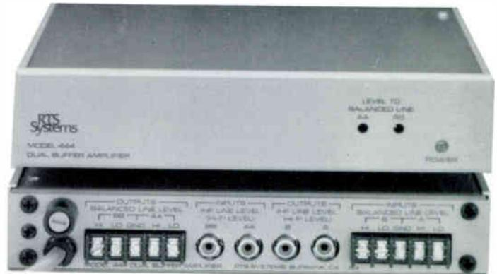
The Model 444 is a dual, two channel buffer amplifier designed to interface professional systems with semi-pro and high fidelity equipment. Although components designed for home use offer desirable features for studio applications, interconnections between the two kinds of equipment are complicated by differences in levels, impedances and balanced and unbalanced modes of operation. The 444 corrects these problems while maintaining signal integrity.
