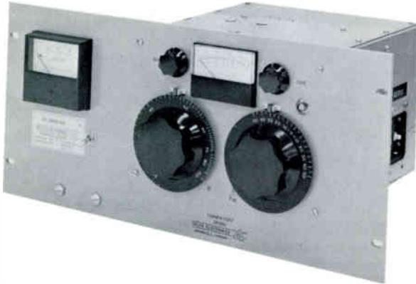
The Common Point Impedance Bridge is an invaluable device for directional array maintenance. The CPB-1 is designed for permanent installation in existing phasing equipment to provide an accurate indication of the common point impedance. The CPB-1 will handle common point powers of up to 5 kW with 100% modulation. The CPB-1A is designed for powers up to 50 kW.
