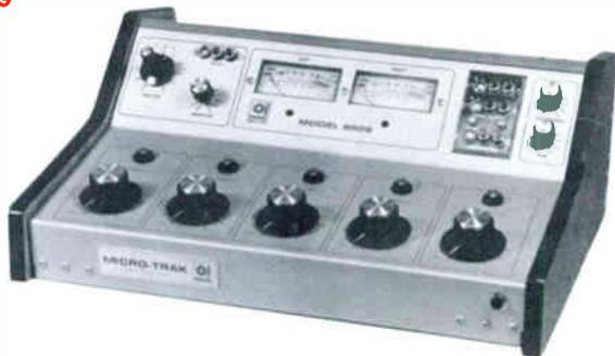
The Model 6509 audio console features five mixing channels, nine mixing inputs, outputs for stereo, mono, monitor, headsets and cue speaker, selectable muting, slotted screw terminal connections, illuminated VU meters. Crosstalk spec'd at -50 dB to -74 dB and distortion is 0.4% Re: +8 dBm output, 800 Hz, hi level input. Package size is 17 3/4 W x 12 3/4 D x 6 1/2 H and weighs 16 lbs.
