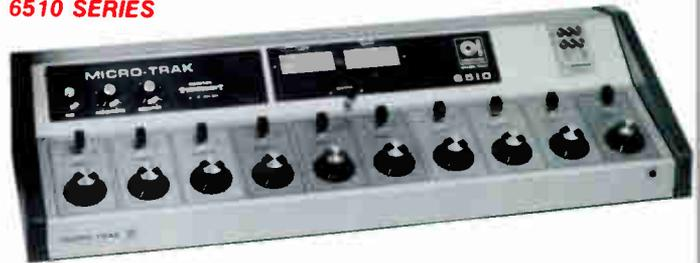
The Model 6510 features ten mixing channels, fourteen inputs, stereo or mono, selectable muting switch, relays for "on-the-air" lights, high quality VU meters, VCA attenuators, plug-in printed circuit cards and switches for easy maintenance, pushbutton input selector switches, barrier terminal strip input and output terminations, monitor output at line level, sealed main pots and compact design.
