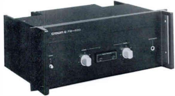
The CROWN PS-400 power amp is designed and built for the professional sound system. Into 8 ohms it will provide 180 watts per channel, into 8 ohms mono it will provide 520 watts. Check the all-pro features, terminal strips and phono jacks, ground separation strip, mono-stereo switch with binding posts conveniently positioned for quick conversion, detented controls, 4 second turn-on delay, IOC and signal presence indicators.
