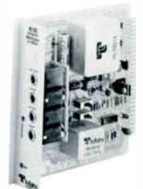
Each Tellabs 4018 module provides a 1 x 8 distribution amplifier with high impedance bridging or 600 ohms input and 600 ohms each port output. The 1012 housing permits mounting of up to eleven 4018 modules plus a 9021 fuse protection module. Combine this package with a rack-mounted 8013 power supply, and you have up to 11 x 88 distribution amplifier. All Tellabs equipment is connected by .075 wirewrap terminals. Cabinets must be wired by user.
