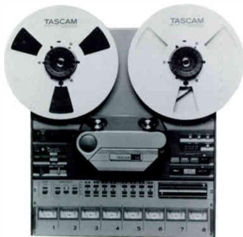
An 8-track 1/2" 8 channel production recorder/reproducer with -10 RCA input/output, 10 1/2" reel capacity, full frequency response in sync mode, full servo, SMPTE interlock capability through an accessory connector and punch in/out recording. The 58 also features pitch control (15% coarse/0.7% fine), manual tach wheel edit, dump edit, search to zero and search to cue and 15 ips speed.
