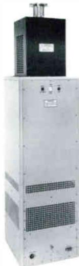
The first of a new series of dry, forced air cooled high power Load Resistors, model 8572 is a well-matched termination for 50 ohm rigid line systems to 25,000 watts for testing and alignment of transmitters. The RF power is dissipated in a large number of rugged parallel/series connected resistor elements, which not only provide an extensive total surface for heat transfer, but assure that the Load is not rendered inoperative due to the unlikely failure of one or two of the elements.
