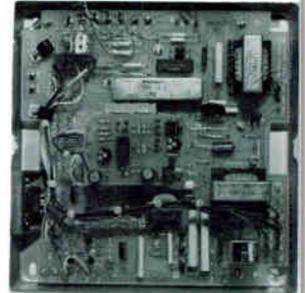
The DTD-5 is a dialtone/busy detector for use in those telephone systems which do not provide momentary open/battery reversal, the actions necessary to implement the ELGIN 20721 "Listen Line."
