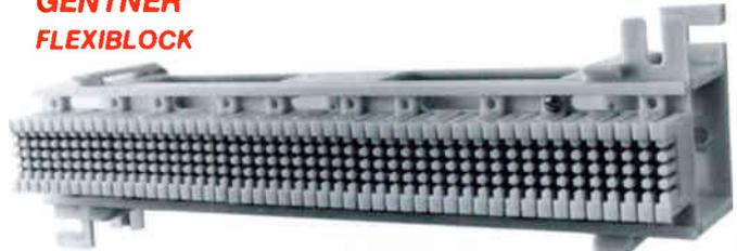
The Gentner Flexiblock is an insulation-displacement punch block system made specifically for stranded wire. Connections to Flexiblock are fast, easy and reliable. A high number of connections may be made in a small space (up to eight connections per circuit) and connections are virtually short-circuit proof. Standard size is 10"L x .56"H x 3.37"W with 50 terminals. (Variables available)
