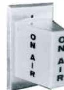
The Allied "MICRO SERIES" warning light is supplied with one 1820/28 volt lamp. The unit is designed for use with 24 volts for extended life. All models mount on standard single gang wall boxes or plaster rings. The wedge shaped translucent cover is available in red or white.
