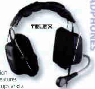
This hearing protection headset from Telex features sound-blocking earcups and a noise-canceling dynamic microphone. The polyurethane earcups house 150 ohm dynamic elements with 21 dB of noise reduction, and feature an easily adjustable headband. The 6 foot cord is coiled for tangle-free use, and the dynamic boom mic is flexible for easy adjustment. Cable is 6 ft.; connector type is A4F.
