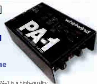
The Whirlwind PA-1 is a high-quality, portable stereo headphone amp. It accepts both balanced and unbalanced stereo line level signals through paralleled XLR and 1/4 TRS inputs. A mono/stereo switch allows selection of either stereo or mono operation. In mono mode, two separate inputs can be mixed in conjunction with the balance control. A pad switch attenuates the input -20 dB. It operates on two 9-volt batteries or AC power.
