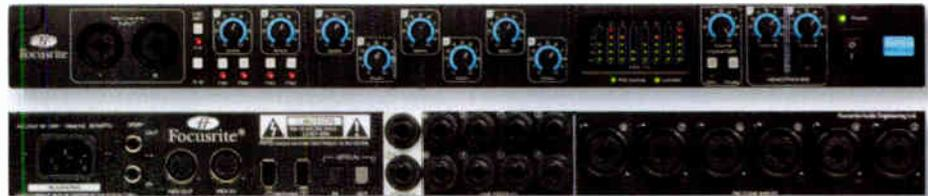
Two independent headphone buses are provided, each with their own level controls available on the front panel. Front panel controls include a main monitor dial with dim and mute switches, all of which fully integrate with customizable software to cover every possible monitoring need, providing a set of controls for any set-up from basic stereo to full 7.1 surround.
