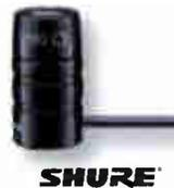
Shure Microflex WL183, WL184 and WL185 lavalier electret condenser mics designed for use with a Shure wireless bodypack transmitter (see page 128). Each mic has a 4 ft. cable terminated with a miniature 4-pin mini connector. The included tie clip can be rotated in 90 degree intervals for placement flexibility. Frequency response is 50 Hz-17 kHz, mic withstands SPL of 120 dB.
