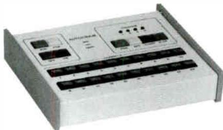
**Autogram's Live Assist Package** consists of one micro-processor board, one control panel and one interface board with cable.
