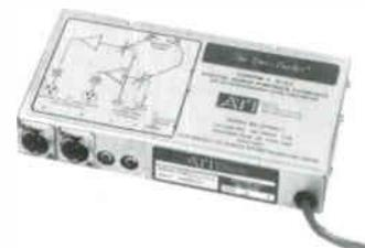
A uni-directional stereo interface for Playback Only applications. It is designed specifically to convert the unbalanced IHF outputs of Digital Compact Disc Players to transformer balanced and isolated 600 ohm line levels with no compromise or degradation of the superb performance available from the digital audio source. The DiscPatcher™ is equally at home on a newsroom desk to interconnect field ENG cassette recorders into broadcast systems for dubbing.
