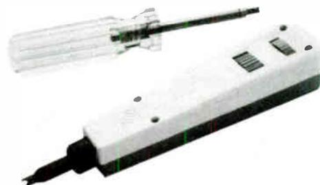
The insertion tools are used for insertion of wire into the QCP split cylinder modules. The impact tool applies the correct force to the wire by a spring loaded mechanism within the tool. Either of 2 impact forces can be applied, as selected by the LO-HI thumbwheel on the side of the tool. The LO position installs 24 or 26 AWG wire, the HI position installs 22 AWG wire. The impact tool includes 1 removable tip which comes stored in the tool's handle.
