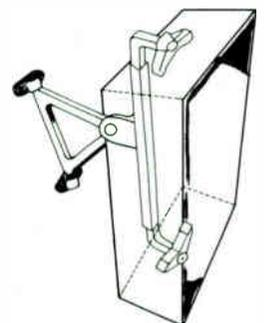
The Limpet Universal Baseplate can be mounted horizontally or vertically, and grips the cabinet from above, below or behind, with rubber covered clamps. Both clamps swivel, so that even equipment with rounded or tapering sides can be securely held.
