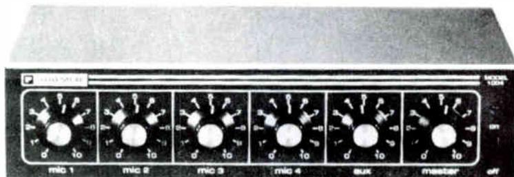
— Plus music mute, bridging inputs, 3-pin connectors, balanced LO-Z output, multiple connector choices and many other features to meet the requirements of the most demanding audio installation.
