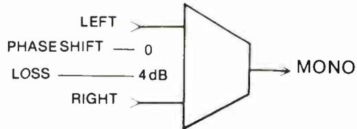
FREQUENCY RESPONSE: 10 Hz — 15 kHz  $\pm 1$  dB • IMPEDANCE: 600 ohm in & out
