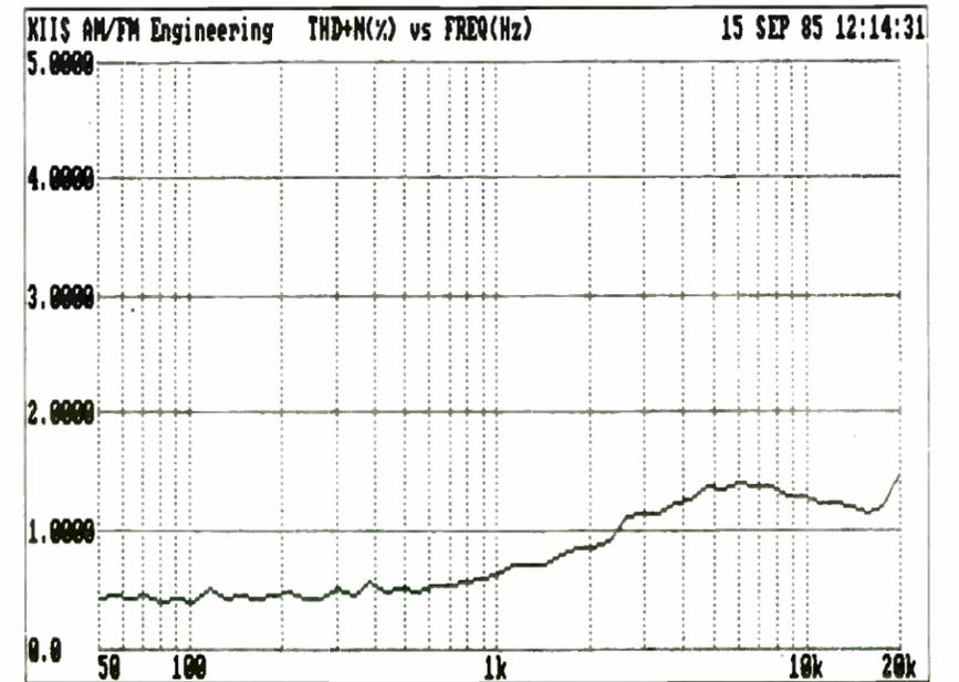
Figure 2. Total harmonic distortion plus noise from 50Hz to 20kHz. The vertical axis represents percent and the horizontal axis represents frequency.
