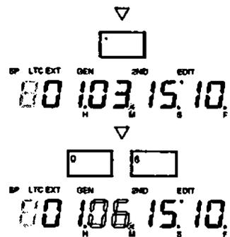
3. After correcting the time data, press the **STO** key, and selected **n** (using the numerical keypad), to store into cue memory "n".
