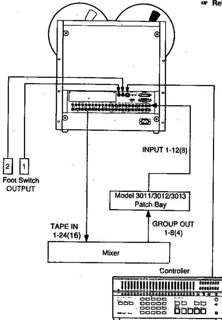
\* The Above illustration shows an example connection with G24S. Bracketed figures are when using G16S.
