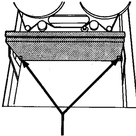
(b) Pull the controller forward and remove as shown in the following figure:
