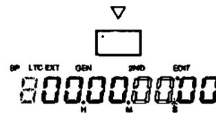
(c) If the [·] key is pressed while the (H) digit is blinking, it will return to the "all digit trim mode." With each press of the [·] key, it will continue to cycle through "all digit" → "two digit (F)" → "two digit (S)" → "two digit (M)" → "two digit (H)" → "all digit" → "two digit (F) .....
