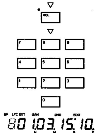
2. Press the [·] key to move the cursor to the digit (H/M/S/F) to be corrected (cursor will move to the left each time it is pressed). Then re-enter time data of that digit using the numerical keypad.
