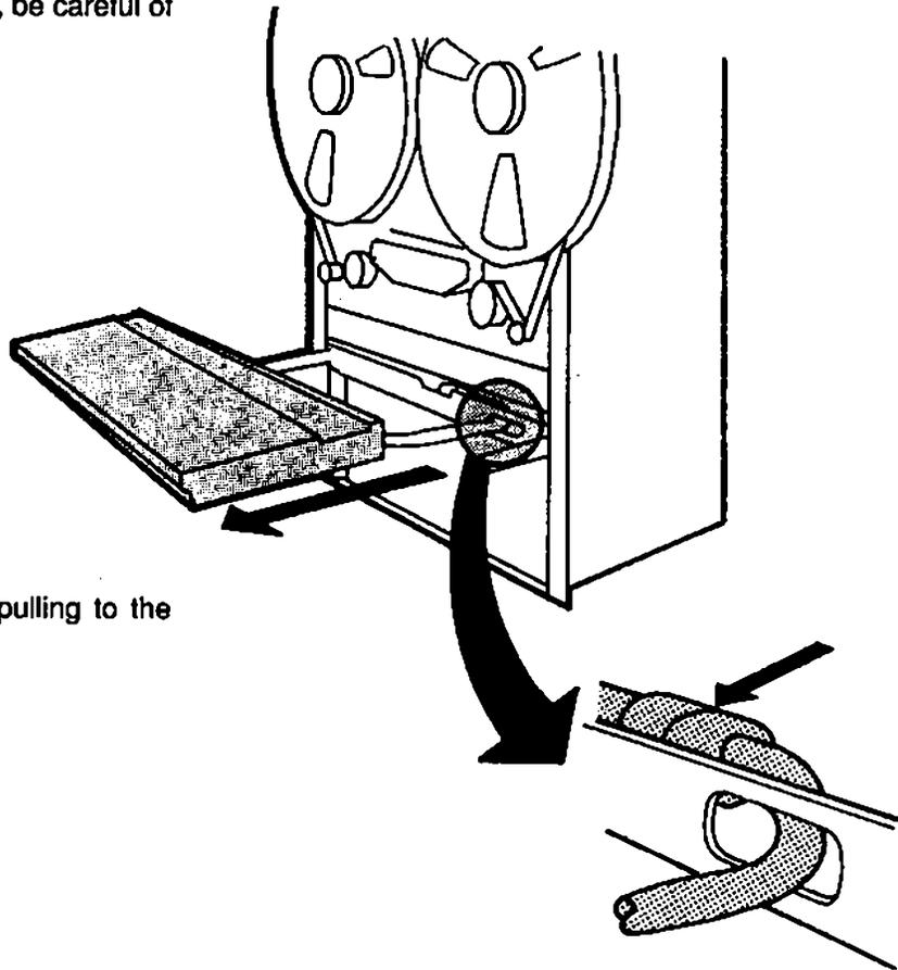
(c) The connector is unlocked by pulling to the right.
