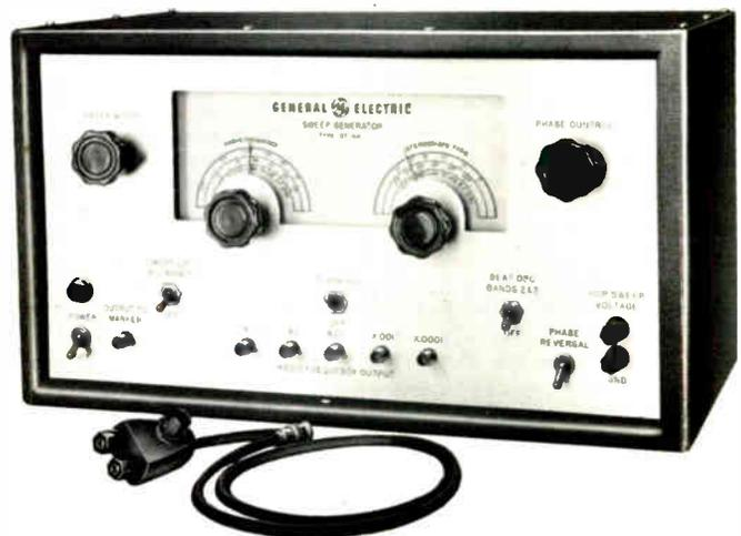
High output voltage is available over the entire range of the equipment, with higher output available in the high television channels where it is most needed for head-end development and testing. Beat output is used on the low bands and direct output on the high bands.
